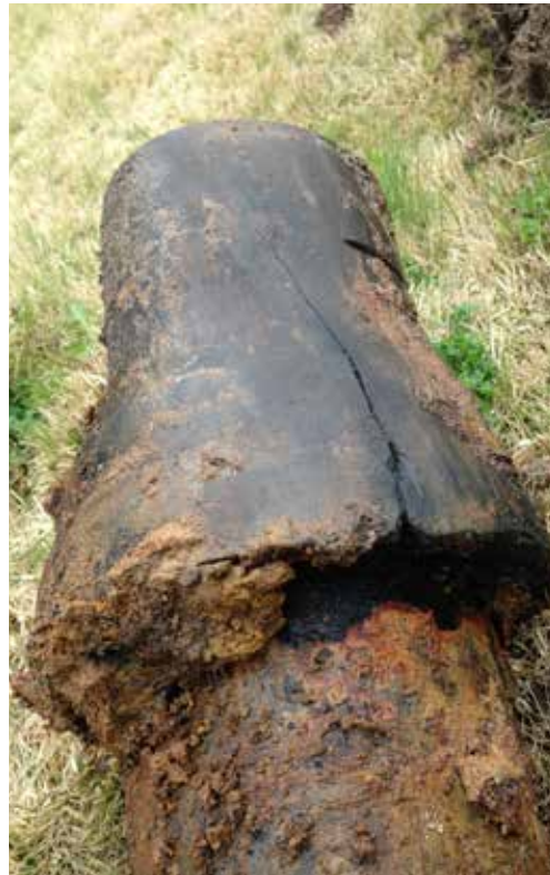
EchoShore-DX platform detected this leak several weeks earlier than by using conventional equipment.
