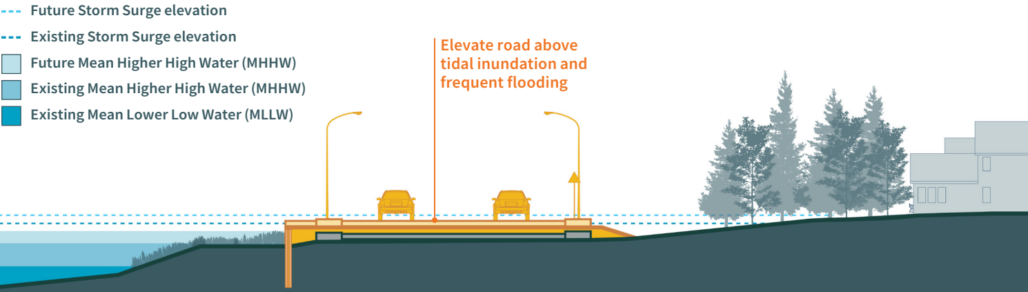
Section 08: Illustrative section of elevating a road above frequent flooding and tidal inundation. Drawing not to scale.
