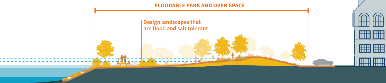
Section 14: Illustrative section of floodable waterfront open spaces. Drawing not to scale.
