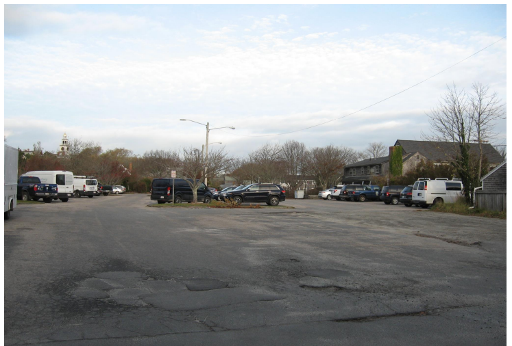
The introduction of permeable surfaces for large parking lots in the historic district’s flood zone should be considered in the future. The large expanses of asphalt in the lots on Salem Street (above) and Fayette and Washington Streets (below) contribute to the flooding in these areas.
