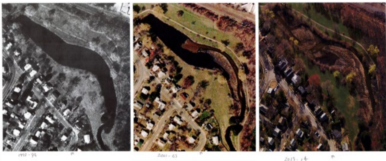
Figure 10. Sediment Accumulation at Davidson Park from Aerial Photographs from the Early 1990s (left panel), Early 2000s (middle panel), and 2013–2014 (right panel)
