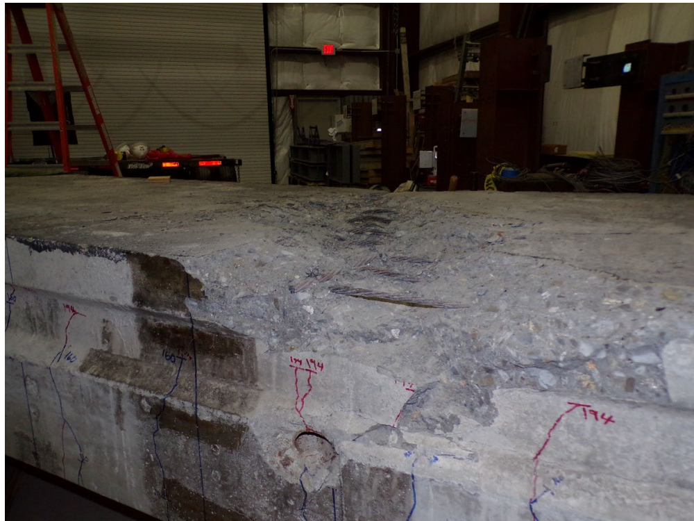
Figure 5.17: Concrete crushing after failure of Specimen R4
