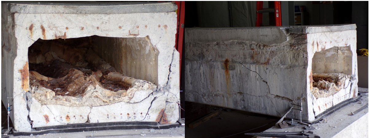
Figure 5.22: South end failure of Specimen E4
