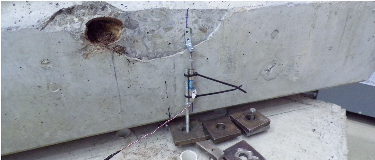
Figure 5.4: Typical attachment of potentiometer at supports
