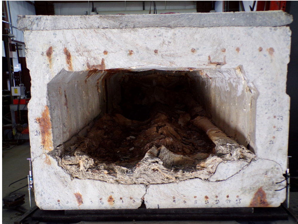
Figure 4.16: Effect of form void shifting in web thickness (Specimen E4)
