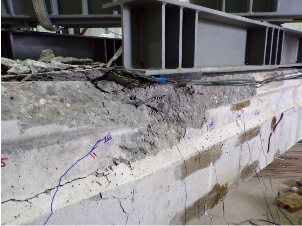
Figure 5.13: Concrete crushing at failure of Specimen R3
