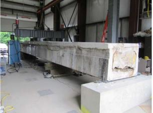
Task 7: Develop load rating procedures for precast, prestressed deteriorated beams for inclusion into the MassDOT bridge manual
