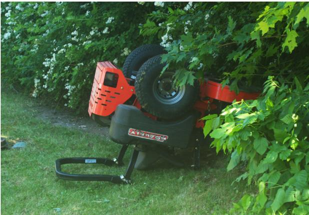
In June 2017, a 57-year-old equipment operator was killed while operating a zero-turn mower with the ROPS folded down. At the time of the incident, the equipment operator was working alone while mowing grass. As the operator turned the mower to the left, it struck a low-lying rock covered by vegetation. The mower overturned, pinning the operator against the ground. Eventually, a motorist passing by noticed the overturned mower, stopped, and placed a call for emergency medical services (EMS).
