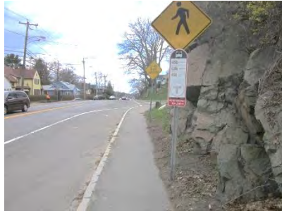
Image III.18: Sign position too low, should be on own post, without obscuring pedestrian crossing sign bus stop sign, inbound at Belleaire/opposite Buchanan.
