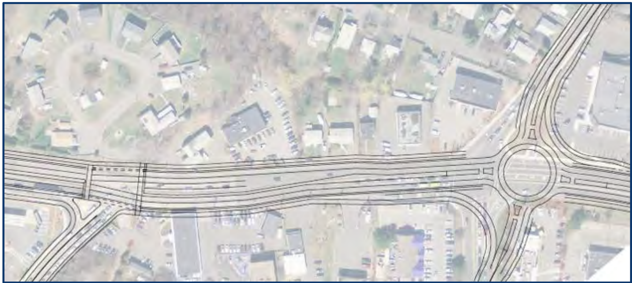
Figure V-42: Marlborough Road Roundabout Shifted Toward CVS with Northbound and Southbound Bypass Lanes and Dual Left Turn Lanes at Swampscott Road
