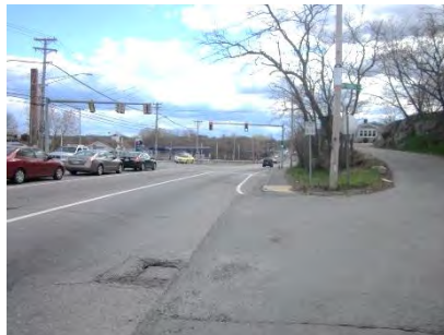
Image III.20: Bus stop sign faded & posted much too high for pedestrian visibility and set back too far from the curb, essentially on the side street, inbound at Thomas Circle.
