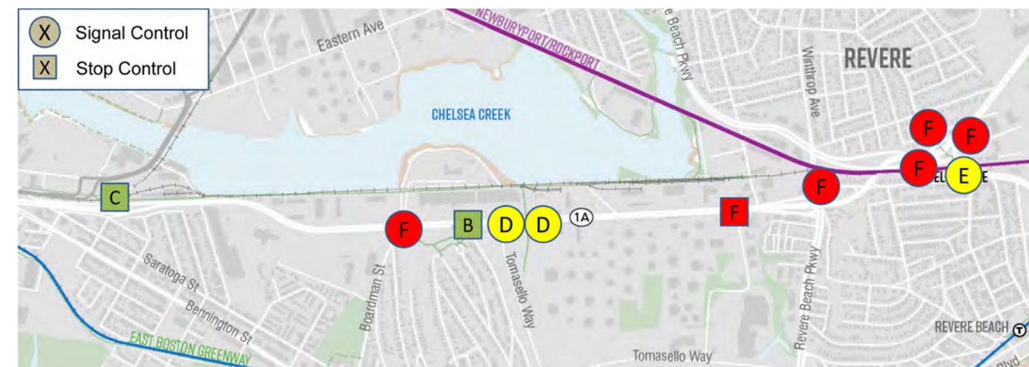
Figure 2-21. Auto Level of Service – Future 2040 with Suffolk Downs Mitigation – Evening Peak Hour
