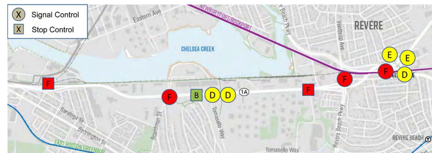
Figure 2-20. Auto Level of Service – Future 2040 with Suffolk Downs Mitigation – Morning Peak Hour
