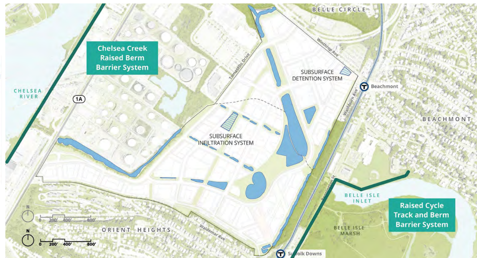
Figure 2-45. Unfunded Proposal for a Raised Berm Barrier System along the State-Owned Rail Corridor (HYM)
