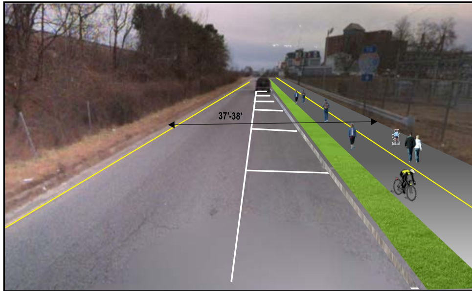
Figure 3.7: Intermediate Improvement – Davol Street West Shared-Use Path
