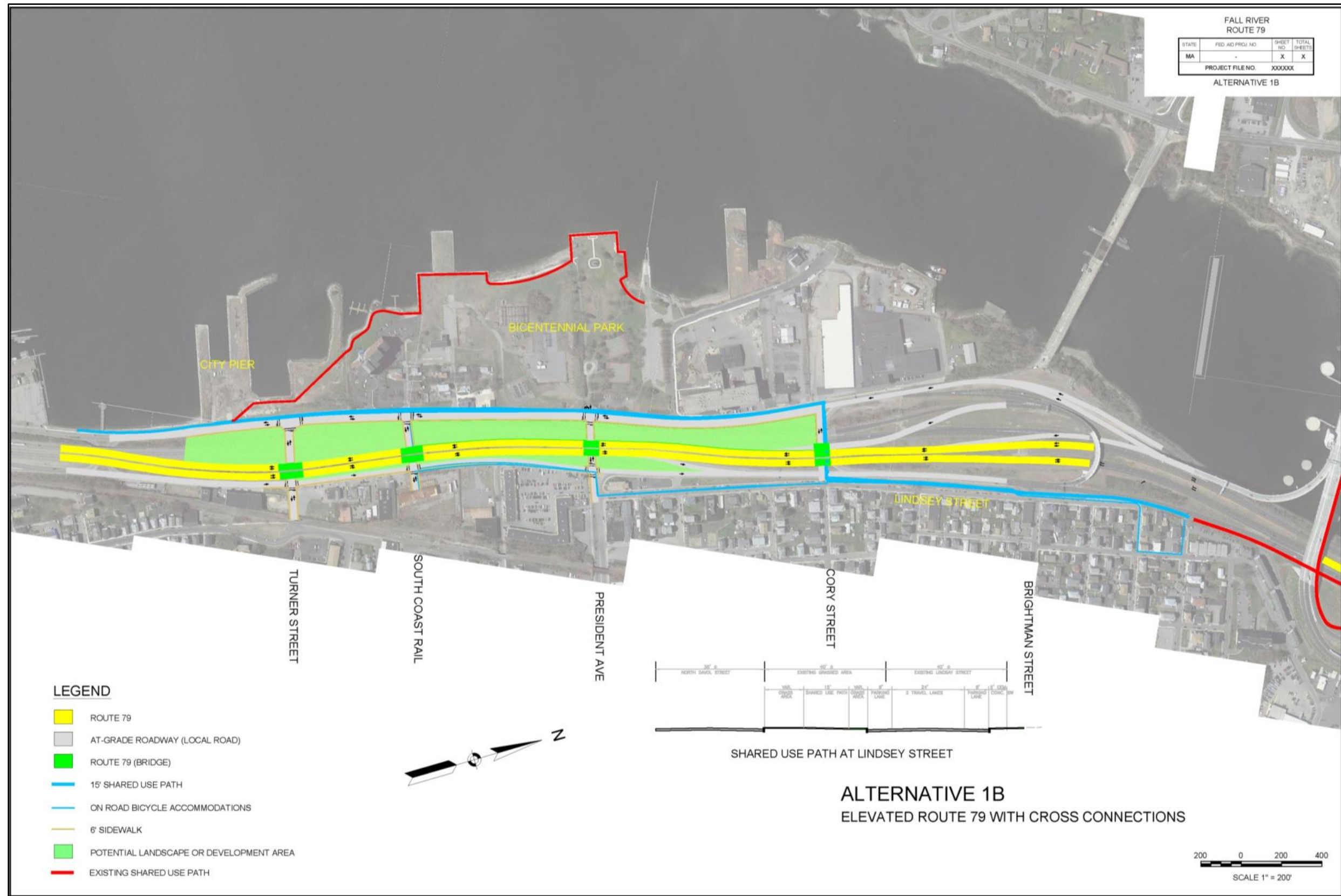
Figure 3.10: Alternative 1B – Elevated Route 79 with Cross Connections
