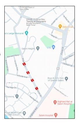
Four pairs of temporary, pre-fab speed cushions, purchased from Traffic Logix, were installed in 2022, resulting in 250 ft spacing. A centerline was striped as well, and flex posts were installed on the centerline at each cushion pair to deter motorists from trying to straddle two cushions. The cushions and flex posts are removed each winter. They were reinstalled in 2023 and are due to be reinstalled in 2024.
