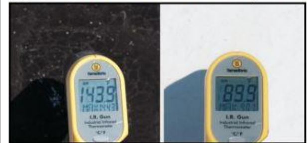
Figure 1: Dark vs. Cool Roof Surface Temperatures
