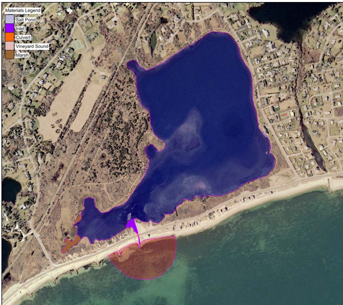
Figure VI-2. Map of Salt Pond water quality model longitudinal dispersion coefficients. Color patterns designate the different areas used to vary model dispersion coefficient values.
