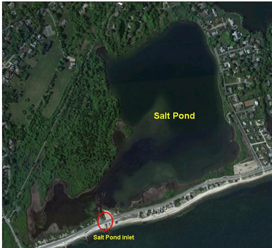
Figure I-2. Salt Pond embayment system for the Massachusetts Estuaries Project assessment and threshold analysis. Tidal waters enter the salt pond through one inlet to Vineyard Sound. Freshwaters enter from the watershed primarily through direct groundwater discharge, precipitation and stormwater from roads. The limited fringing wetland area results primarily from the limited tide range (0.25 ft) due to the restricted inlet.
