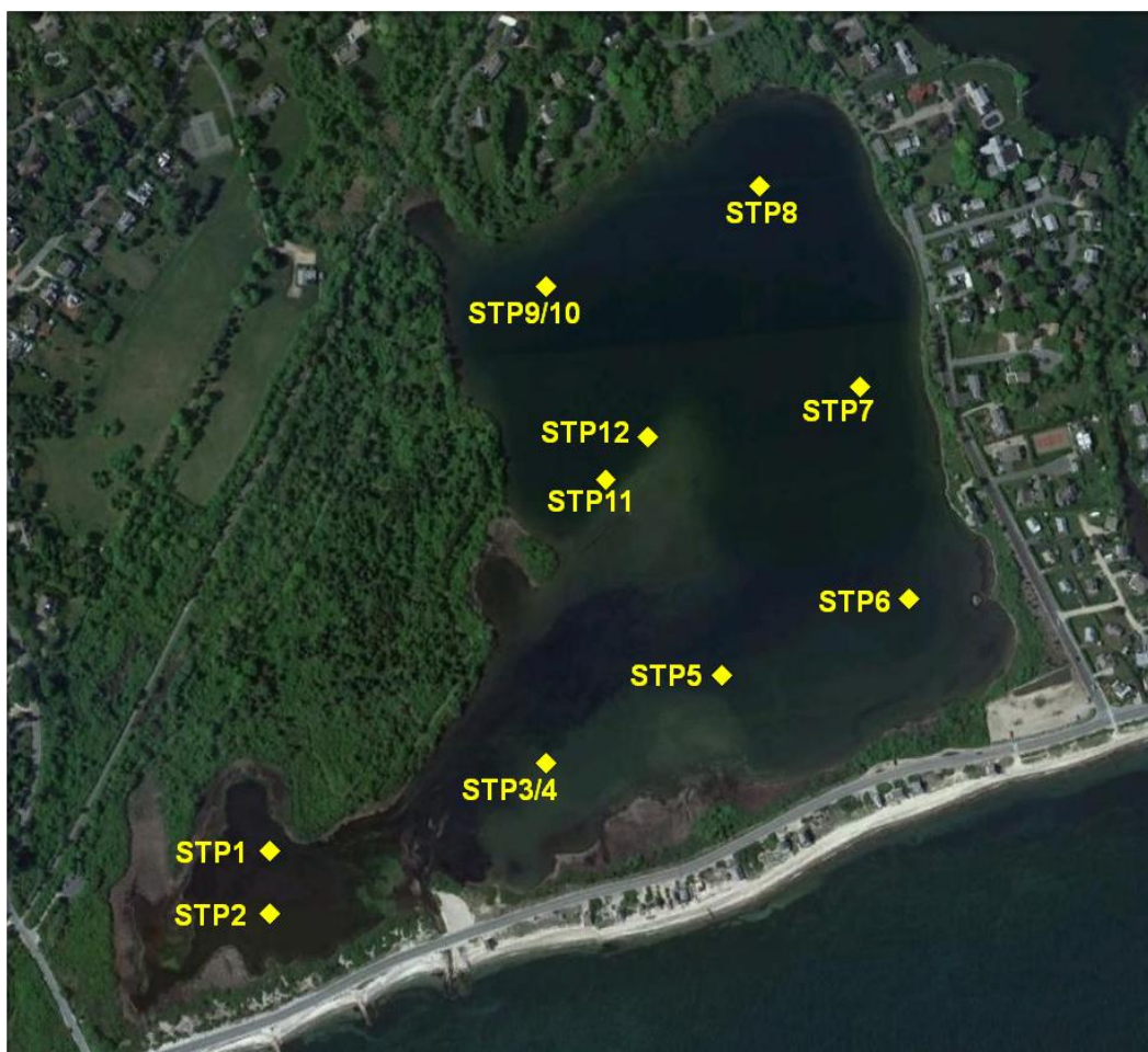
Figure IV-6. Salt Pond Estuary. Locations (yellow symbols) of sediment sample collection for determination of nitrogen regeneration rates and/or infaunal community analysis. Numbers are for reference to station listing above. Not all stations were sampled for both parameters.
