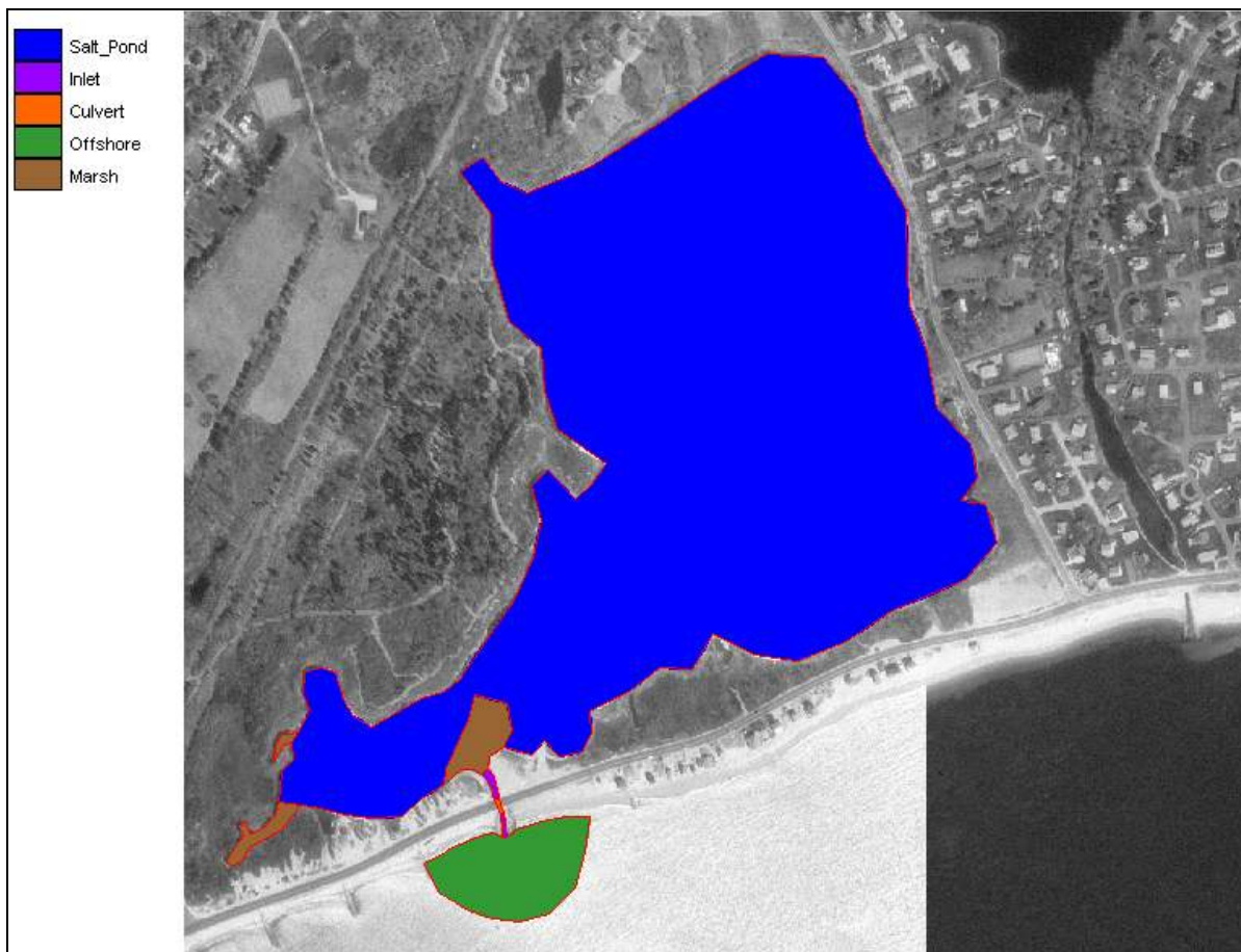
Figure V-7. Hydrodynamic model grid material properties. Color patterns designate the different model material types used to vary model calibration parameters and compute flushing rates.
