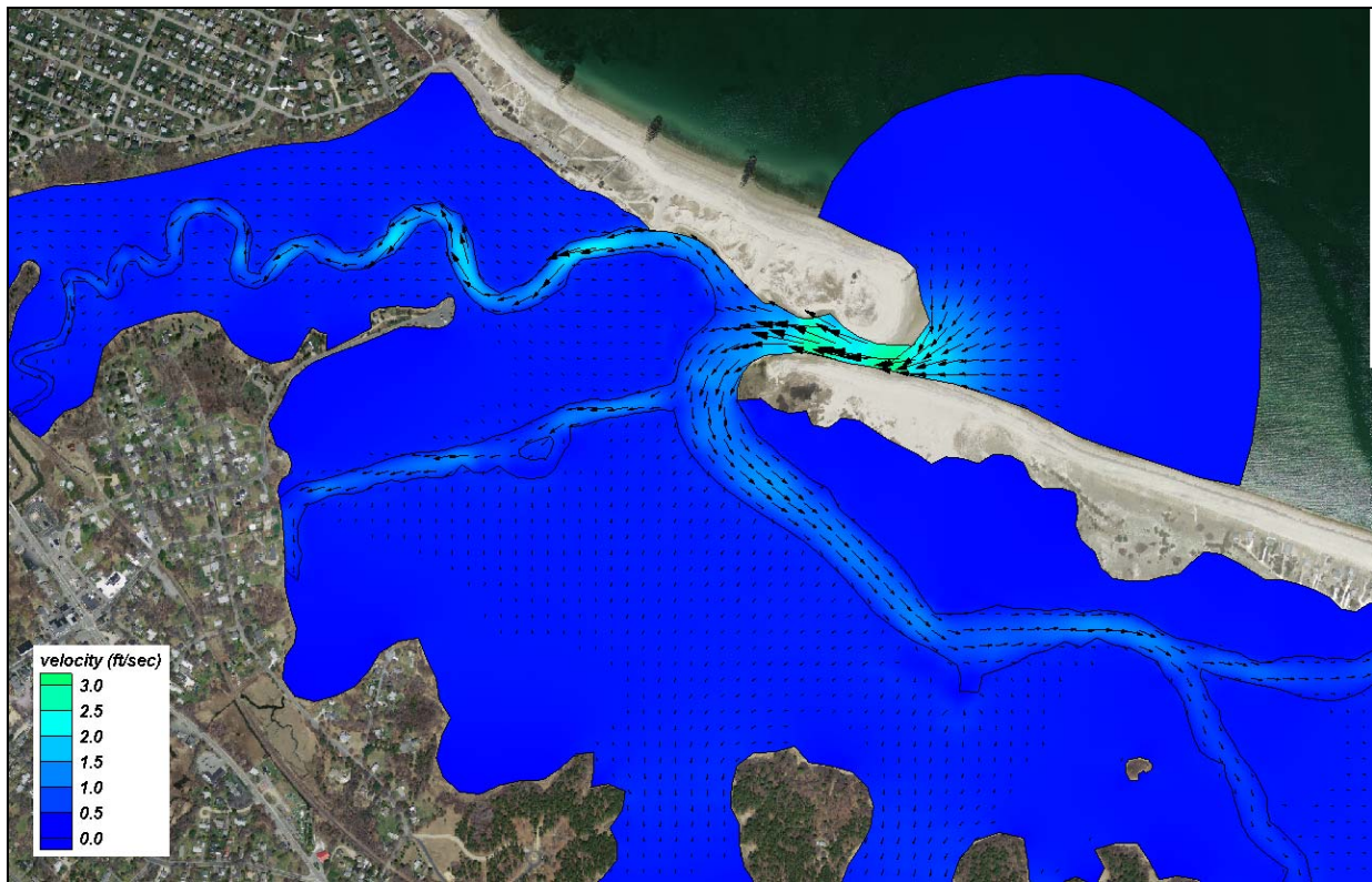
Figure V-14. Example of Sandwich Harbor hydrodynamic model output for a single time step during a flooding tide. Color contours indicate velocity magnitude, and vectors indicate the direction of flow. Areas of marsh are also shown as the solid black lines within the model domain.
