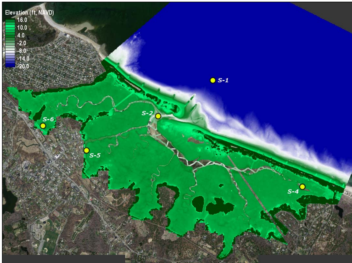
Figure V-2. Bathymetric/Topographic data used to develop the RMA-2 hydrodynamic model. Points are colored to represent the bottom elevation relative to NAVD. The data sources used to develop the grid mesh are the 2008 bathymetry survey, and the NOAA LiDAR data.
