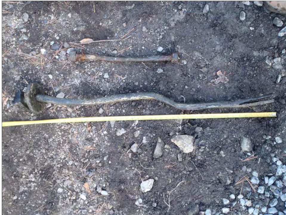
Figure 27. Bolt that attached two northern longitudinal timbers to bedrock.
