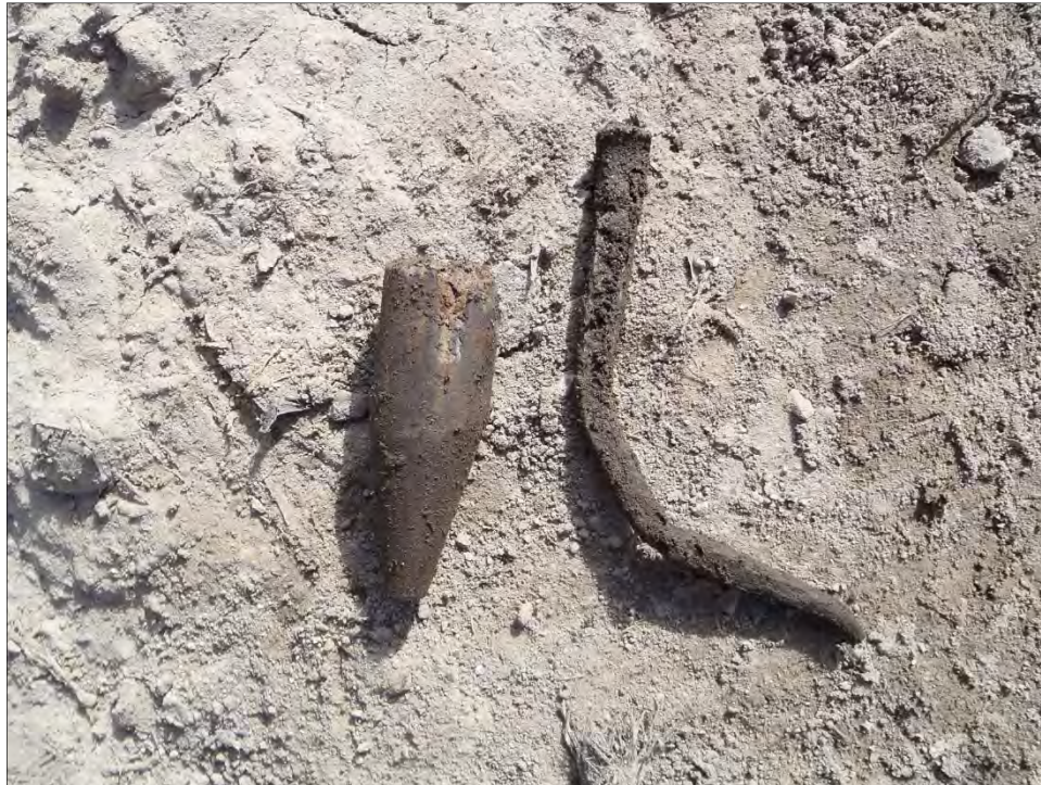
Figure 25. Wooden peg and machine-cut spike removed from northern longitudinal timber.
