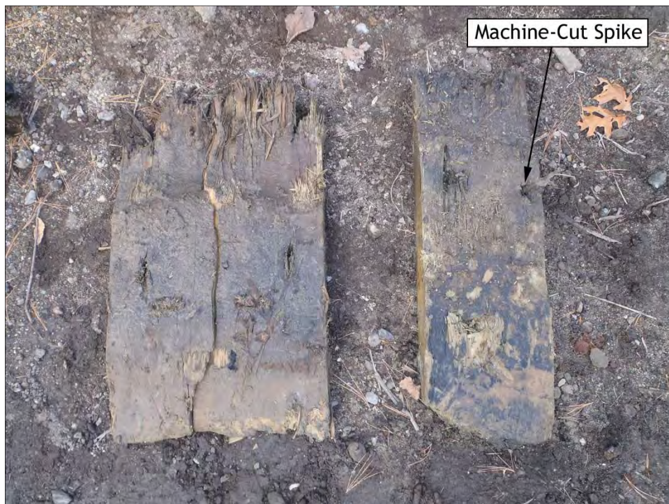
Figure 28. Representative sheet piling (with machine-cut spike) removed from lower northern timber for documentation.
