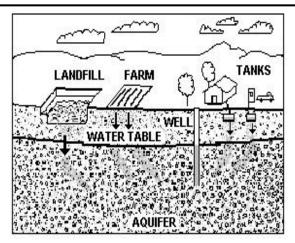
Figure 1: Example of how a well could become contaminated by different land uses and activities.
