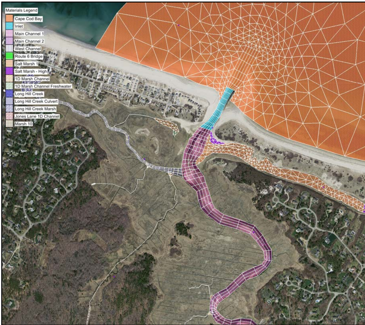
Figure V-8. Plot of hydrodynamic model grid mesh for Scorton Creek. Colors are used to designate the different model material types used to vary model calibration parameters and compute flushing rates.
