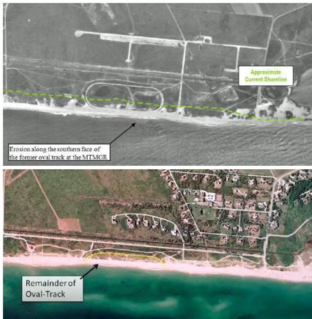
Aerial images of South Beach in 1952 (top) and 2010 (bottom). The oval target system from the naval gunnery range is intact and visible in the top photo; much of it had washed away by 2010. From Funk et al. (2011). (See Appendix G for photo information.)
