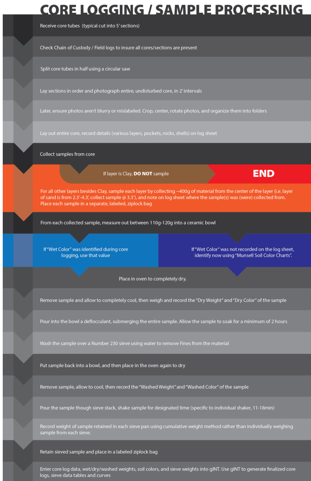
Figure 29: Flow chart depicting the steps for vibracore logging, sampling, and sample analysis.
