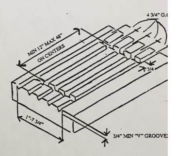
NOTE: The positive limiting barrier to be 5 continuous square or "V" grooves 3/4"x3/4" deep, on 4 3/4 centers with cross interconnecting grooves, either square or "V", equally spaced on min. 12" max. 48" centers. The outside groove to be at limits of hazard protection area and the potential spill area to be within this protection area.
