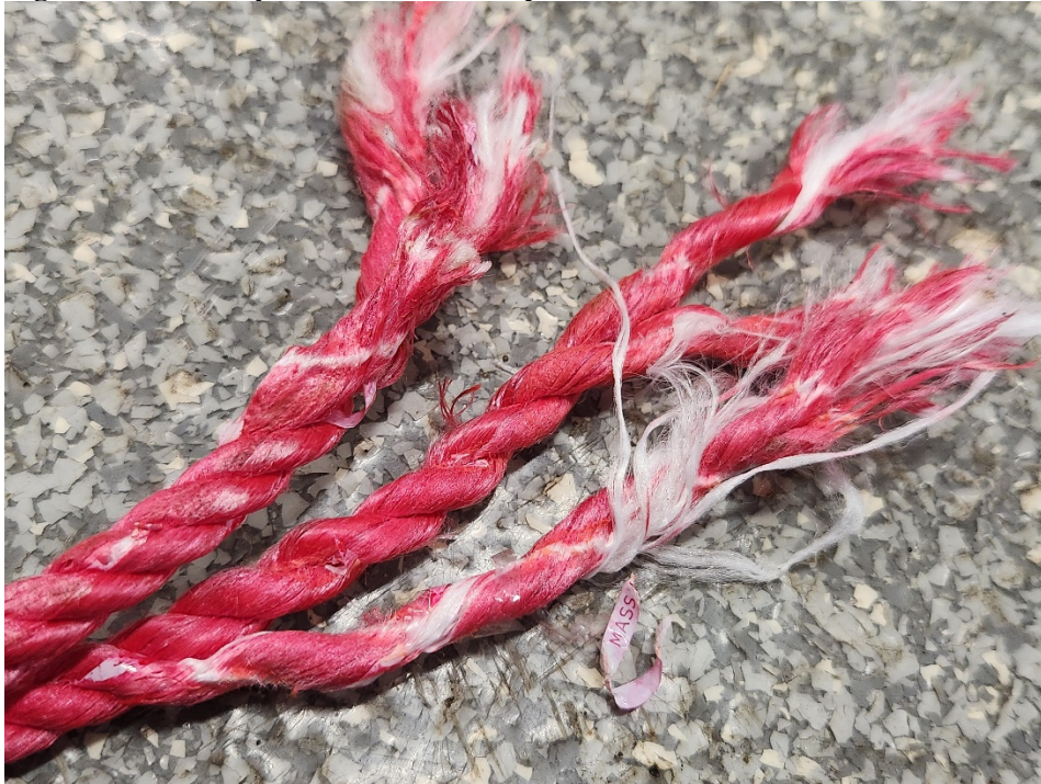
Figure 1. Red Fully Formed Weak Rope With Tracer
