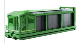
**General:** A self-contained, completely assembled above ground Air Curtain Burner (air curtain incinerator or FireBox) with a refractory lined burn-container and steel floor and fittings for cable-hoist trucks or hook-lift trucks in accordance with ANSI Specification Z245.60 for portable applications. The S116R is protected by US Patent Number 7895956.
