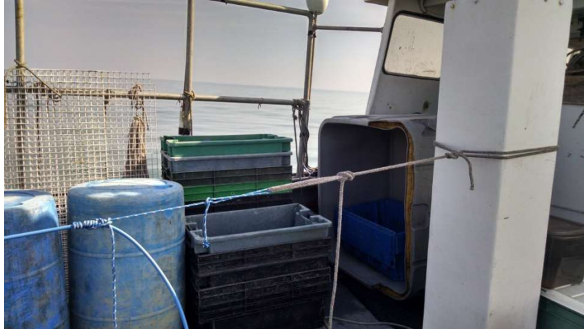
Figure 7C. Whipping knot securing blue tow cable to exhaust post on the centerline of the offshore lobster vessel.
