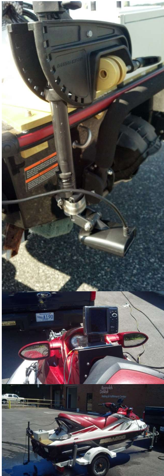
Figure 5. Jet ski and trolling motor mount of a Humminbird transducer.
