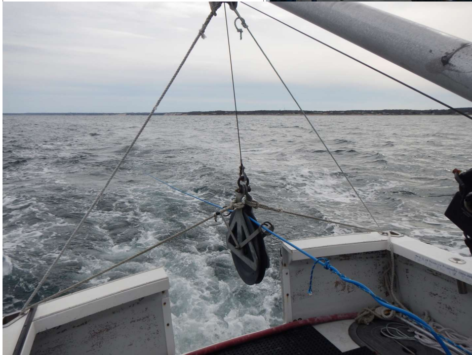
Figure 4. Deployment arrangements for a towfish on the Mya research vessel.
