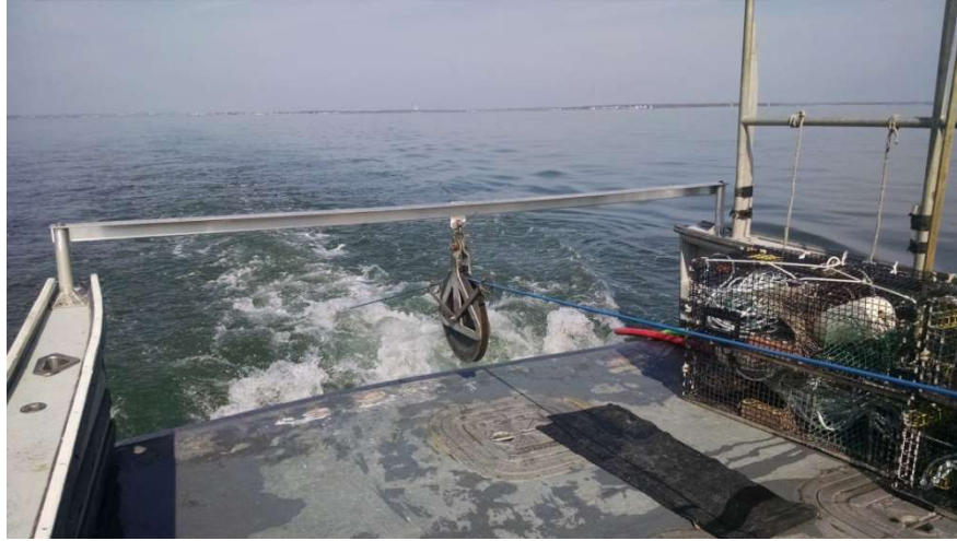
Figure 7A. Aluminum L-bracket bar across stern of an offshore lobster vessel. Sheave is hanging from the middle of the bar. It did begin to sag, so a pipe or U or square pipe bar might have been a better choice for longer-term work.
