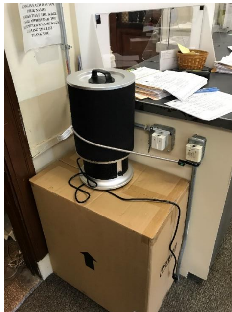
Photo 2 – Portable HEPA Filter
