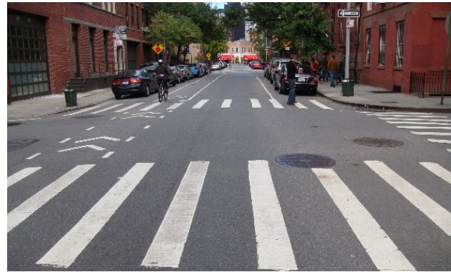
Figure 7-7 and 7-8. Bar or Zebra Crosswalks improve pedestrian safety and are more visible to drivers. Parallel Line (or Traverse Line) Crosswalk is less visible to drivers, particularly at night.
