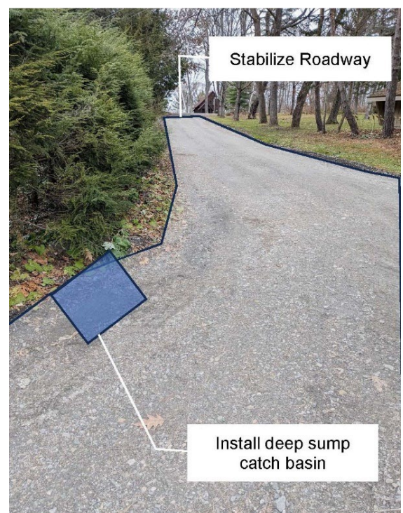
Photos C-11: Spruce Road BMPs: deep sump catch basin location at the intersection of Bridge Street (left photo) and catch basin location at corner of Spruce and Hemlock Streets (right photo)
