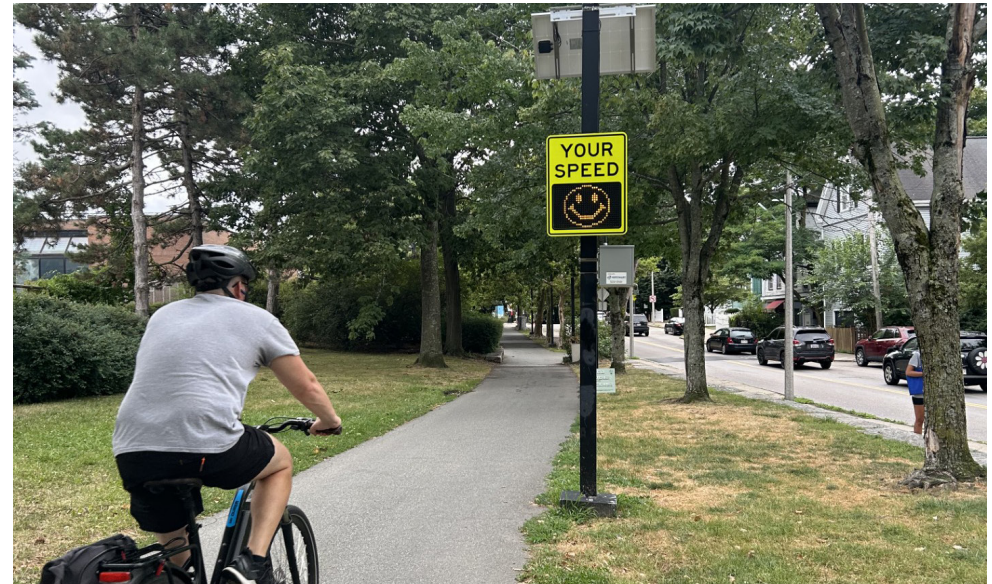
A feedback sign pilot is being evaluated to help slow speeds and potentially establish a speed limit for the corridor
