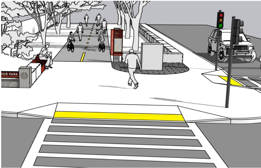
Widen curb ramps, and bring up to ADA/PROWAG compliance
