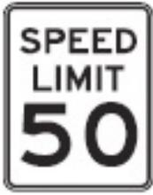
Speed limit signage that includes black legend on a white background indicates the presence of a regulatory limit. These are speed limits that have a special speed regulation and has been established in accordance with the Massachusetts General Laws (MGL) c. 90 § 18 and the MassDOT Procedures for Speed Zoning.
