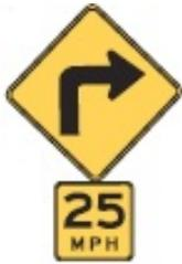
Advisory speed signs have a black legend on a yellow background and are used to supplement other warning signs of a condition that may require a reduction in operating speed, such as an approach to a sharp curve or winding road. Advisory speeds are not enforceable since their intent is to advise motorists of an appropriate speed, not regulate it.
