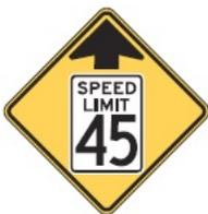
Reduced speed limit ahead signs are used to inform road users of an impending reduced speed zone where the speed limit is typically being reduced by 10 mph or more. Drivers should take proper care and begin reducing their speeds accordingly.
