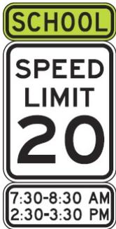
School zone speeds, which have been established in accordance with the Massachusetts Amendments to the MUTCD, are set at 20 mph for school zones in Massachusetts. School zone speed limit signs should be supplemented with times of day, a message stating "When Children Are Present," or flashing yellow beacons to indicate when the speed limit is in effect.
