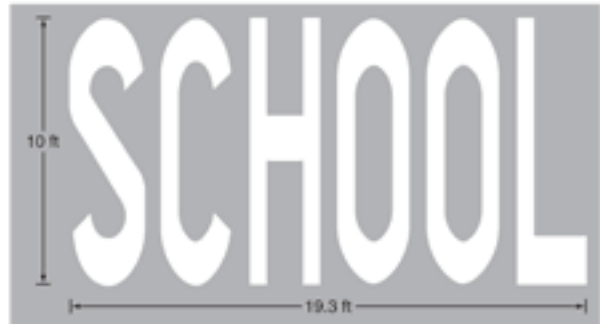
Figure 7C-1. Two-Lane Pavement Marking of "SCHOOL"
