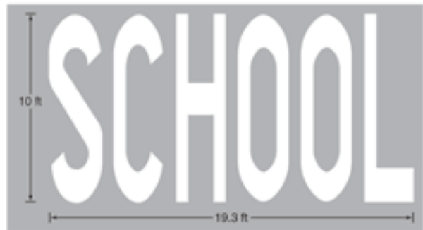
Figure 7C-1. Two-Lane Pavement Marking of "SCHOOL"
