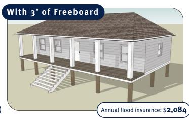
Elevating a home a few feet above legally mandated heights has very little effect on its overall look, yet it can lead to substantial reductions in flood insurance, substantially decrease the chances the home will be damaged by storms and flooding, and help protect against sea level rise.
