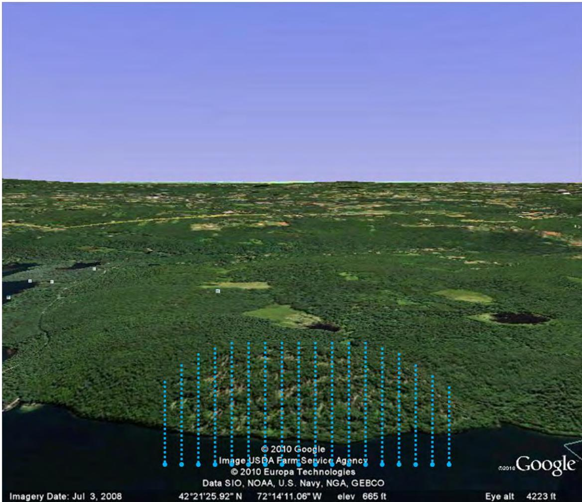
**Figure 5.7** – Google Earth image (altitude = 4,223 feet; oblique viewing angle, identical to Figures 5.6 and 5.8; 2X vertical exaggeration) of irregular shelterwood cut on the Hardwick Block of the Quabbin Forest. Regularly spaced flow paths (dashed blue lines), perpendicular to the slope contours, are superimposed on the image.
