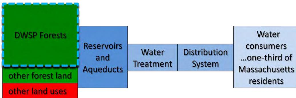
**Figure 1.2** – Simple schematic diagram of the DWSP/MWRA water supply system. Water treatment includes disinfection to kill pathogens (bacteria, giardia, etc.), fluoride addition, and pH and water chemistry adjustment to prevent corrosion in the water distribution system. Filtration is not required.
