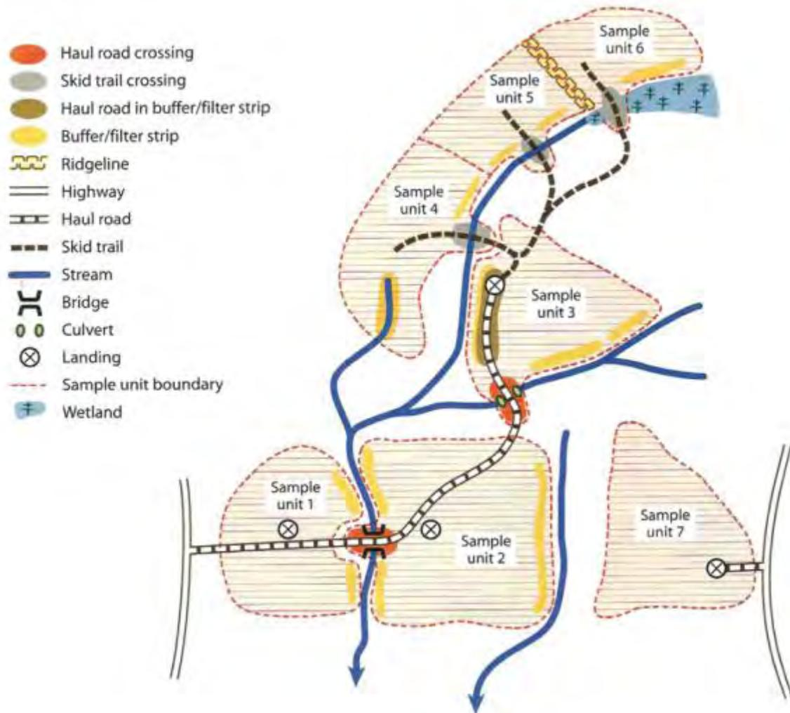
**Figure 6.5** –Definition sketch for sample unit delineation using harvest area boundaries, ownership boundaries, and stream or wetland crossings, US Forest Service Northeastern Area BMP monitoring protocol (Welsch et al., 2006)
