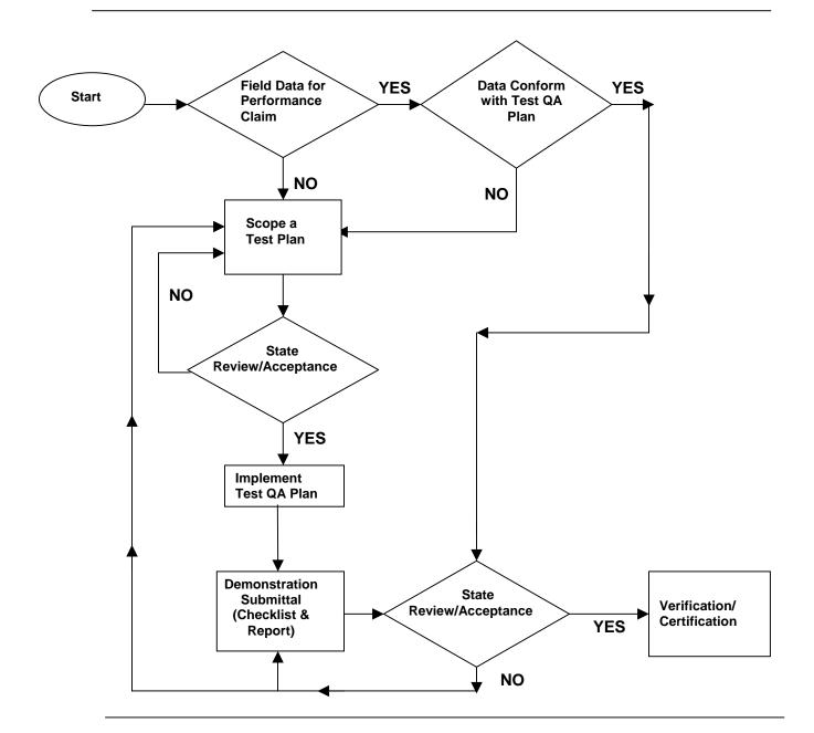
Figure 1. Overview of the Test QA Plan and Field Demonstration Review Processes
