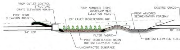
SEDIMENTATION FOREBAY & BIORETENTION BASIN B PROFILE
