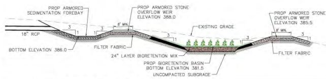
SEDIMENTATION FOREBAY & BIORETENTION BASIN A PROFILE
