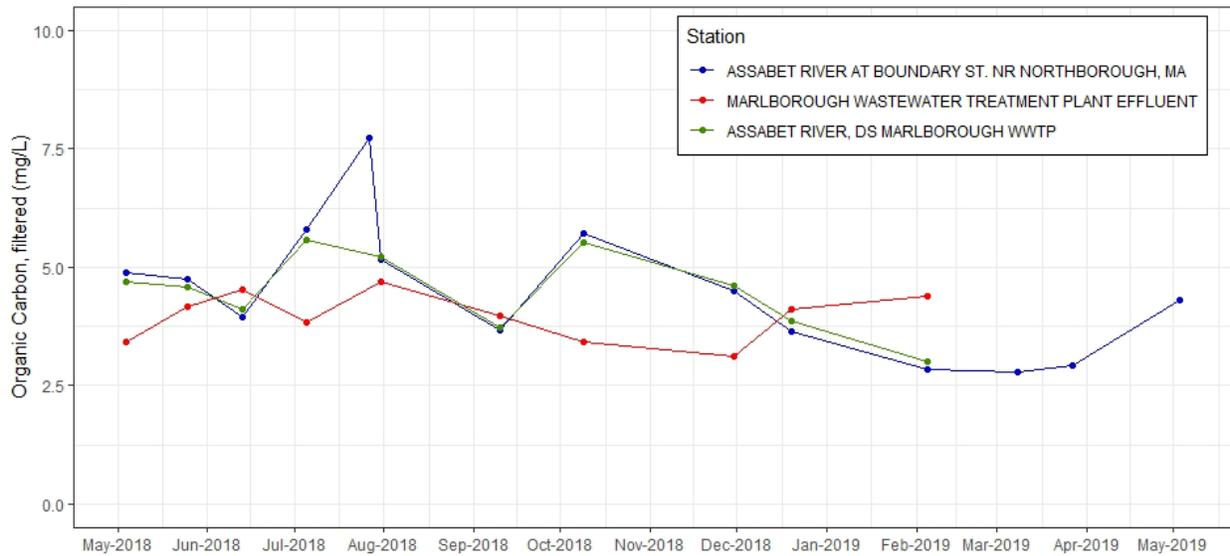
**Figure C-17.** Time series plot of organic carbon, filtered (mg/L) from discrete samples taken at effluent and ambient stations near Marlborough WWTF, 2018-2019. Note additional sample collected at Assabet River at Boundary St. near Northborough, MA on July 27, 2018 is not a replicate (see Table C-1 for detail).
