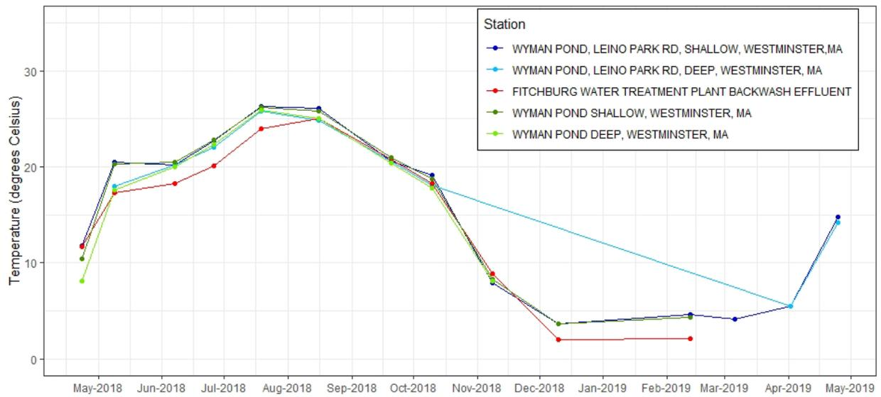
Figure C-66. Time series plot of water temperature ( $^{\circ}\text{C}$ ) from discrete samples taken at effluent and ambient stations near Fitchburg WTF, 2018-2019.
