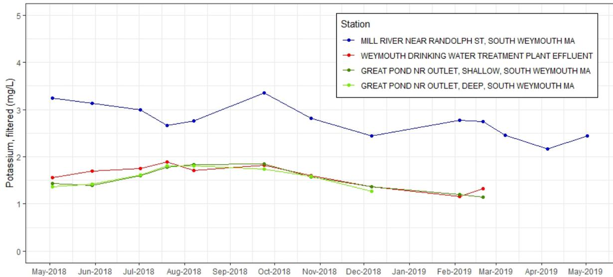
**Figure C-107.** Time series plot of Potassium, filtered (mg/L) from discrete samples taken at effluent and ambient stations near Weymouth WTF, 2018-2019.
