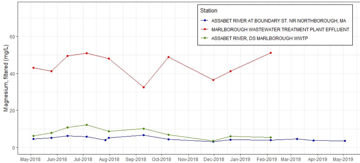
**Figure C-16.** Time series plot of magnesium, filtered (mg/L) from discrete samples taken at effluent and ambient stations near Marlborough WWTF, 2018-2019. Note additional sample collected at Assabet River at Boundary St. near Northborough, MA on July 27, 2018 is not a replicate (see Table C-1 for detail).
