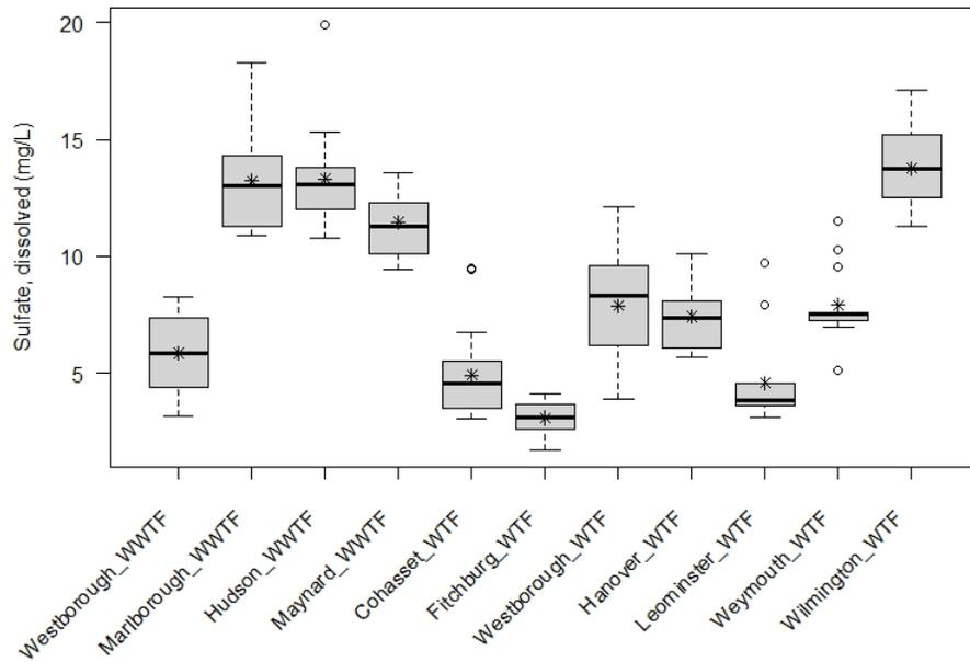
**Figure 12.** Boxplot of sulfate, filtered (mg/L), from discrete samples taken at selected ambient stations (upstream or pond) at 11 water or wastewater treatment facilities in eastern and central Massachusetts, 2018-2019. Data include only those from selected ambient stations used for copper criteria value calculations in the Biotic Ligand Model (BLM).
