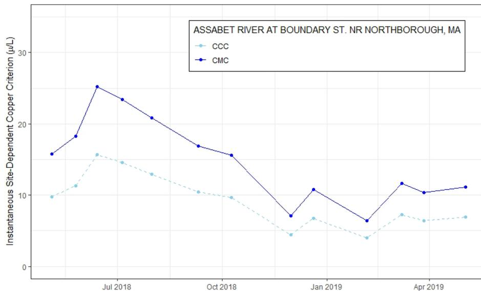
Figure D-2. Time series plot of site-dependent instantaneous Criteria Maximum Concentration (CMC) and Criteria Continuous Concentration (CCC) values ( $\mu\text{g/L}$ ) for ambient stations used in the BLM near Marlborough WWTF, 2018-2019.
