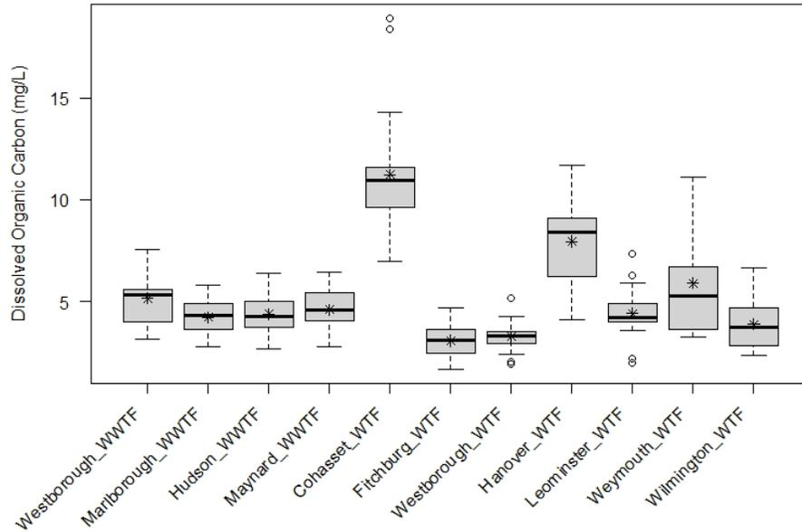
**Figure 8.** Boxplot of organic carbon, filtered (dissolved organic carbon (DOC); mg/L), from discrete samples taken at selected ambient stations (upstream or pond) at 11 water or wastewater treatment facilities in eastern and central Massachusetts, 2018-2019. Data include only those from selected ambient stations used for copper criteria value calculations in the Biotic Ligand Model (BLM).
