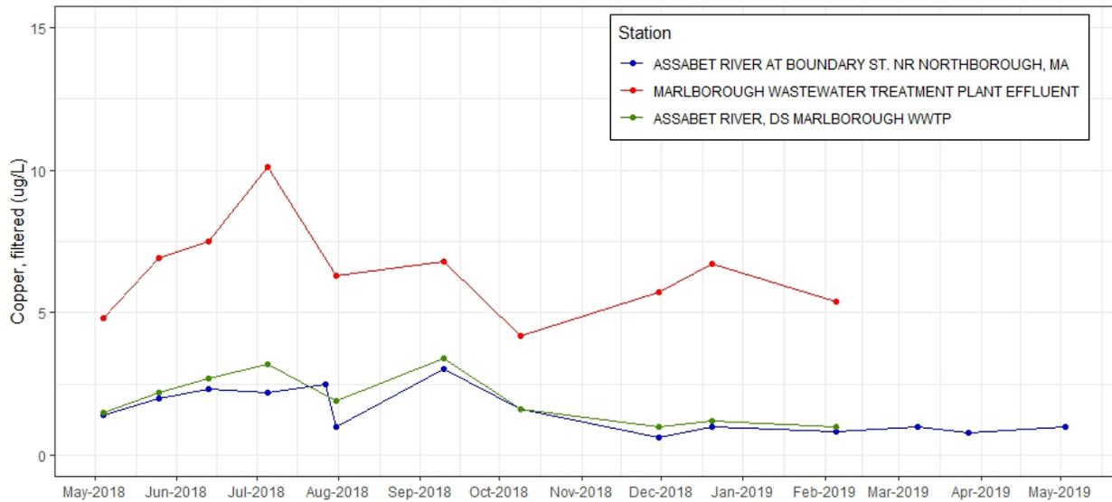
**Figure C-15.** Time series plot of copper, filtered (µg/L) from discrete samples taken at effluent and ambient stations near Marlborough WWTF, 2018-2019. Note additional sample collected at Assabet River at Boundary St. near Northborough, MA on July 27, 2018 is not a replicate (see Table C-1 for detail).
