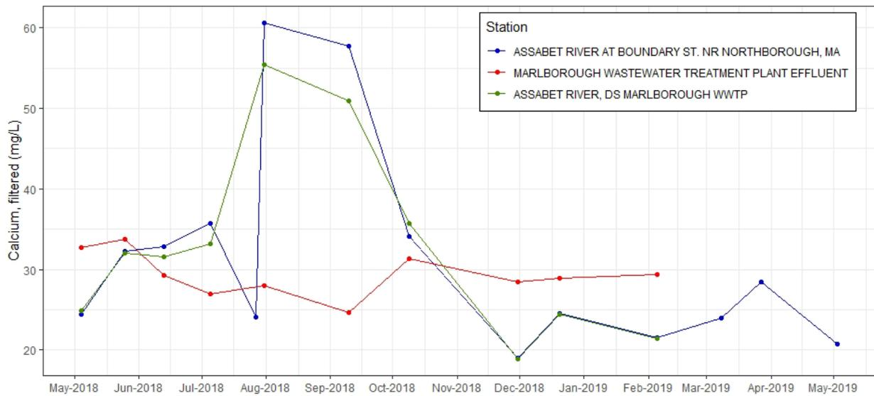
**Figure C-13.** Time series plot of calcium, filtered (mg/L) from discrete samples taken at effluent and ambient stations near Marlborough WWTF, 2018-2019. Note additional sample collected at Assabet River at Boundary St. near Northborough, MA on July 27, 2018 is not a replicate (see Table C-1 for detail).
