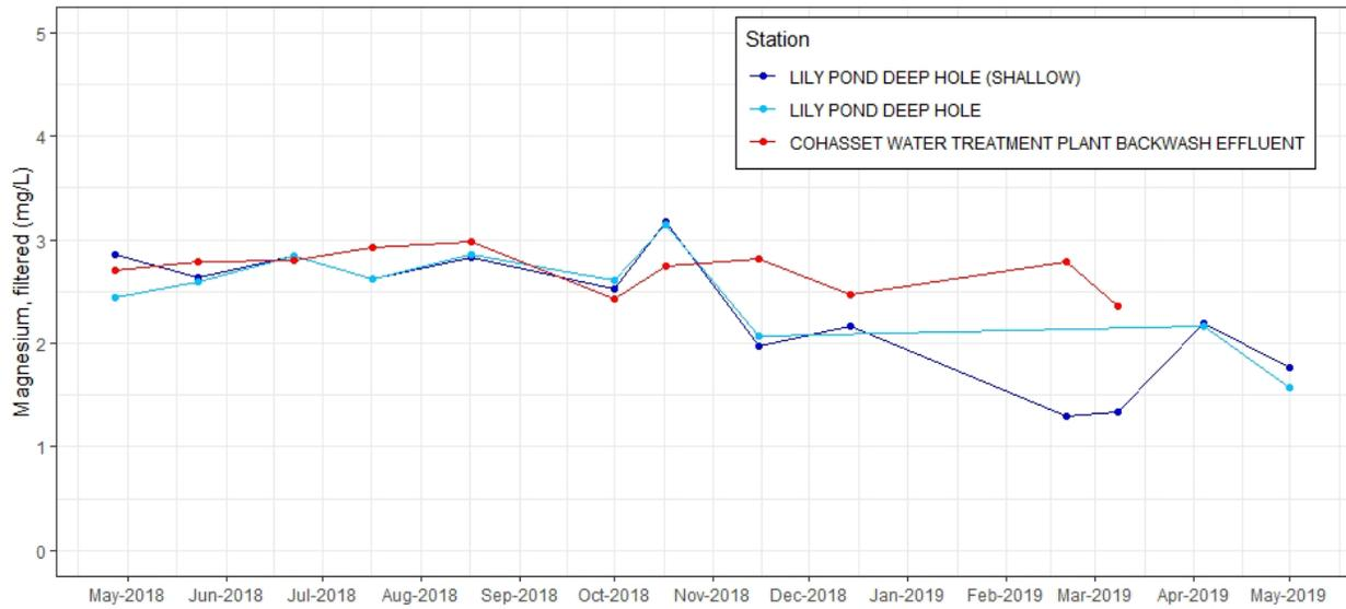
*Figure C-49. Time series plot of magnesium, filtered (mg/L) from discrete samples taken at effluent and ambient stations near Cohasset WTF, 2018-2019.*
