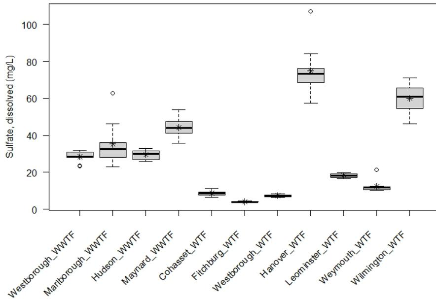
**Figure B-10.** Boxplot of sulfate, filtered (mg/L), from discrete samples taken at effluent stations at 11 water or wastewater treatment facilities in eastern and central Massachusetts, 2018-2019.
