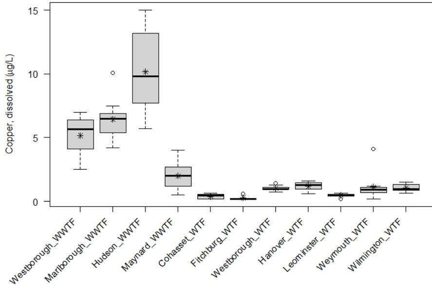
**Figure B-4.** Boxplot of copper, filtered ( $\mu\text{g/L}$ ), from discrete samples taken at effluent stations at 11 water or wastewater treatment facilities in eastern and central Massachusetts, 2018-2019.
