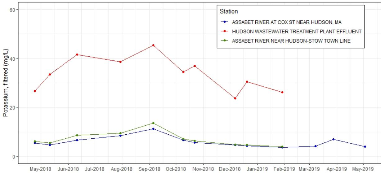
**Figure C-30.** Time series plot of Potassium, filtered (mg/L) from discrete samples taken at effluent and ambient stations near Hudson WWTF, 2018-2019.
