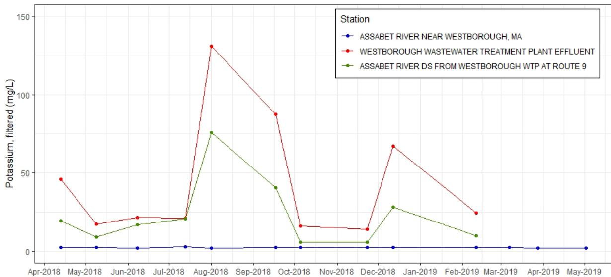
**Figure C-8.** Time series plot of potassium, filtered (mg/L) from discrete samples taken at effluent and ambient stations near Westborough WWTF, 2018-2019.
