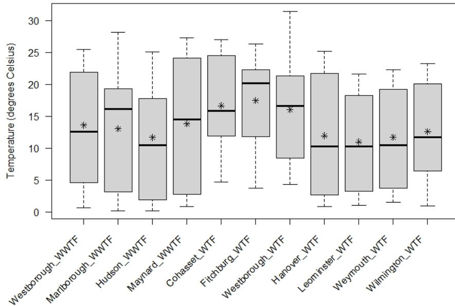
**Figure 13.** Boxplot of temperature (°C) from discrete samples taken at selected ambient stations (upstream or pond) at 11 water or wastewater treatment facilities in eastern and central Massachusetts, 2018-2019. Data include only those from selected ambient stations used for copper criteria value calculations in the Biotic Ligand Model (BLM).
