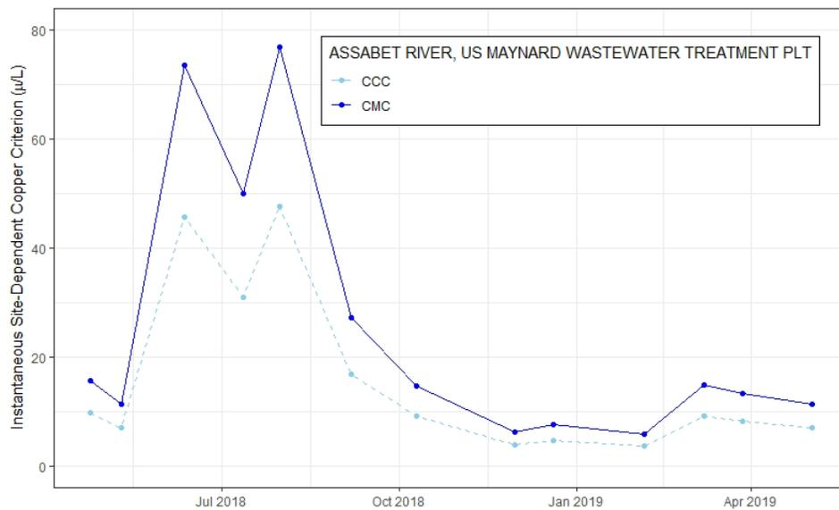
Figure D-4. Time series plot of site-dependent instantaneous Criteria Maximum Concentration (CMC) and Criteria Continuous Concentration (CCC) values ( $\mu\text{g/L}$ ) for ambient stations used in the BLM near Maynard WWTF, 2018-2019.
