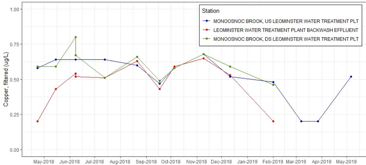
**Figure C-92.** Time series plot of copper, filtered (ug/L) from discrete samples taken at effluent and ambient stations near Leominster WTF, 2018-2019. Note additional samples collected at Leominster Water Treatment Plant Backwash Effluent and Monoosnoc Brook, DS Leominster Water Treatment Plt on June 8, 2018 are not replicates (see Table C-1 for detail).
