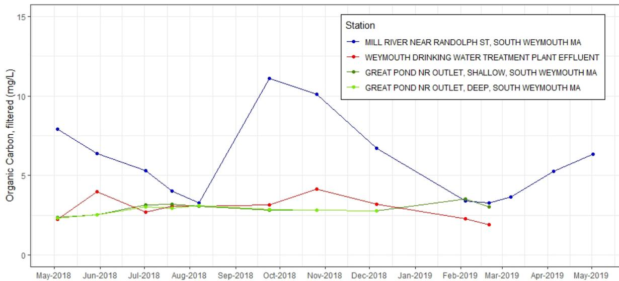
**Figure C-105.** Time series plot of Organic Carbon, filtered (mg/L) from discrete samples taken at effluent and ambient stations near Weymouth WTF, 2018-2019.
