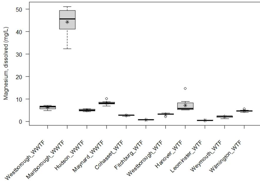
**Figure B-5.** Boxplot of magnesium, filtered (mg/L) from discrete samples taken at effluent stations at 11 water or wastewater treatment facilities in eastern and central Massachusetts, 2018-2019.
