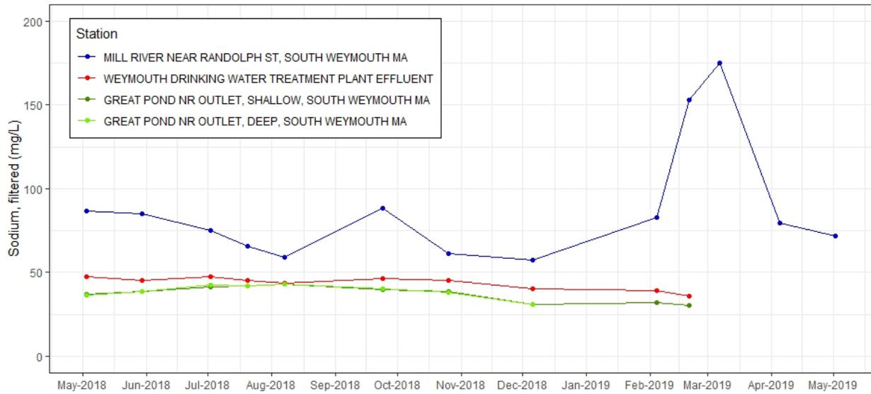
**Figure C-108.** Time series plot of Sodium, filtered (mg/L) from discrete samples taken at effluent and ambient stations near Weymouth WTF, 2018-2019.
