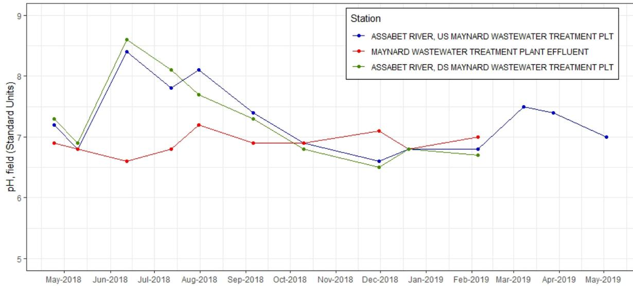
**Figure C-40.** Time series plot of pH (SU) from discrete samples taken at effluent and ambient stations near Maynard WWTF, 2018-2019.
