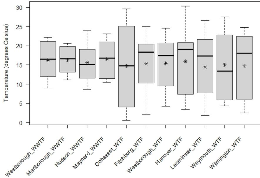
**Figure B-11.** Boxplot of temperature (°C) from discrete samples taken at effluent stations at 11 water or wastewater treatment facilities in eastern and central Massachusetts, 2018-2019.
