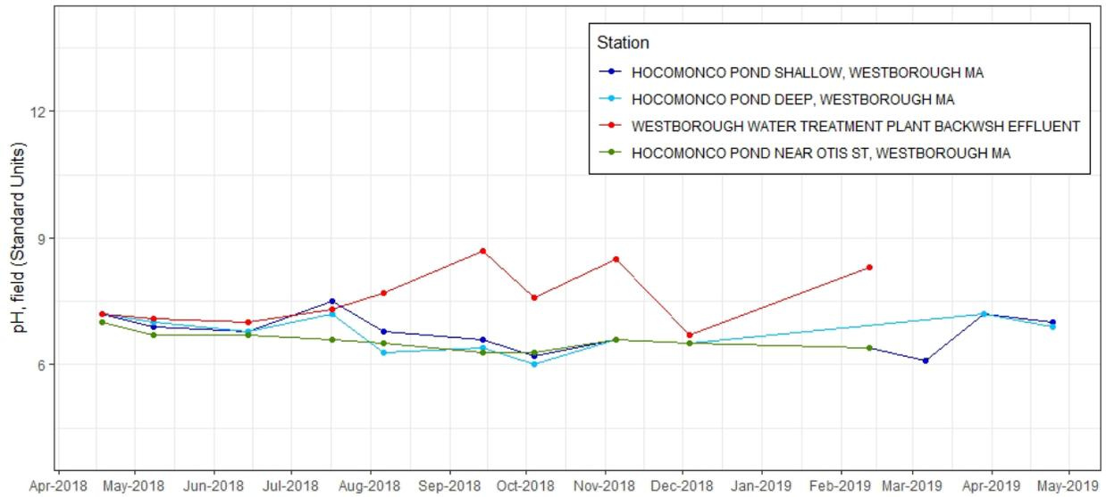
**Figure C-73.** Time series plot of pH (SU) from discrete samples taken at effluent and ambient stations near Westborough WTF, 2018-2019.
