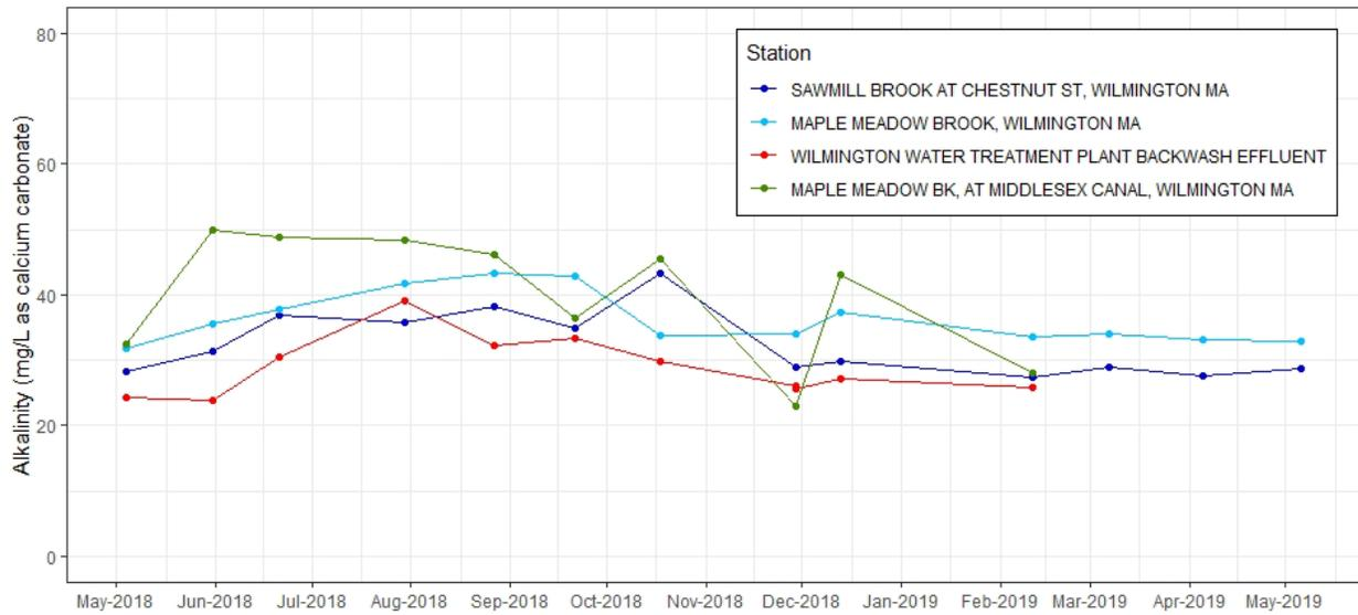
**Figure C-111.** Time series plot of Alkalinity, filtered (mg/L as calcium carbonate) from discrete samples taken at effluent and ambient stations near Wilmington WTF, 2018-2019. Note additional sample collected at Wilmington Water Treatment Plant Backwash Effluent on November 29, 2018 is not a replicate (see Table C-1 for detail).
