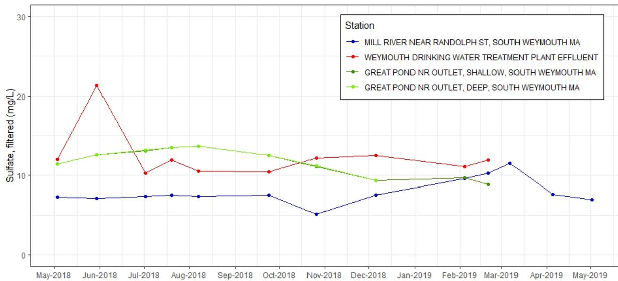
**Figure C-109.** Time series plot of Sulfate, filtered (mg/L) from discrete samples taken at effluent and ambient stations near Weymouth WTF, 2018-2019.
