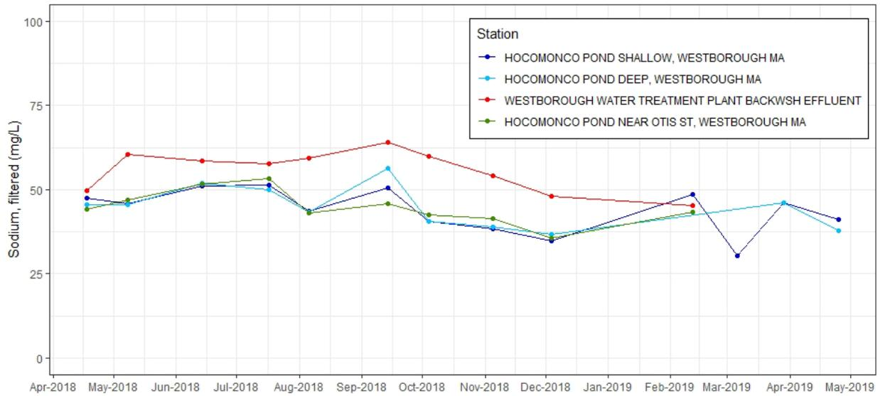
**Figure C-75.** Time series plot of sodium, filtered (mg/L) from discrete samples taken at effluent and ambient stations near Westborough WTF, 2018-2019.
