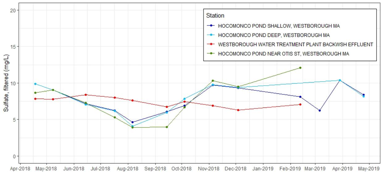
**Figure C-76.** Time series plot of sulfate, filtered (mg/L) from discrete samples taken at effluent and ambient stations near Westborough WTF, 2018-2019.
