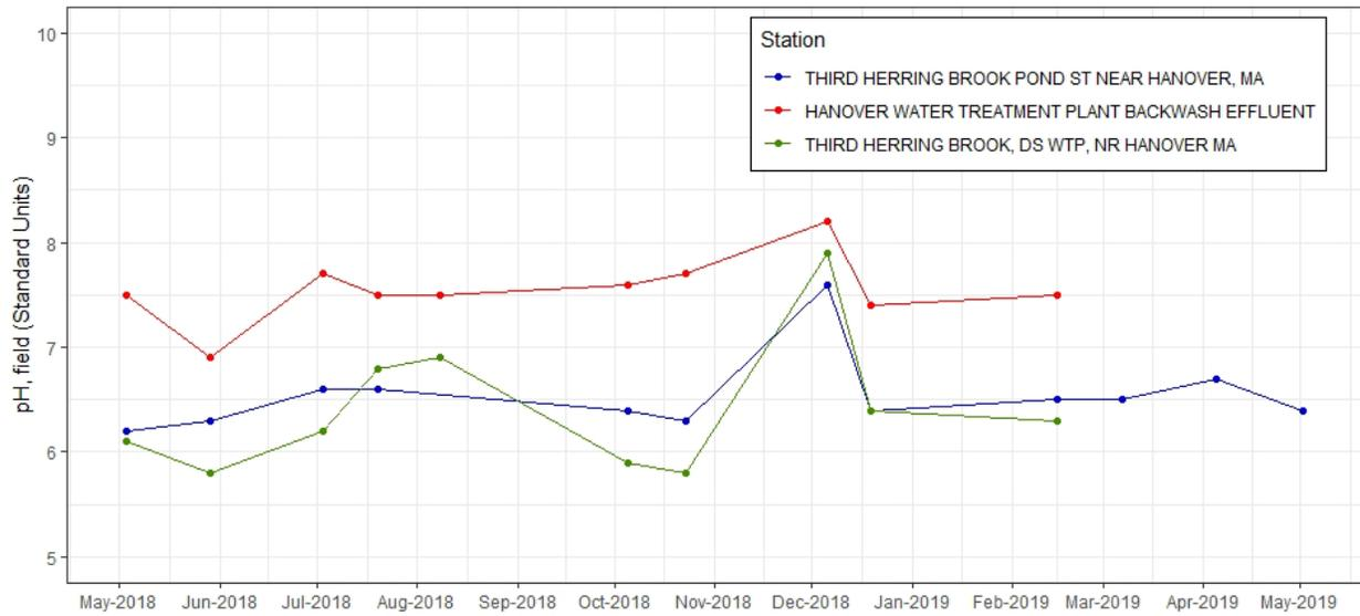
**Figure C-84.** Time series plot of pH (SU) from discrete samples taken at effluent and ambient stations near Hanover WTF, 2018-2019. Note additional sample collected at Hanover Water Treatment Plant Backwash Effluent on August 8, 2018 is not a replicate (see Table C-1 for detail).
