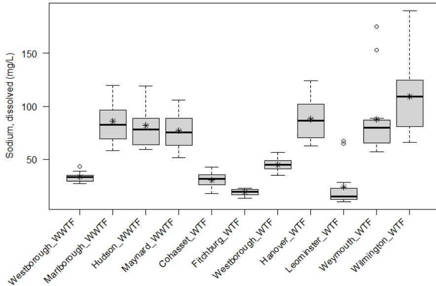
**Figure 11.** Boxplot of sodium, filtered (mg/L), from discrete samples taken at selected ambient stations (upstream or pond) at 11 water or wastewater treatment facilities in eastern and central Massachusetts, 2018-2019. Data include only those from selected ambient stations used for copper criteria value calculations in the Biotic Ligand Model (BLM).
