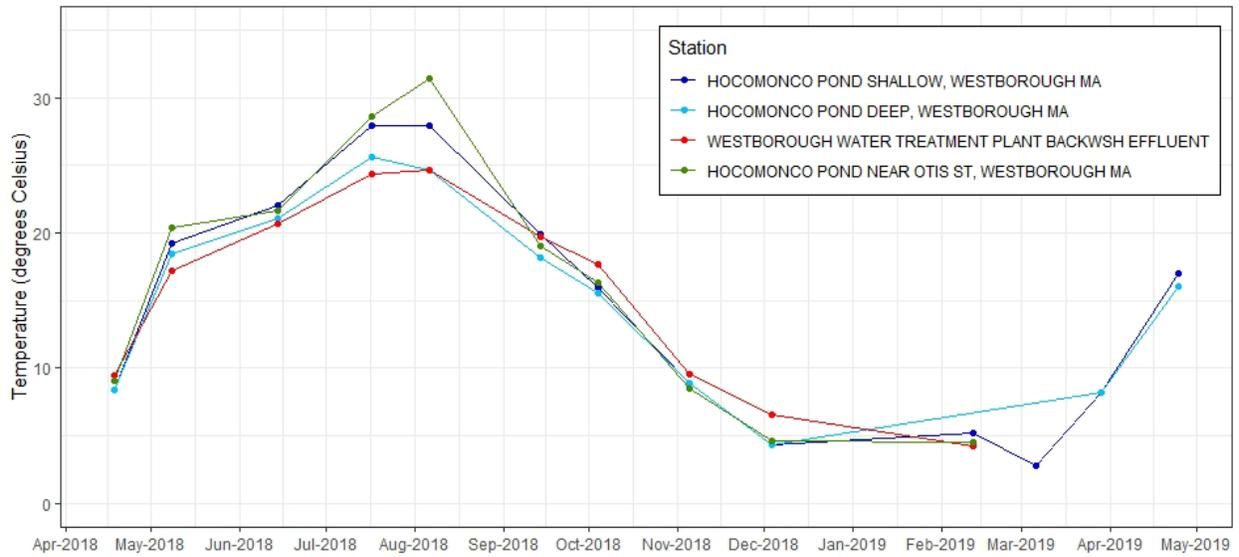
Figure C-77. Time series plot of water temperature (°C) from discrete samples taken at effluent and ambient stations near Westborough WTF, 2018-2019.
