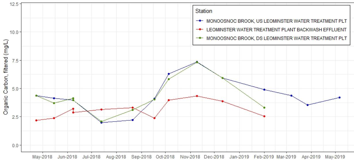
**Figure C-94.** Time series plot of organic carbon, filtered (mg/L) from discrete samples taken at effluent and ambient stations near Leominster WTF, 2018-2019. Note additional samples collected at Leominster Water Treatment Plant Backwash Effluent and Monoosnoc Brook, DS Leominster Water Treatment Plt on June 8, 2018 are not replicates (see Table C-1 for detail).
