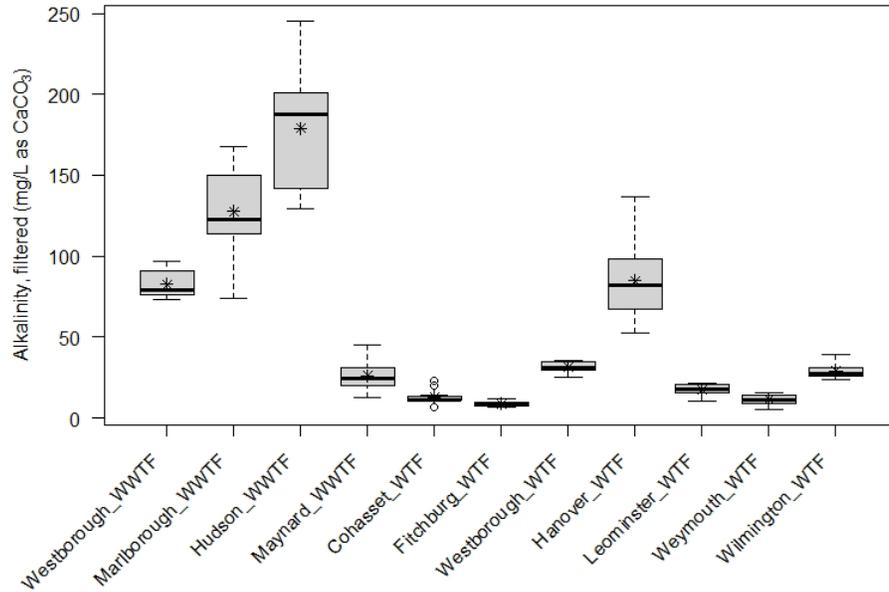
**Figure B-1.** Boxplot of alkalinity (mg/L as CaCO<sub>3</sub>) from discrete samples taken at effluent stations at 11 water or wastewater treatment facilities in eastern and central Massachusetts, 2018-2019.
