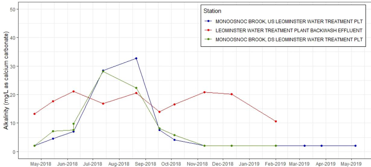
**Figure C-89.** Time series plot of alkalinity, filtered (mg/L as calcium carbonate) from discrete samples taken at effluent and ambient stations near Leominster WTF, 2018-2019. Note additional samples collected at Leominster Water Treatment Plant Backwash Effluent and Monoosnoc Brook, DS Leominster Water Treatment Plt on June 8, 2018 are not replicates (see Table C-1 for detail).
