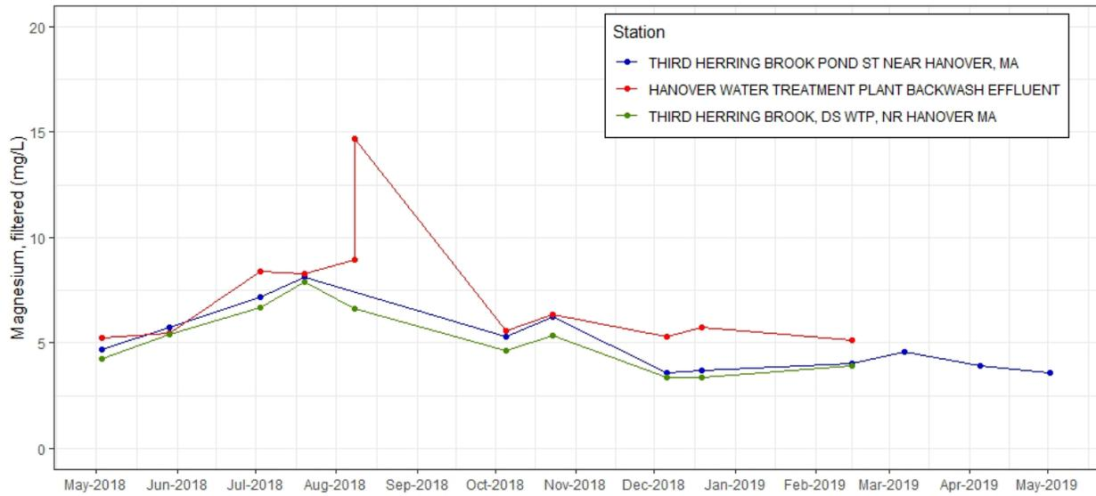
**Figure C-82.** Time series plot of magnesium, filtered (mg/L) from discrete samples taken at effluent and ambient stations near Hanover WTF, 2018-2019. Note additional sample collected at Hanover Water Treatment Plant Backwash Effluent on August 8, 2018 is not a replicate (see Table C-1 for detail).
