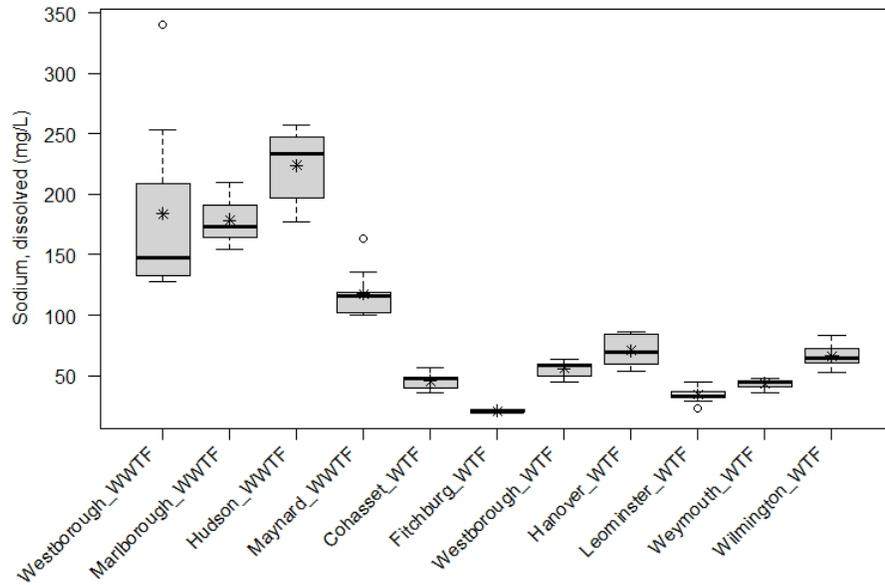
**Figure B-9.** Boxplot of sodium, filtered (mg/L), from discrete samples taken at effluent stations at 11 water or wastewater treatment facilities in eastern and central Massachusetts, 2018-2019.
