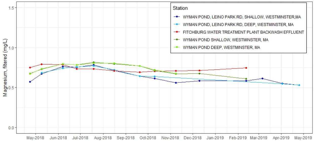
**Figure C-60.** Time series plot of magnesium, filtered (mg/L) from discrete samples taken at effluent and ambient stations near Fitchburg WTF, 2018-2019.
