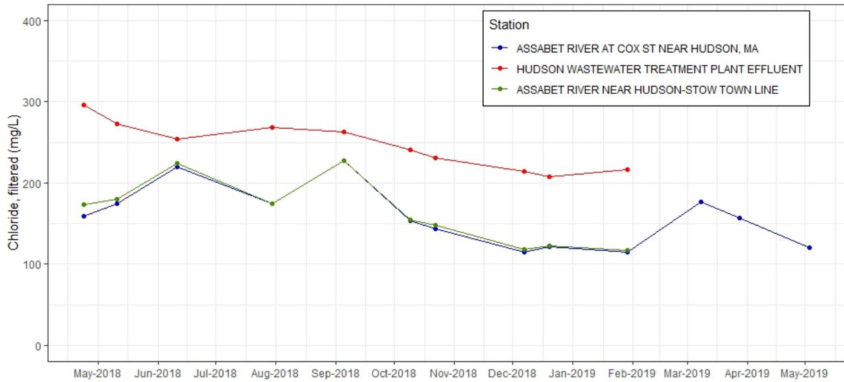
*Figure C-25. Time series plot of chloride, filtered (mg/L) from discrete samples taken at effluent and ambient stations near Hudson WWTF, 2018-2019.*
