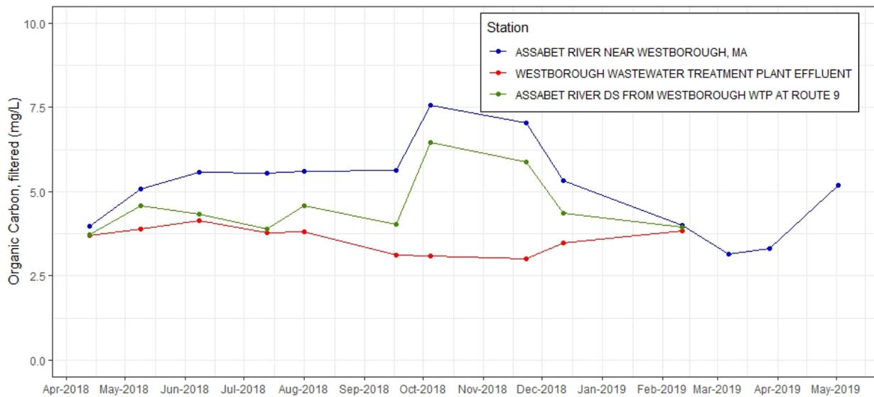
**Figure C-6.** Time series plot of organic carbon, filtered (mg/L) from discrete samples taken at effluent and ambient stations near Westborough WWTF, 2018-2019.
