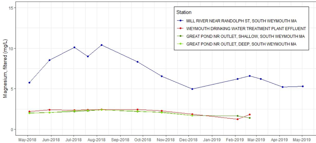
**Figure C-104.** Time series plot of Magnesium, filtered (mg/L) from discrete samples taken at effluent and ambient stations near Weymouth WTF, 2018-2019.
