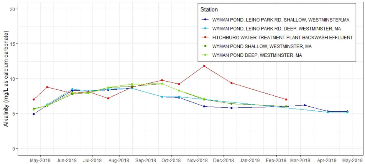
**Figure C-56.** Time series plot of alkalinity, filtered (mg/L as calcium carbonate) from discrete samples taken at effluent and ambient stations near Fitchburg WTF, 2018-2019.
