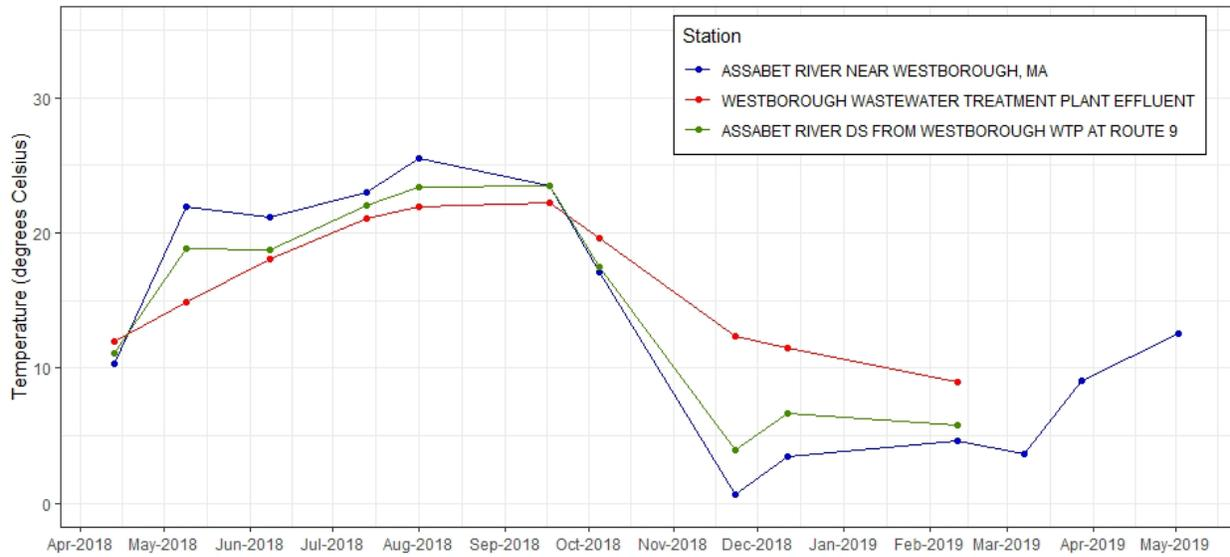
**Figure C-11.** Time series plot of water temperature (°C) from discrete samples taken at effluent and ambient stations near Westborough WWTF, 2018-2019.
