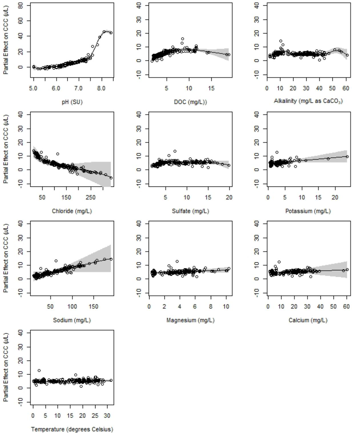
Figure 16. Smooth partial effects plots for the Generalized Additive Model (GAM) for chronic (criterion continuous concentration, CCC) values as a function of each input parameter to the Biotic Ligand Model (BLM). The y-axis is the smooth or spline function partial effect in response to the respective BLM input parameter. Shaded area indicates the 95% confidence interval for the mean shape of the effect.
