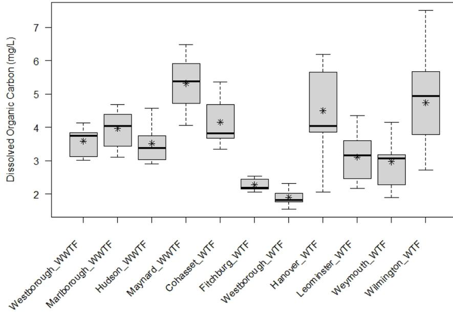
Figure B-6. Boxplot of dissolved organic carbon, filtered (mg/L), from discrete samples taken at effluent stations at 11 water or wastewater treatment facilities in eastern and central Massachusetts, 2018-2019.
