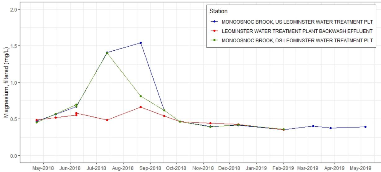
**Figure C-93.** Time series plot of magnesium, filtered (mg/L) from discrete samples taken at effluent and ambient stations near Leominster WTF, 2018-2019. Note additional samples collected at Leominster Water Treatment Plant Backwash Effluent and Monoosnoc Brook, DS Leominster Water Treatment Plt on June 8, 2018 are not replicates (see Table C-1 for detail).
