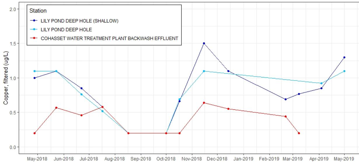
**Figure C-48.** Time series plot of copper, filtered (µg/L) from discrete samples taken at effluent and ambient stations near Cohasset WTF, 2018-2019.
