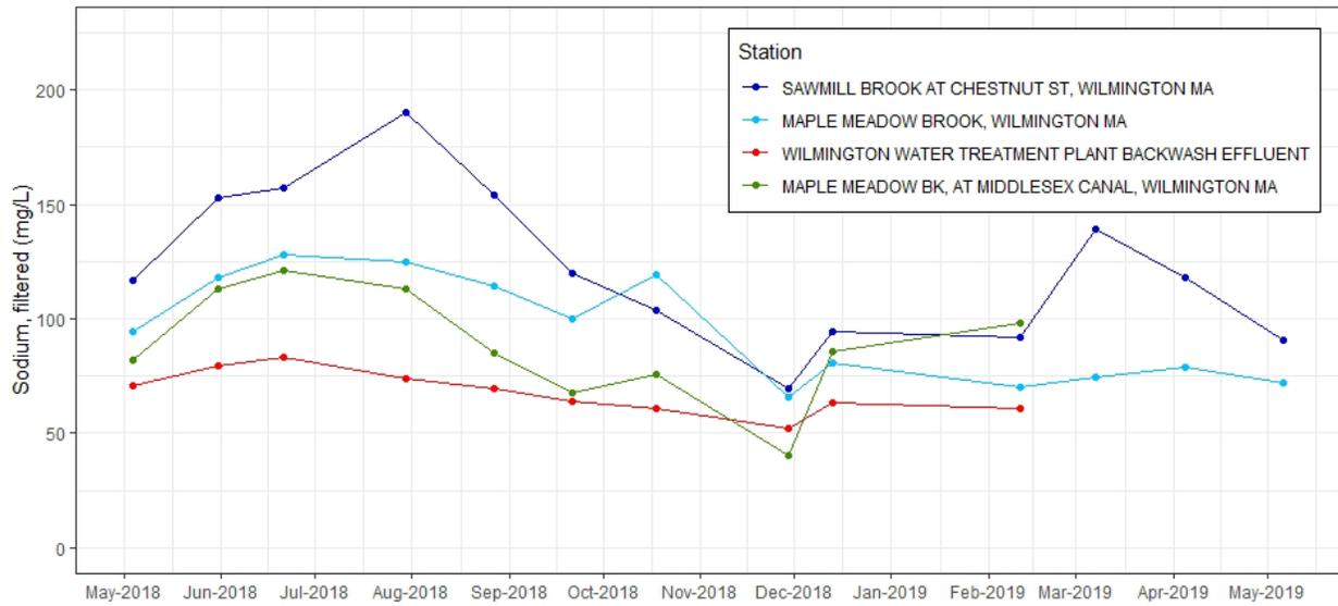
**Figure C-119.** Time series plot of Sodium, filtered (mg/L) from discrete samples taken at effluent and ambient stations near Wilmington WTF, 2018-2019. Note additional sample collected at Wilmington Water Treatment Plant Backwash Effluent on November 29, 2018 is not a replicate (see Table C-1 for detail).
