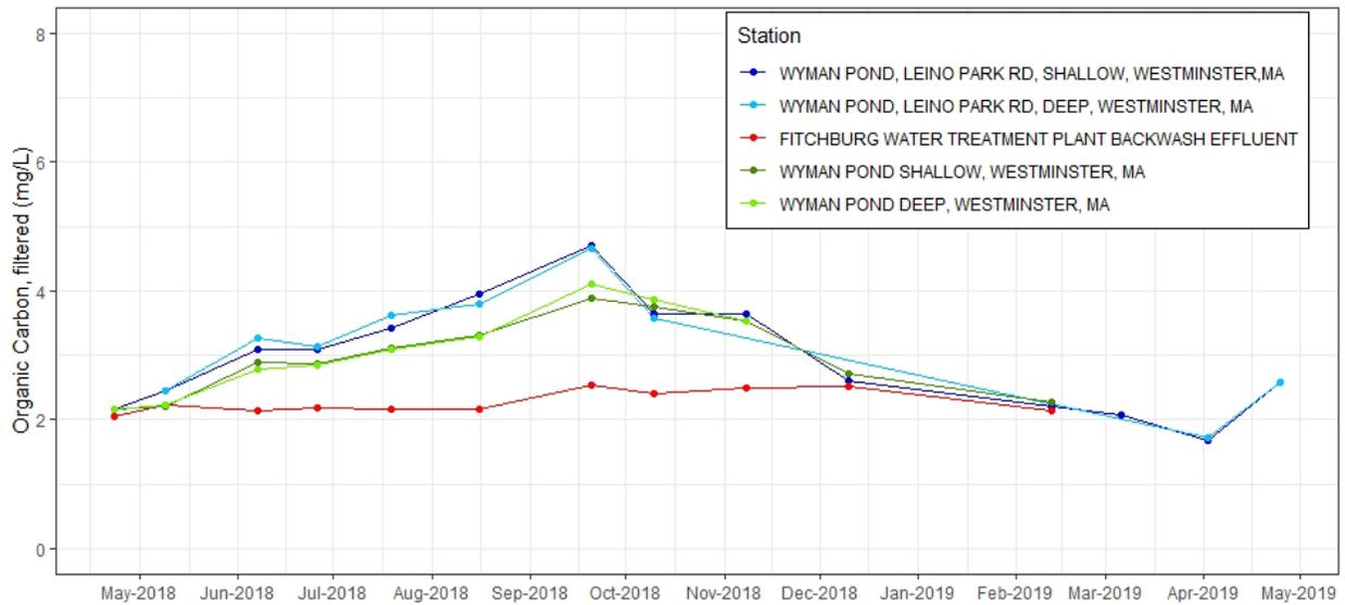
**Figure C-61.** Time series plot of organic carbon, filtered (mg/L) from discrete samples taken at effluent and ambient stations near Fitchburg WTF, 2018-2019.
