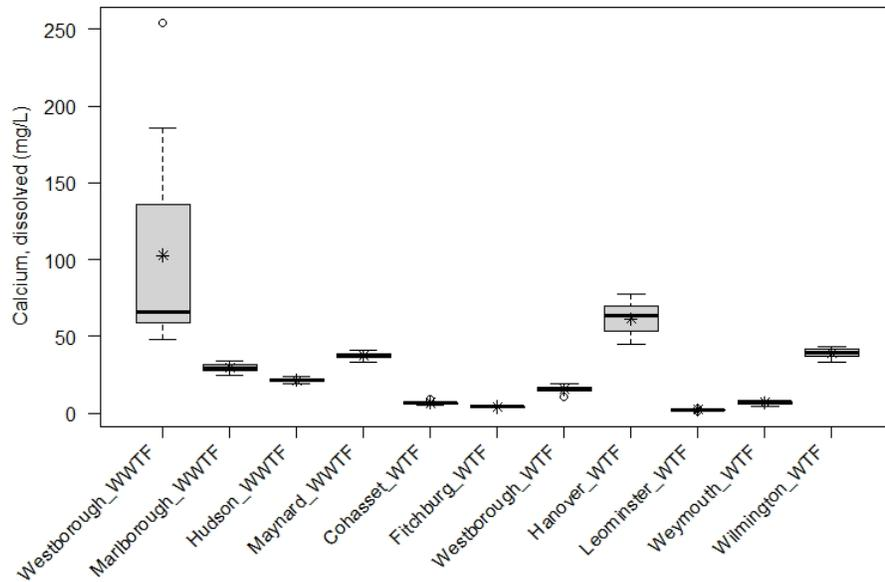
**Figure B-2.** Boxplot of calcium, filtered (mg/L), from discrete samples taken at effluent stations at 11 water or wastewater treatment facilities in eastern and central Massachusetts, 2018-2019.
