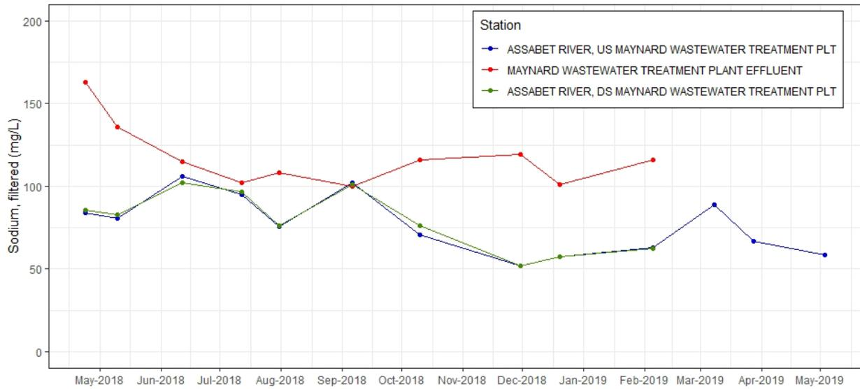
*Figure C-42. Time series plot of sodium, filtered (mg/L) from discrete samples taken at effluent and ambient stations near Maynard WWTF, 2018-2019.*
