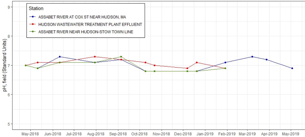
**Figure C-29.** Time series plot of pH (SU) from discrete samples taken at effluent and ambient stations near Hudson WWTF, 2018-2019.
