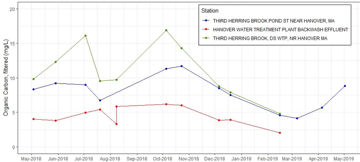
**Figure C-83.** Time series plot of organic carbon, filtered (mg/L) from discrete samples taken at effluent and ambient stations near Hanover WTF, 2018-2019. Note additional sample collected at Hanover Water Treatment Plant Backwash Effluent on August 8, 2018 is not a replicate (see Table C-1 for detail).
