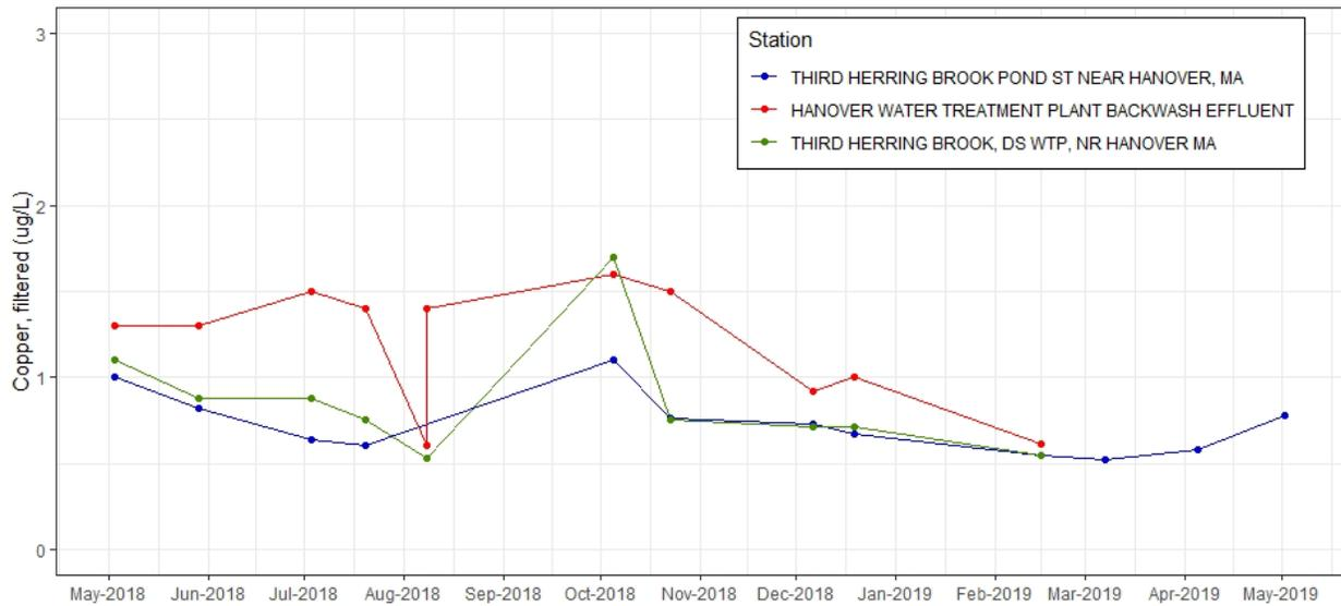
**Figure C-81.** Time series plot of copper, filtered (µg/L) from discrete samples taken at effluent and ambient stations near Hanover WTF, 2018-2019. Note additional sample collected at Hanover Water Treatment Plant Backwash Effluent on August 8, 2018 is not a replicate (see Table C-1 for detail).
