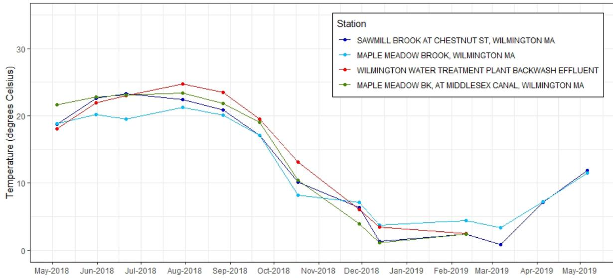
**Figure C-121.** Time series plot of water temperature (°C) from discrete samples taken at effluent and ambient stations near Wilmington WTF, 2018-2019. Note additional sample collected at Wilmington Water Treatment Plant Backwash Effluent on November 29, 2018 is not a replicate (see Table C-1 for detail).
