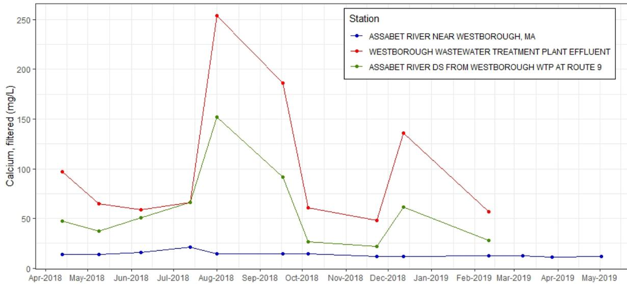
Figure C-2. Time series plot of calcium, filtered (mg/L) from discrete samples taken at effluent and ambient stations near Westborough WWTF, 2018-2019.
