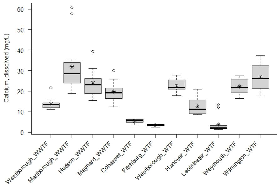
**Figure 4.** Boxplot of calcium, filtered (mg/L), from discrete samples taken at selected ambient stations (upstream or pond) at 11 water or wastewater treatment facilities in eastern and central Massachusetts, 2018-2019. Data include only those from selected ambient stations used for copper criteria value calculations in the Biotic Ligand Model (BLM).
