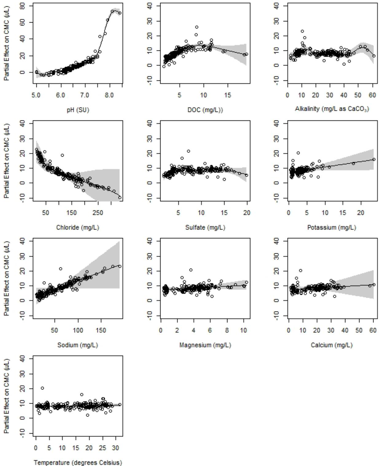
Figure 15. Smooth partial effects plots for the Generalized Additive Model (GAM) for acute (criterion maximum concentration, CMC) values as a function of each input parameter to the Biotic Ligand Model (BLM). The y-axis is the smooth or spline function partial effect in response to the respective BLM input parameter. Shaded area indicates the 95% confidence interval for the mean shape of the effect.
