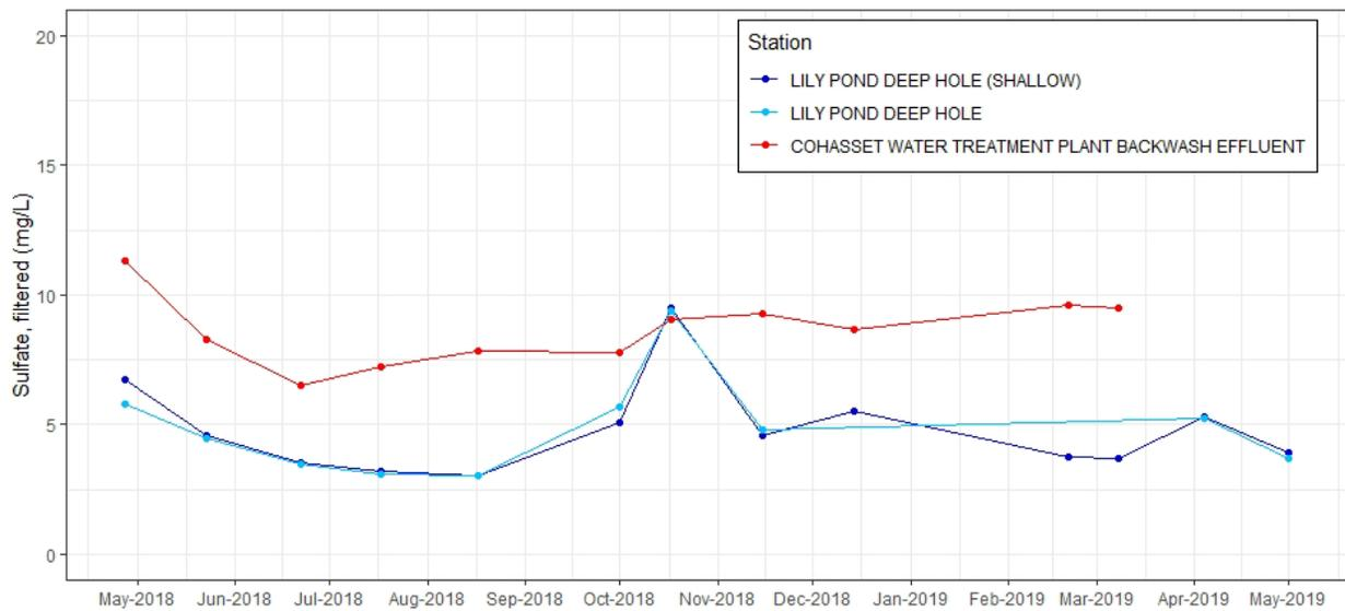
**Figure C-54.** Time series plot of sulfate, filtered (mg/L) from discrete samples taken at effluent and ambient stations near Cohasset WTF, 2018-2019.
