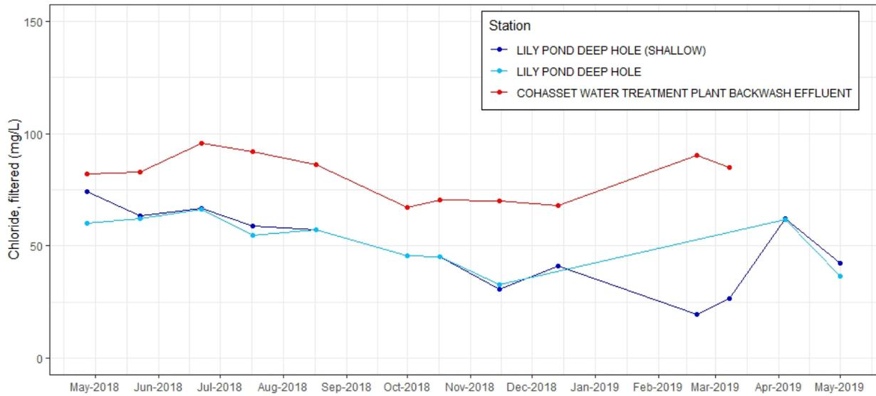
**Figure C-47.** Time series plot of chloride, filtered (mg/L) from discrete samples taken at effluent and ambient stations near Cohasset WTF, 2018-2019.
