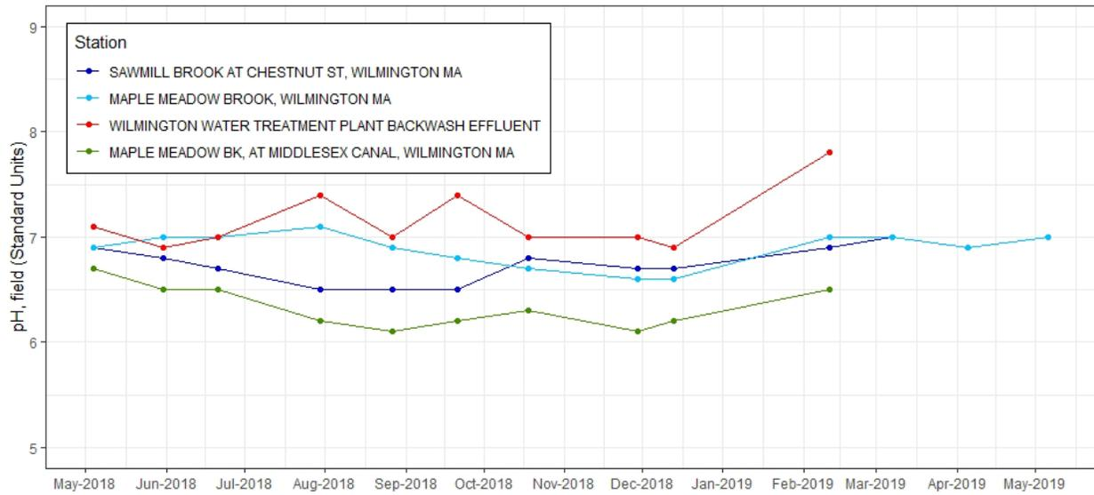
**Figure C-117.** Time series plot of pH (SU) from discrete samples taken at effluent and ambient stations near Wilmington WTF, 2018-2019. Note additional sample collected at Wilmington Water Treatment Plant Backwash Effluent on November 29, 2018 is not a replicate (see Table C-1 for detail).
