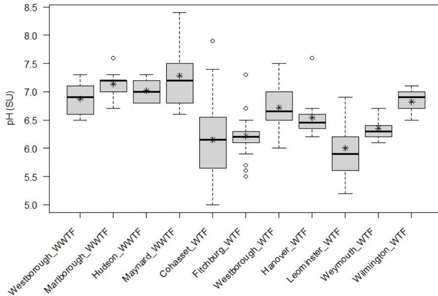
**Figure 9.** Boxplot of pH (standard units; SU) from discrete samples taken at selected ambient stations (upstream or pond) at 11 water or wastewater treatment facilities in eastern and central Massachusetts, 2018-2019. Data include only those from selected ambient stations used for copper criteria value calculations in the Biotic Ligand Model (BLM).
