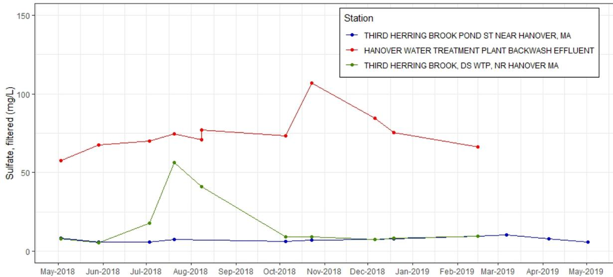
**Figure C-87.** Time series plot of sulfate, filtered (mg/L) from discrete samples taken at effluent and ambient stations near Hanover WTF, 2018-2019. Note additional sample collected at Hanover Water Treatment Plant Backwash Effluent on August 8, 2018 is not a replicate (see Table C-1 for detail).
