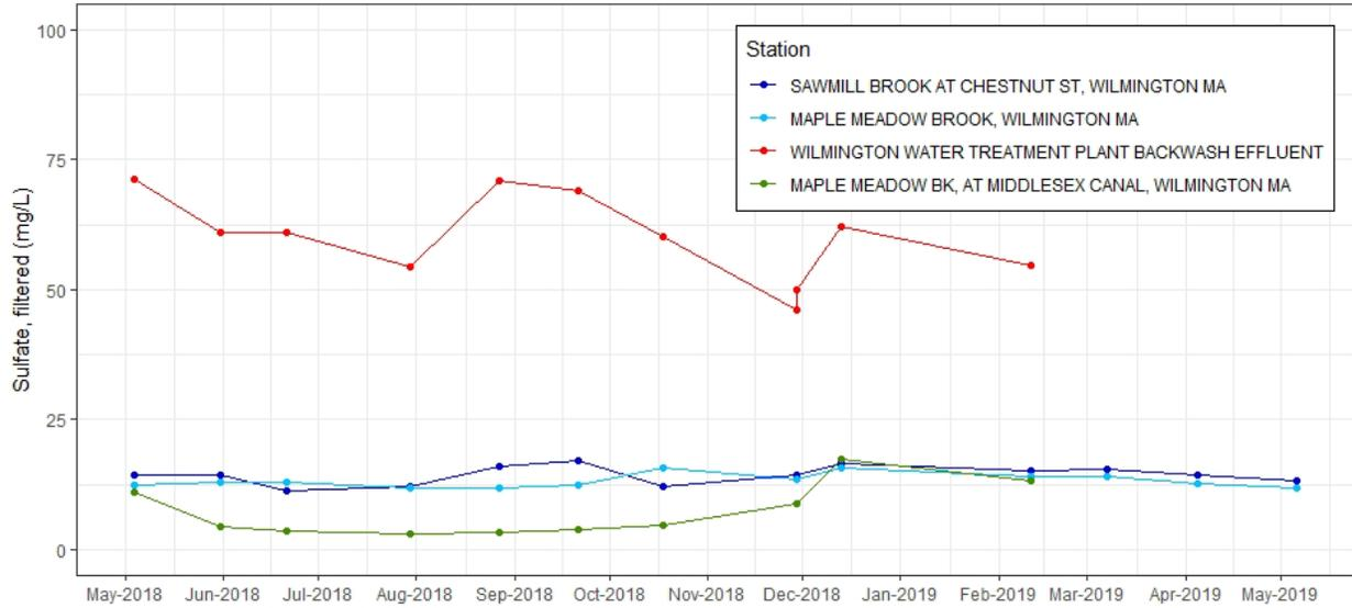
**Figure C-120.** Time series plot of Sulfate, filtered (mg/L) from discrete samples taken at effluent and ambient stations near Wilmington WTF, 2018-2019. Note additional sample collected at Wilmington Water Treatment Plant Backwash Effluent on November 29, 2018 is not a replicate (see Table C-1 for detail).
