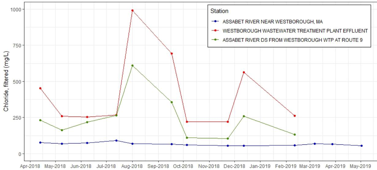
**Figure C-3.** Time series plot of chloride, filtered (mg/L) from discrete samples taken at effluent and ambient stations near Westborough WWTF, 2018-2019.
