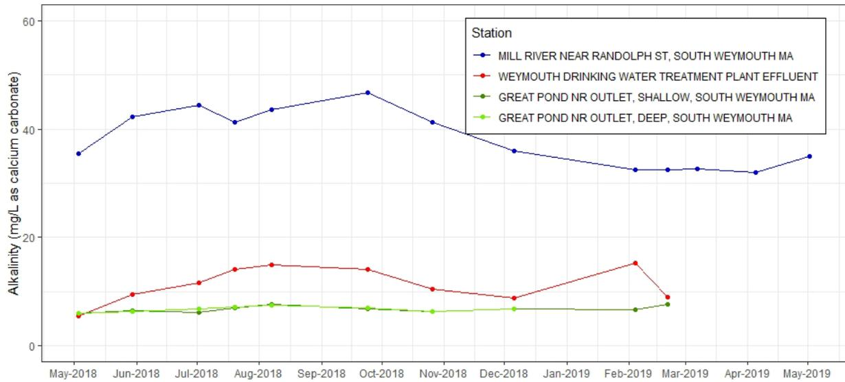
**Figure C-100.** Time series plot of Alkalinity, filtered (mg/L as calcium carbonate) from discrete samples taken at effluent and ambient stations near Weymouth WTF, 2018-2019.
