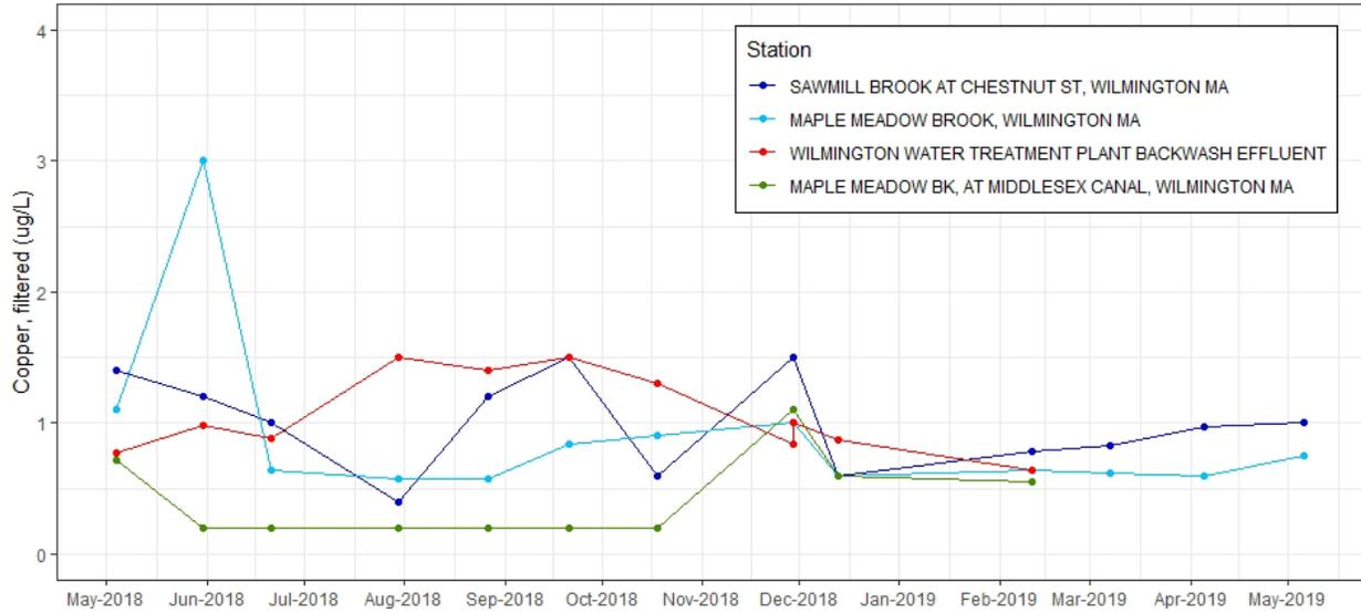
**Figure C-114.** Time series plot of Copper, filtered (µg/L) from discrete samples taken at effluent and ambient stations near Wilmington WTF, 2018-2019. Note additional sample collected at Wilmington Water Treatment Plant Backwash Effluent on November 29, 2018 is not a replicate (see Table C-1 for detail).
