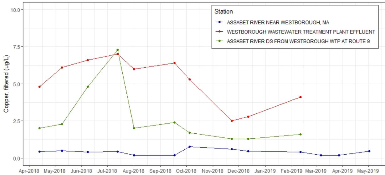
**Figure C-4.** Time series plot of copper, filtered (µg/L) from discrete samples taken at effluent and ambient stations near Westborough WWTF, 2018-2019.
