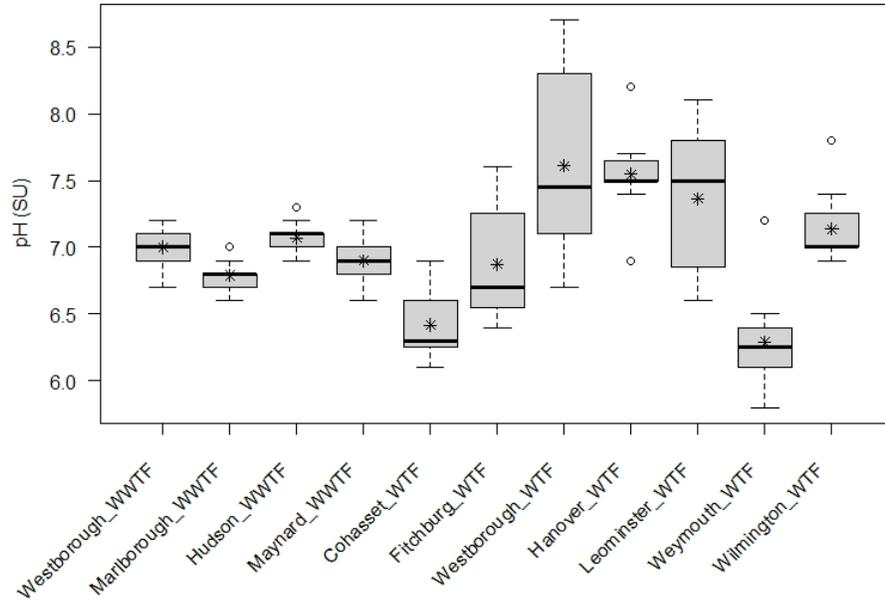
**Figure B-7.** Boxplot of pH (SU) from discrete samples taken at effluent stations at 11 water or wastewater treatment facilities in eastern and central Massachusetts, 2018-2019.
