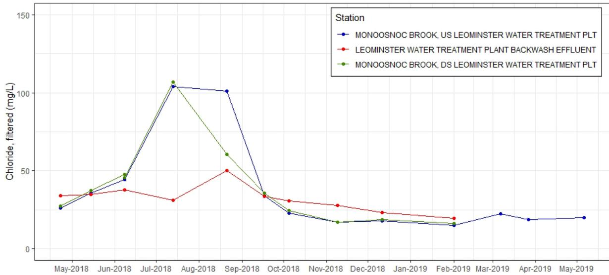
**Figure C-91.** Time series plot of chloride, filtered (mg/L) from discrete samples taken at effluent and ambient stations near Leominster WTF, 2018-2019. Note additional samples collected at Leominster Water Treatment Plant Backwash Effluent and Monoosnoc Brook, DS Leominster Water Treatment Plt on June 8, 2018 are not replicates (see Table C-1 for detail).
