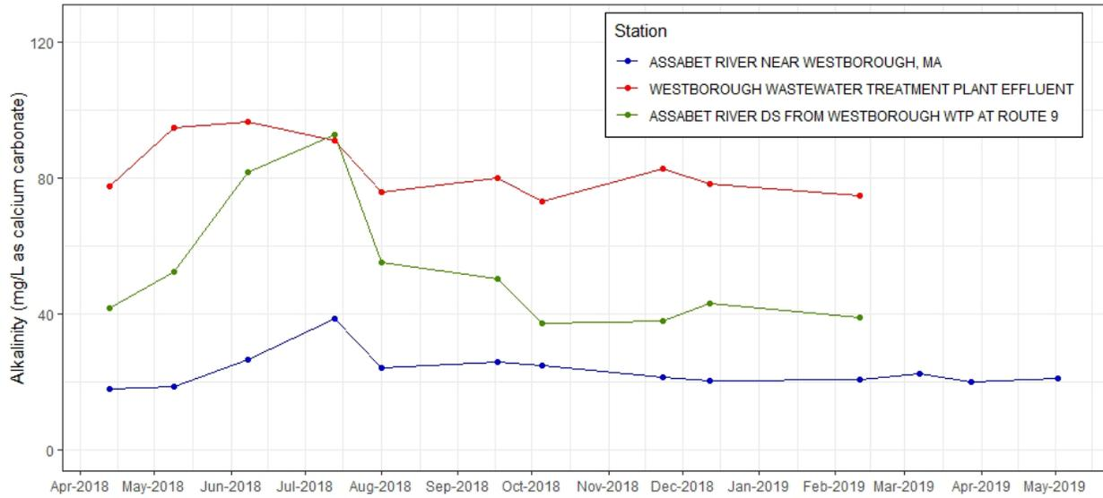
Figure C-1. Time series plot of alkalinity, filtered (mg/L as calcium carbonate) from discrete samples taken at effluent and ambient stations near Westborough WWTF, 2018-2019.
