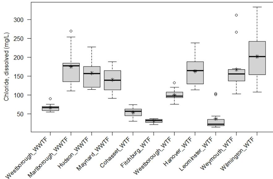
**Figure 5.** Boxplot of chloride, filtered (mg/L), from discrete samples taken at selected ambient stations (upstream or pond) at 11 water or wastewater treatment facilities in eastern and central Massachusetts, 2018-2019. Data include only those from selected ambient stations used for copper criteria value calculations in the Biotic Ligand Model (BLM).
