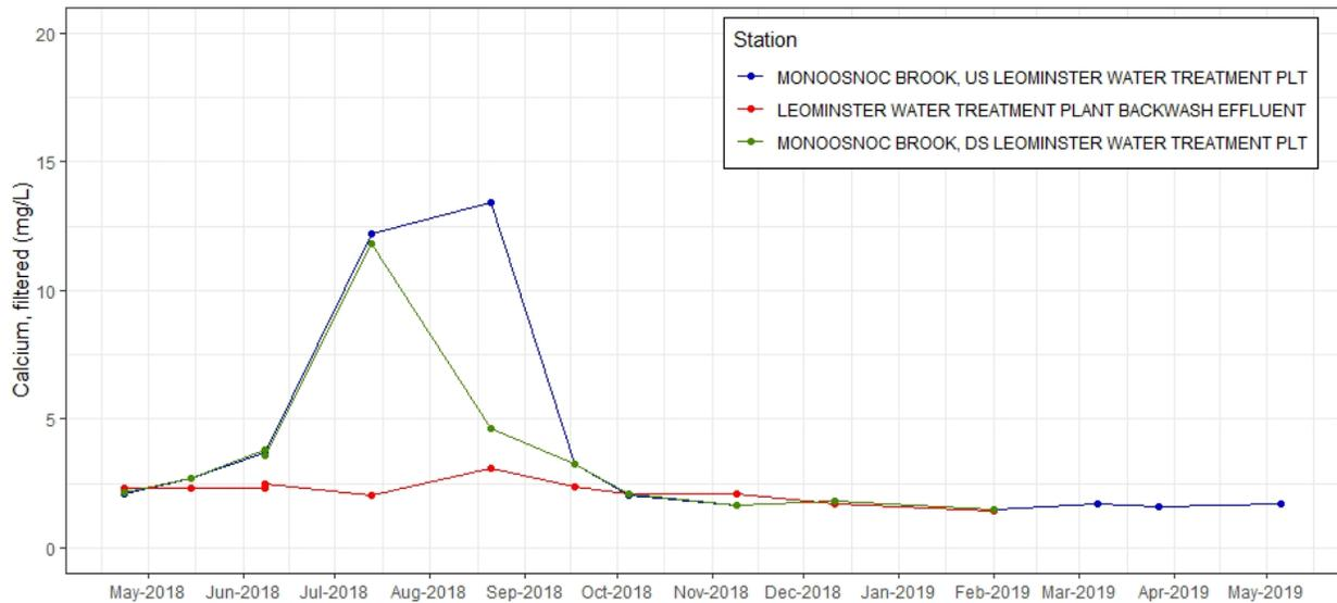
**Figure C-90.** Time series plot of calcium, filtered (mg/L) from discrete samples taken at effluent and ambient stations near Leominster WTF, 2018-2019. Note additional samples collected at Leominster Water Treatment Plant Backwash Effluent and Monoosnoc Brook, DS Leominster Water Treatment Plt on June 8, 2018 are not replicates (see Table C-1 for detail).
