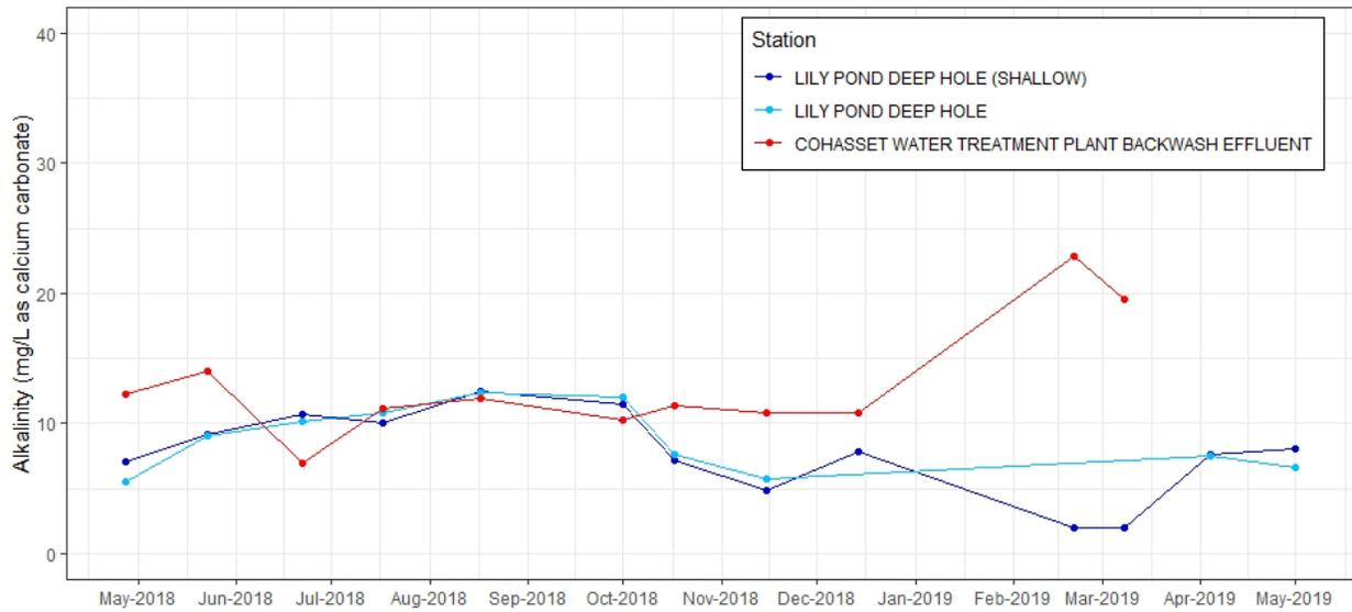
**Figure C-45.** Time series plot of alkalinity, filtered (mg/L as calcium carbonate) from discrete samples taken at effluent and ambient stations near Cohasset WTF, 2018-2019.
