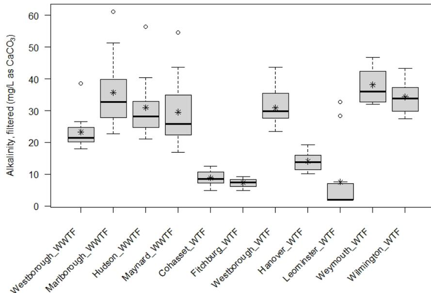
**Figure 3.** Boxplot of alkalinity, filtered (mg/L as calcium carbonate), from discrete samples taken at selected ambient stations (upstream or pond) at 11 water or wastewater treatment facilities in eastern and central Massachusetts, 2018-2019. Data include only those from selected ambient stations used for copper criteria value calculations in the Biotic Ligand Model (BLM).
