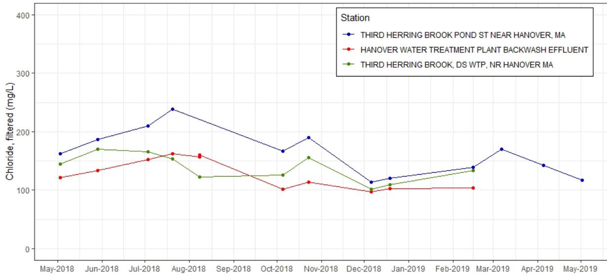
**Figure C-80.** Time series plot of chloride, filtered (mg/L) from discrete samples taken at effluent and ambient stations near Hanover WTF, 2018-2019. Note additional sample collected at Hanover Water Treatment Plant Backwash Effluent on August 8, 2018 is not a replicate (see Table C-1 for detail).
