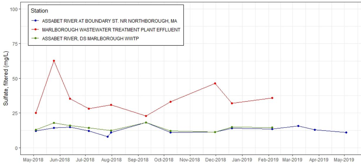
**Figure C-21.** Time series plot of Sulfate, filtered (mg/L) from discrete samples taken at effluent and ambient stations near Marlborough WWTF, 2018-2019. Note additional sample collected at Assabet River at Boundary St. near Northborough, MA on July 27, 2018 is not a replicate (see Table C-1 for detail).
