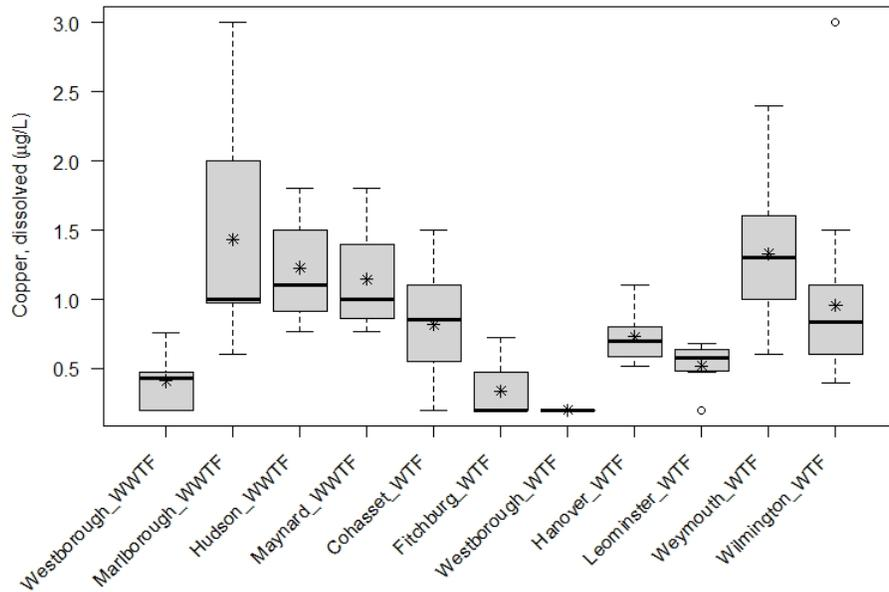
**Figure 6.** Boxplot of copper, filtered ( $\mu\text{g/L}$ ), from discrete samples taken at selected ambient stations (upstream or pond) at 11 water or wastewater treatment facilities in eastern and central Massachusetts, 2018-2019. Data include only those from selected ambient stations used for copper criteria value calculations in the Biotic Ligand Model (BLM).
