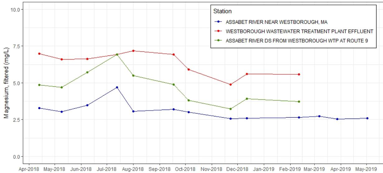
**Figure C-5.** Time series plot of magnesium, filtered (mg/L) from discrete samples taken at effluent and ambient stations near Westborough WWTF, 2018-2019.
