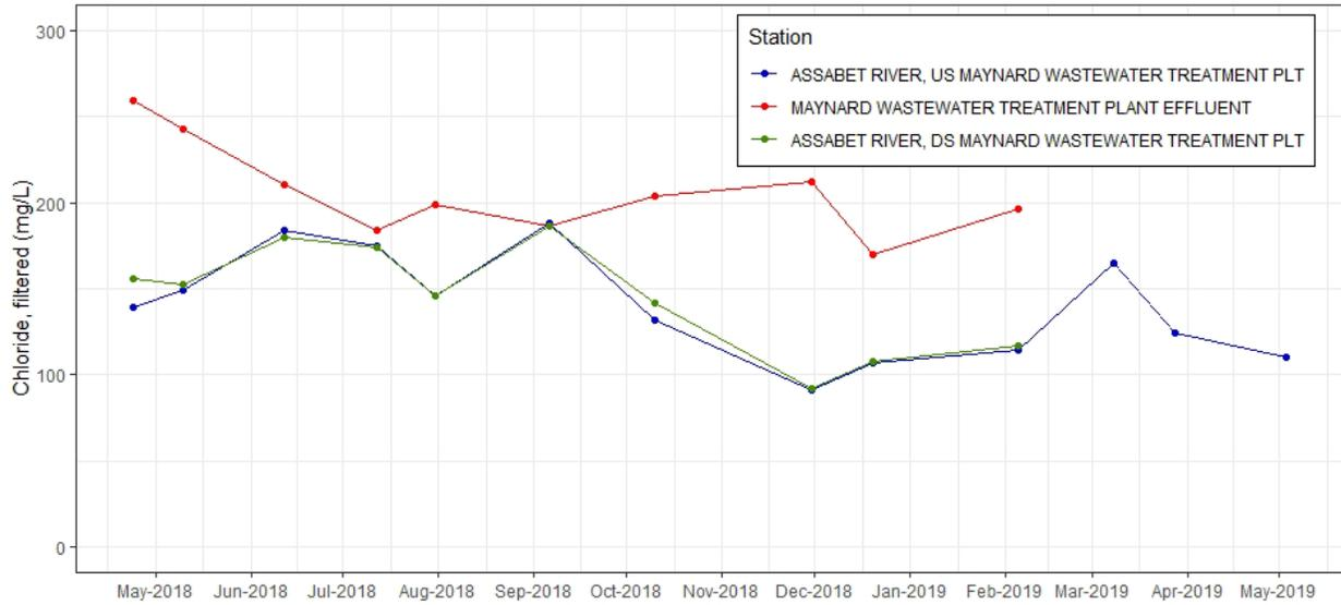
*Figure C-36. Time series plot of chloride, filtered (mg/L) from discrete samples taken at effluent and ambient stations near Maynard WWTF, 2018-2019.*
