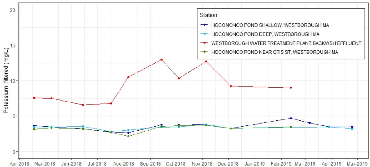
**Figure C-74.** Time series plot of potassium, filtered (mg/L) from discrete samples taken at effluent and ambient stations near Westborough WTF, 2018-2019.
