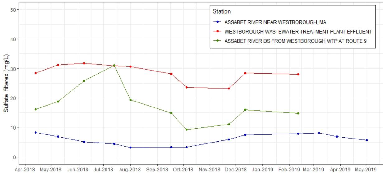
**Figure C-10.** Time series plot of sulfate, filtered (mg/L) from discrete samples taken at effluent and ambient stations near Westborough WWTF, 2018-2019.
