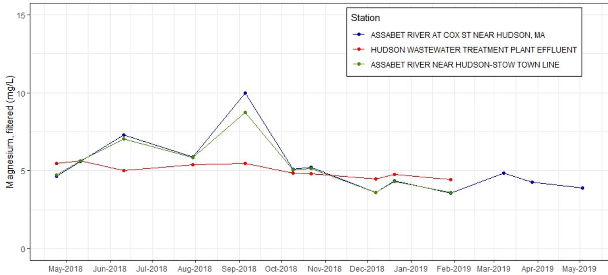
**Figure C-27.** Time series plot of magnesium, filtered (mg/L) from discrete samples taken at effluent and ambient stations near Hudson WWTF, 2018-2019.
