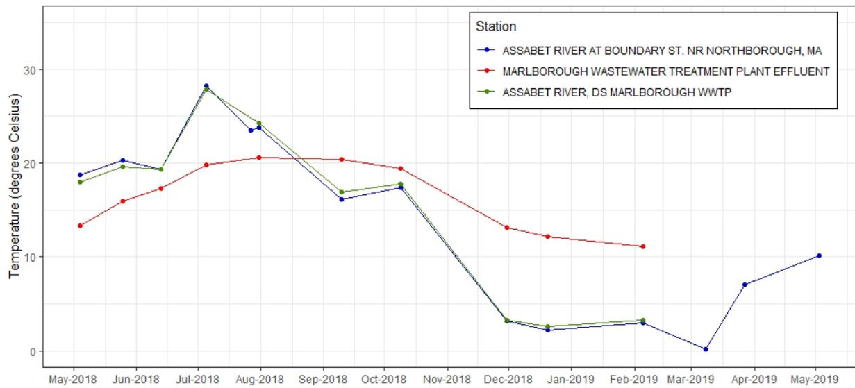
**Figure C-22.** Time series plot of water temperature (°C) from discrete samples taken at effluent and ambient stations near Marlborough WWTF, 2018-2019. Note additional sample collected at Assabet River at Boundary St. near Northborough, MA on July 27, 2018 is not a replicate (see Table C-1 for detail).
