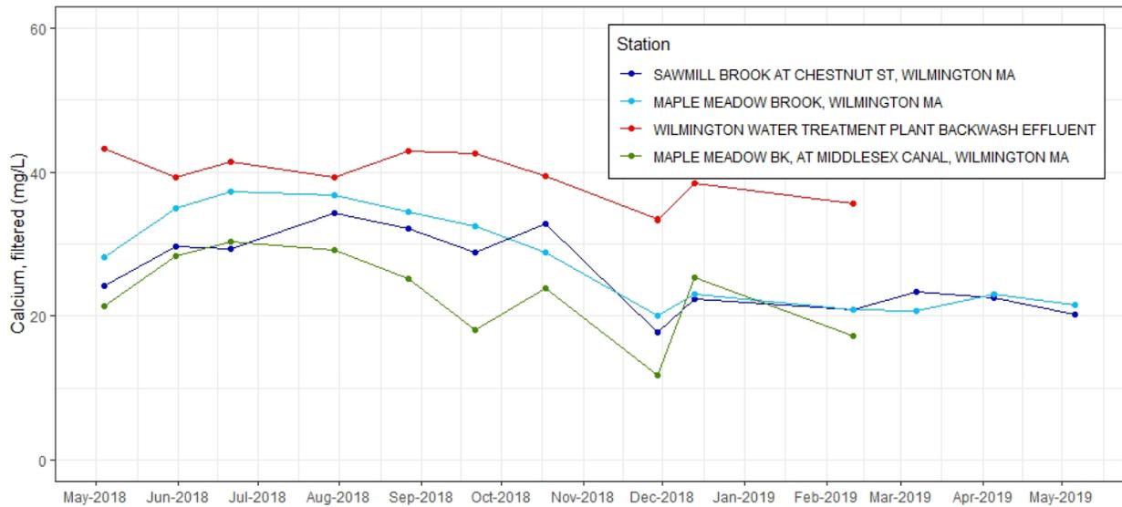
**Figure C-112.** Time series plot of Calcium, filtered (mg/L) from discrete samples taken at effluent and ambient stations near Wilmington WTF, 2018-2019. Note additional sample collected at Wilmington Water Treatment Plant Backwash Effluent on November 29, 2018 is not a replicate (see Table C-1 for detail).
