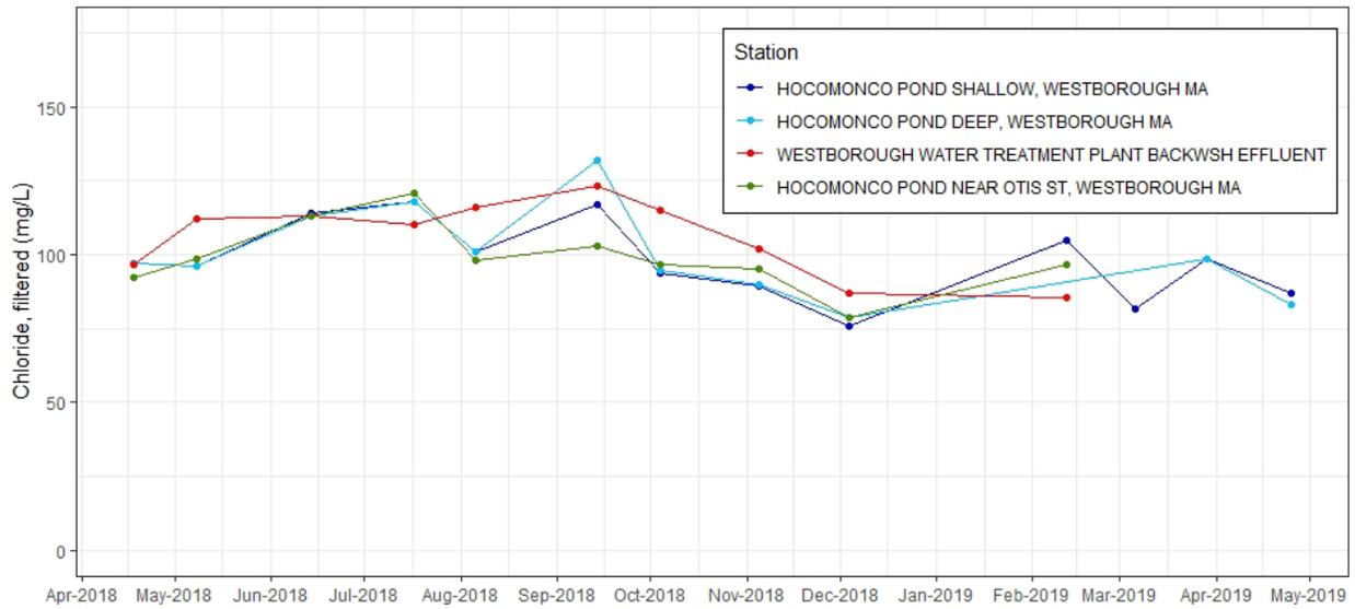
**Figure C-69.** Time series plot of chloride, filtered (mg/L) from discrete samples taken at effluent and ambient stations near Westborough WTF, 2018-2019.
