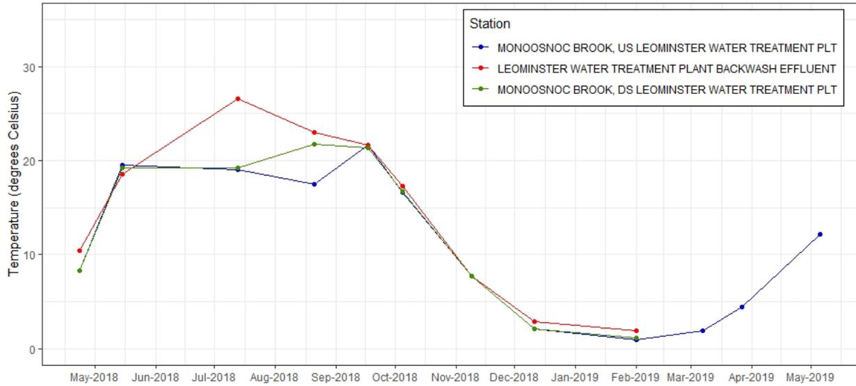
**Figure C-99.** Time series plot of water temperature (°C) from discrete samples taken at effluent and ambient stations near Leominster WTF, 2018-2019. Note additional samples collected at Leominster Water Treatment Plant Backwash Effluent and Monoosnoc Brook, DS Leominster Water Treatment Plt on June 8, 2018 are not replicates (see Table C-1 for detail).
