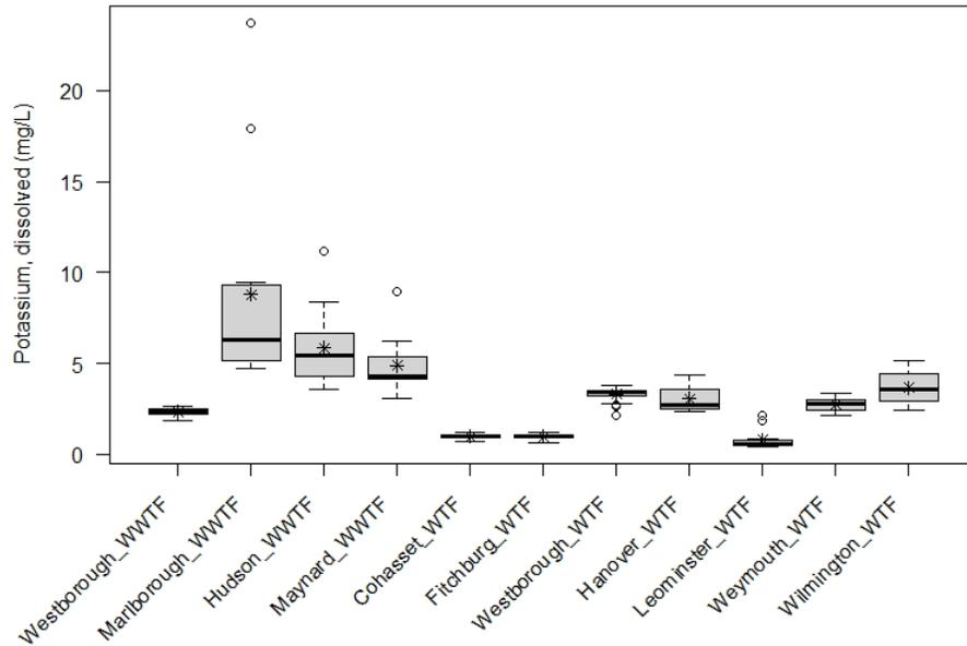
**Figure 10.** Boxplot of potassium, filtered (mg/L), from discrete samples taken at selected ambient stations (upstream or pond) at 11 water or wastewater treatment facilities in eastern and central Massachusetts, 2018-2019. Data include only those from selected ambient stations used for copper criteria value calculations in the Biotic Ligand Model (BLM).
