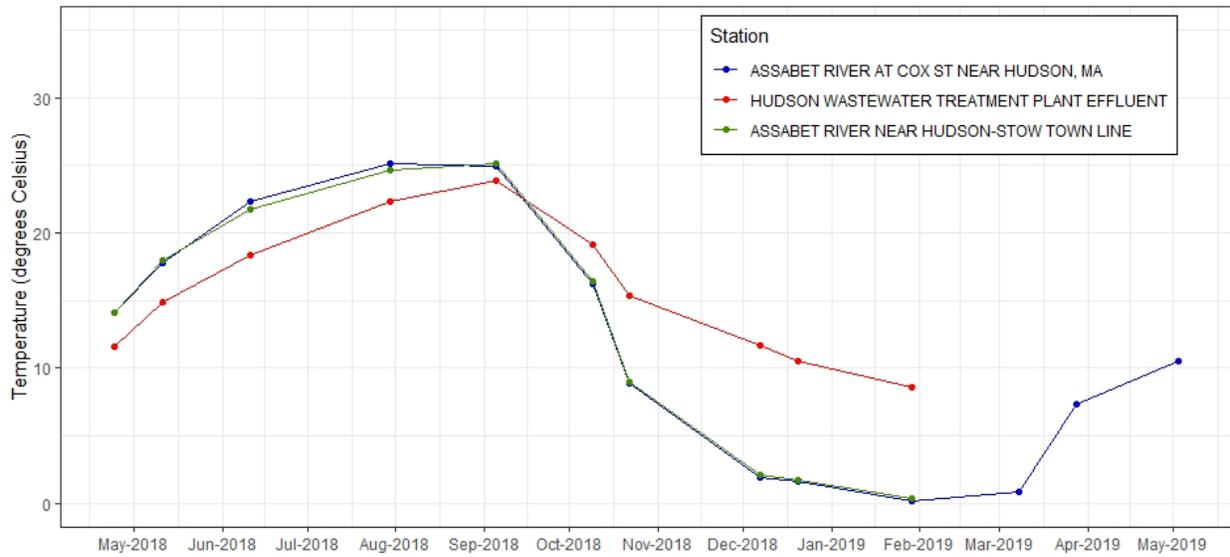
**Figure C-33.** Time series plot of water temperature (°C) from discrete samples taken at effluent and ambient stations near Hudson WWTF, 2018-2019.
