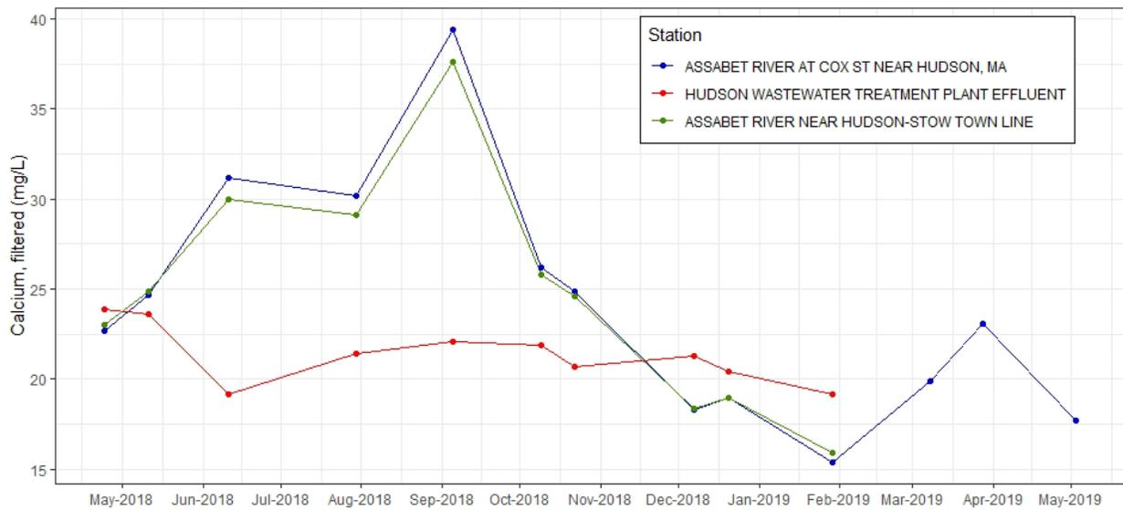
**Figure C-24.** Time series plot of calcium, filtered (mg/L) from discrete samples taken at effluent and ambient stations near Hudson WWTF, 2018-2019.
