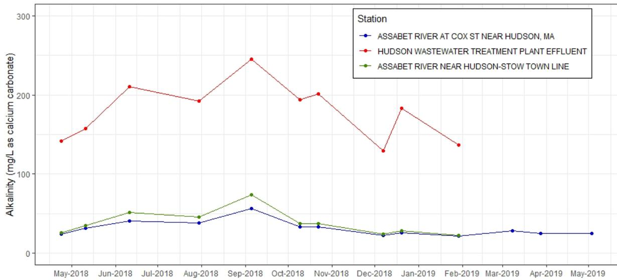
**Figure C-23.** Time series plot of alkalinity, filtered (mg/L as calcium carbonate) from discrete samples taken at effluent and ambient stations near Hudson WWTF, 2018-2019.
