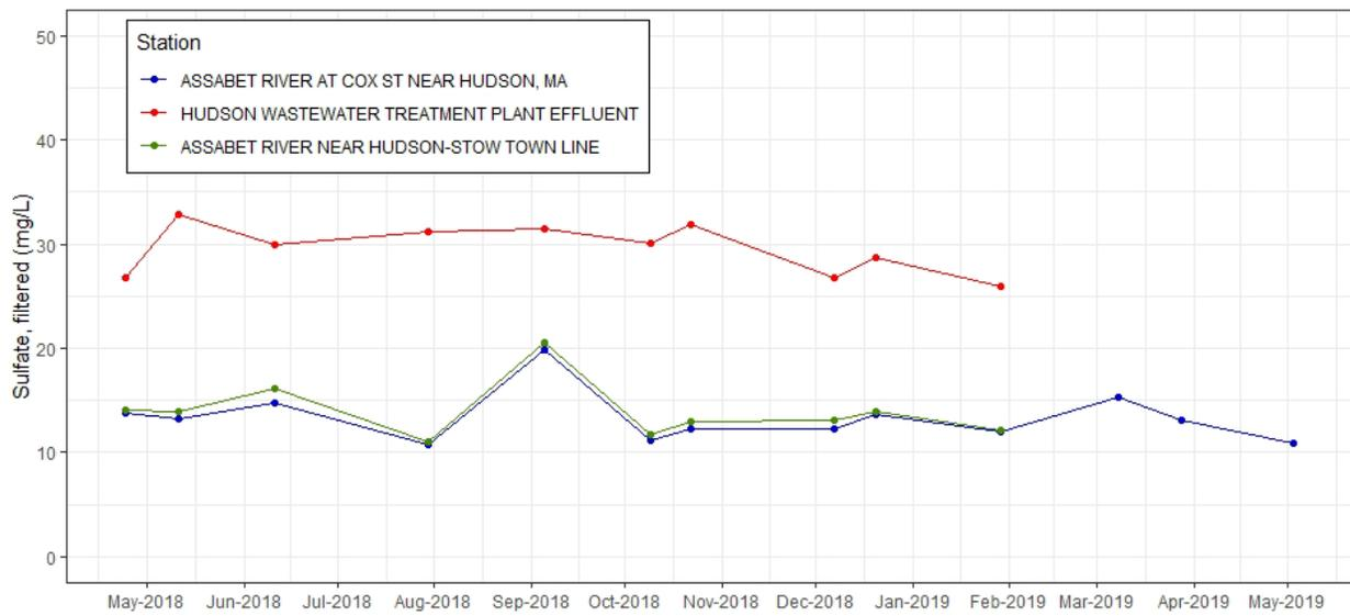
**Figure C-32.** Time series plot of sulfate, filtered (mg/L) from discrete samples taken at effluent and ambient stations near Hudson WWTF, 2018-2019.
