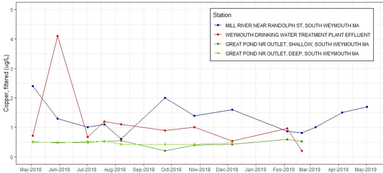
**Figure C-103.** Time series plot of Copper, filtered (µg/L) from discrete samples taken at effluent and ambient stations near Weymouth WTF, 2018-2019.
