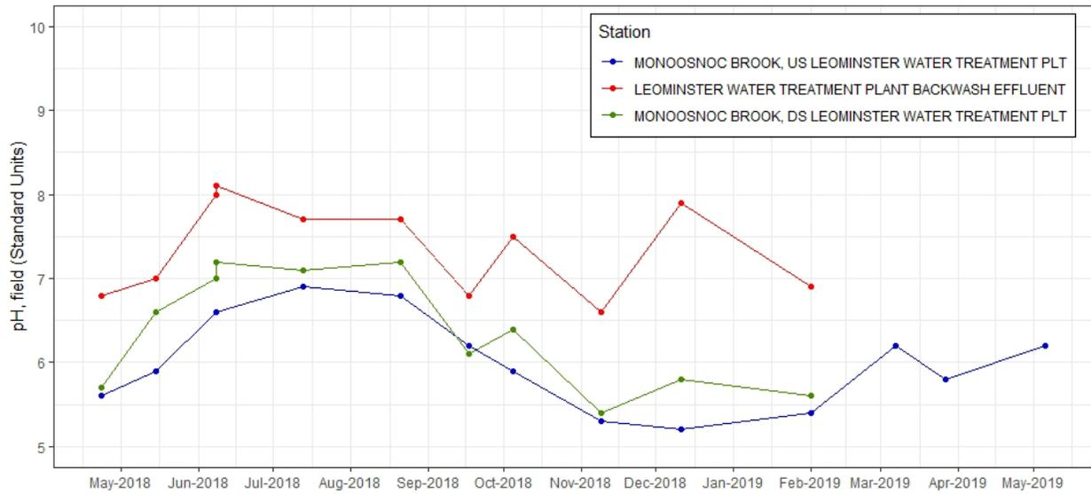
**Figure C-95.** Time series plot of pH (SU) from discrete samples taken at effluent and ambient stations near Leominster WTF, 2018-2019. Note additional samples collected at Leominster Water Treatment Plant Backwash Effluent and Monoosnoc Brook, DS Leominster Water Treatment Plt on June 8, 2018 are not replicates (see Table C-1 for detail).
