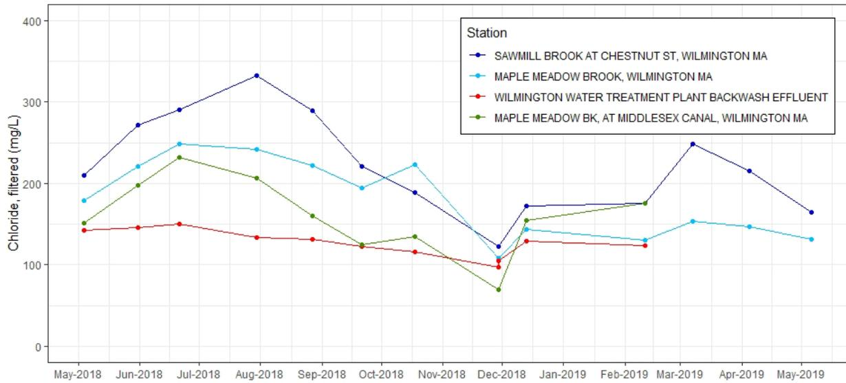
**Figure C-113.** Time series plot of Chloride, filtered (mg/L) from discrete samples taken at effluent and ambient stations near Wilmington WTF, 2018-2019. Note additional sample collected at Wilmington Water Treatment Plant Backwash Effluent on November 29, 2018 is not a replicate (see Table C-1 for detail).
