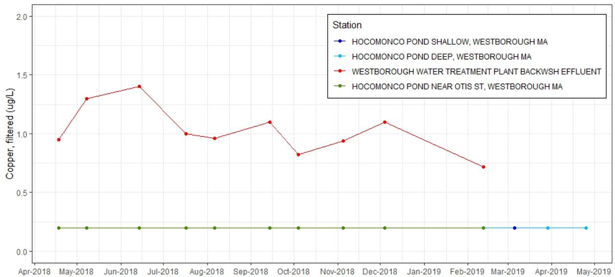
**Figure C-70.** Time series plot of copper, filtered (µg/L) from discrete samples taken at effluent and ambient stations near Westborough WTF, 2018-2019.
