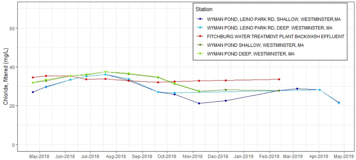
**Figure C-58.** Time series plot of chloride, filtered (mg/L) from discrete samples taken at effluent and ambient stations near Fitchburg WTF, 2018-2019.
