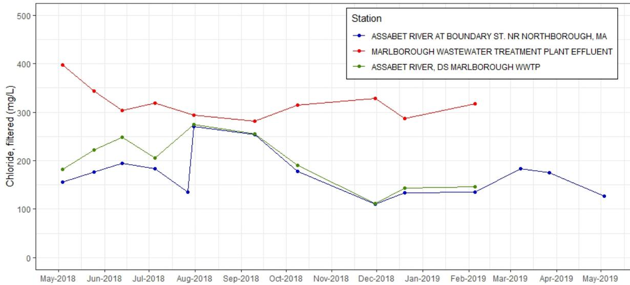
**Figure C-14.** Time series plot of chloride, filtered (mg/L) from discrete samples taken at effluent and ambient stations near Marlborough WWTF, 2018-2019. Note additional sample collected at Assabet River at Boundary St. near Northborough, MA on July 27, 2018 is not a replicate (see Table C-1 for detail).
