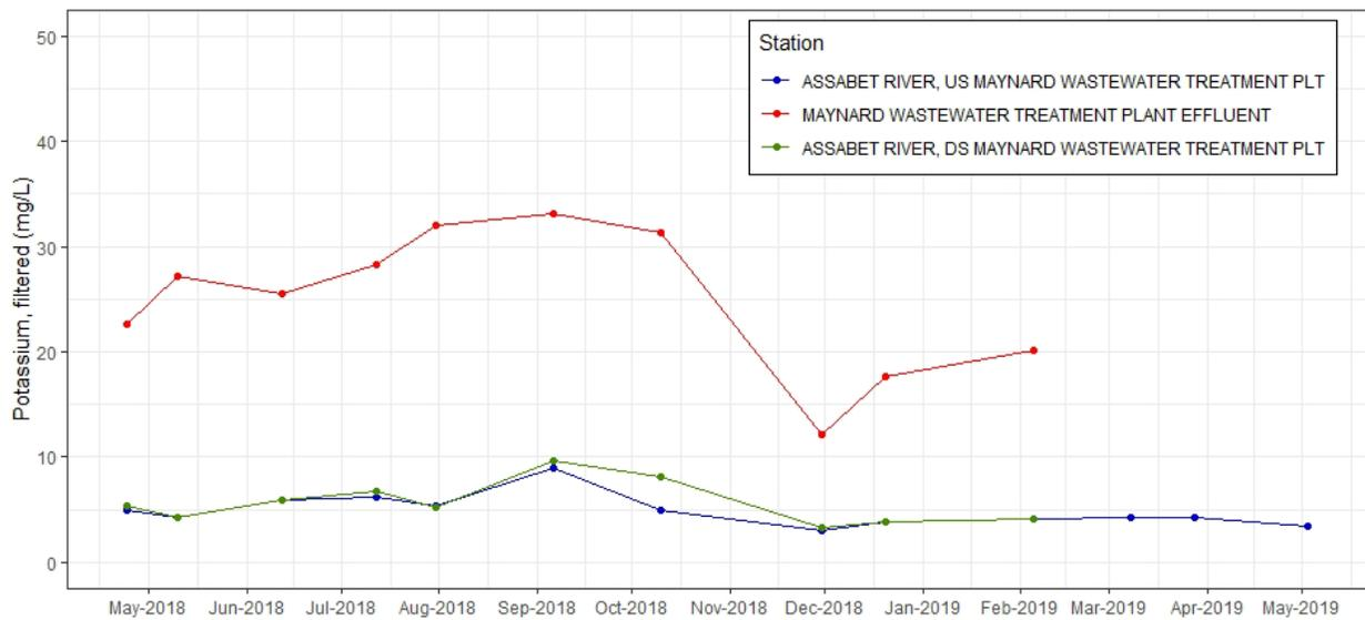
**Figure C-41.** Time series plot of potassium, filtered (mg/L) from discrete samples taken at effluent and ambient stations near Maynard WWTF, 2018-2019.
