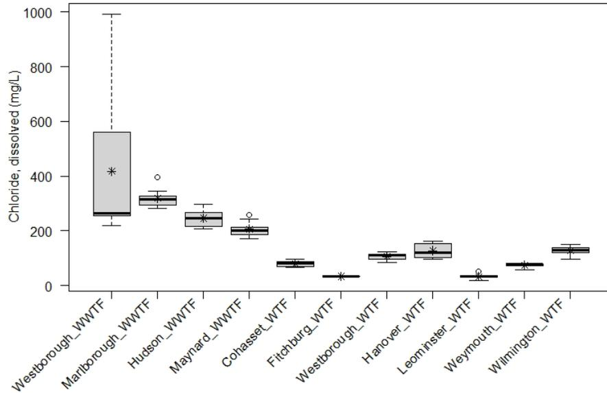
**Figure B-3.** Boxplot of chloride, filtered (mg/L), from discrete samples taken at effluent stations at 11 water or wastewater treatment facilities in eastern and central Massachusetts, 2018-2019.
