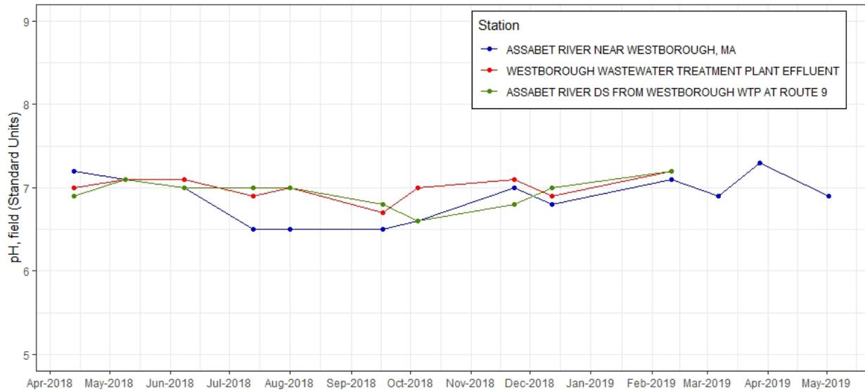
**Figure C-7.** Time series plot of pH (SU) from discrete samples taken at effluent and ambient stations near Westborough WWTF, 2018-2019.
