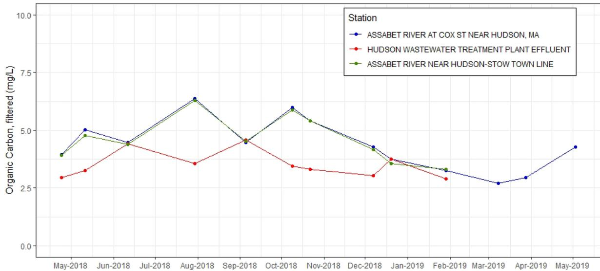
**Figure C-28.** Time series plot of organic carbon, filtered (mg/L) from discrete samples taken at effluent and ambient stations near Hudson WWTF, 2018-2019.
