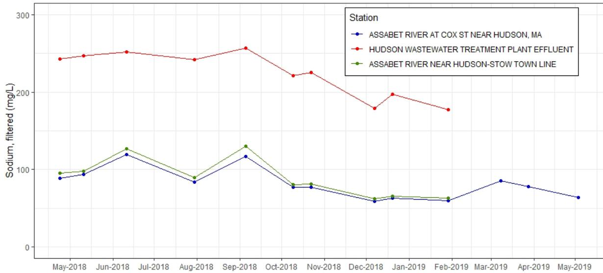
**Figure C-31.** Time series plot of sodium, filtered (mg/L) from discrete samples taken at effluent and ambient stations near Hudson WWTF, 2018-2019.
