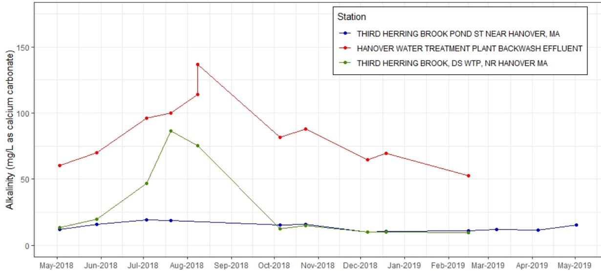
**Figure C-78.** Time series plot of alkalinity, filtered (mg/L as calcium carbonate) from discrete samples taken at effluent and ambient stations near Hanover WTF, 2018-2019. Note additional sample collected at Hanover Water Treatment Plant Backwash Effluent on August 8, 2018 is not a replicate (see Table C-1 for detail).
