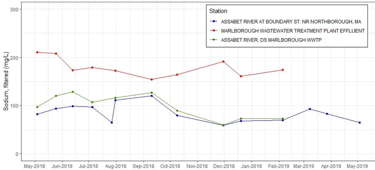
**Figure C-20.** Time series plot of Sodium, filtered (mg/L) from discrete samples taken at effluent and ambient stations near Marlborough WWTF, 2018-2019. Note additional sample collected at Assabet River at Boundary St. near Northborough, MA on July 27, 2018 is not a replicate (see Table C-1 for detail).
