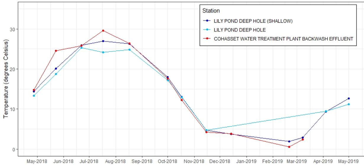
**Figure C-55.** Time series plot of water temperature (°C) from discrete samples taken at effluent and ambient stations near Cohasset WTF, 2018-2019.
