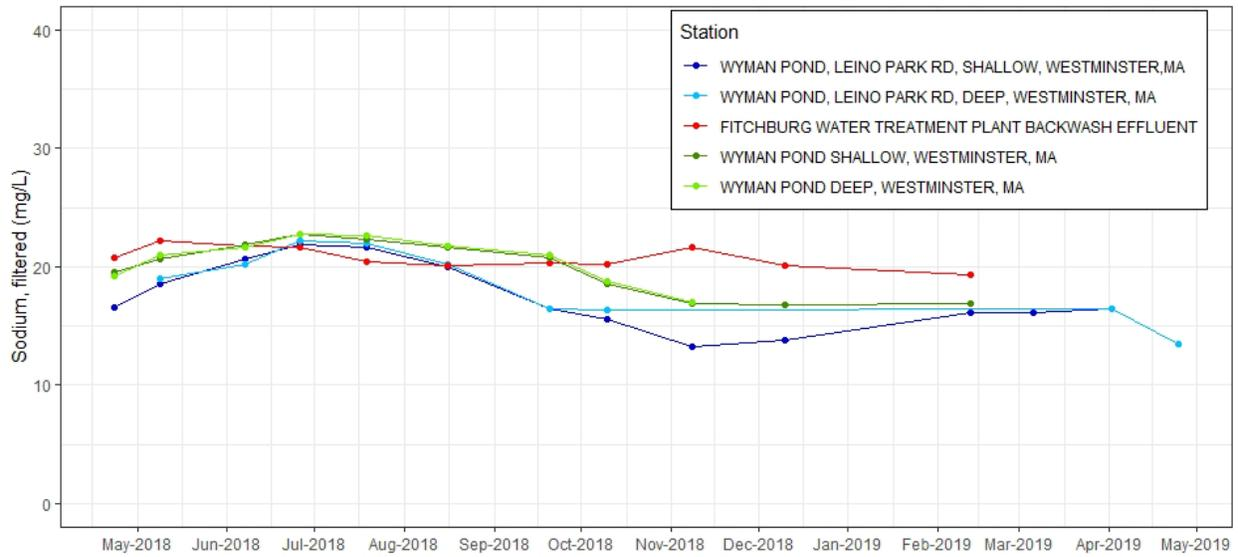
**Figure C-64.** Time series plot of sodium, filtered (mg/L) from discrete samples taken at effluent and ambient stations near Fitchburg WTF, 2018-2019.
