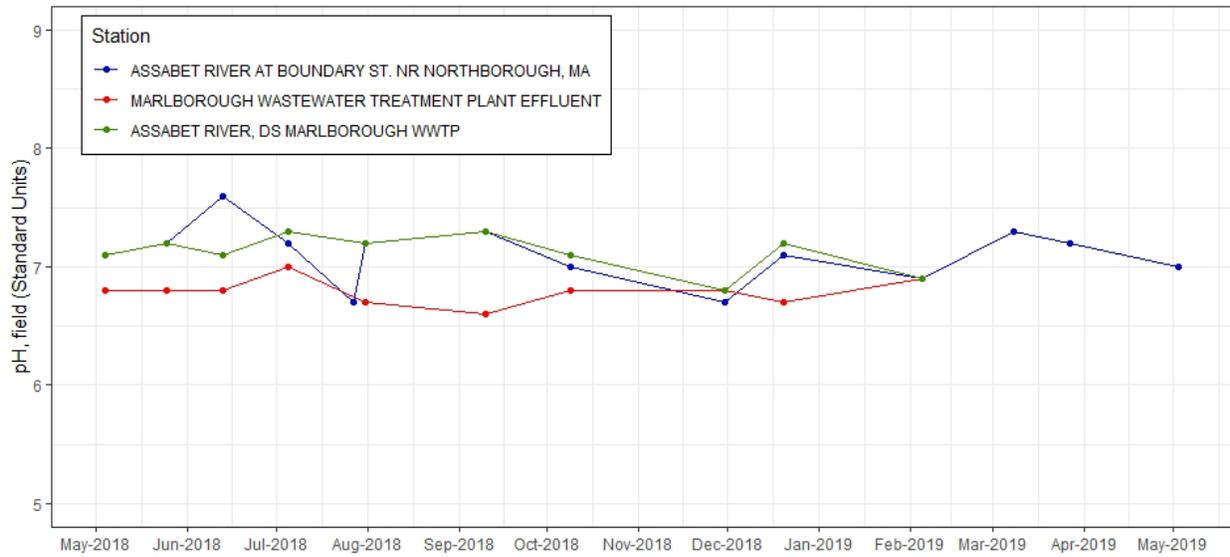
**Figure C-18.** Time series plot of pH (SU) from discrete samples taken at effluent and ambient stations near Marlborough WWTF, 2018-2019. Note additional sample collected at Assabet River at Boundary St. near Northborough, MA on July 27, 2018 is not a replicate (see Table C-1 for detail).
