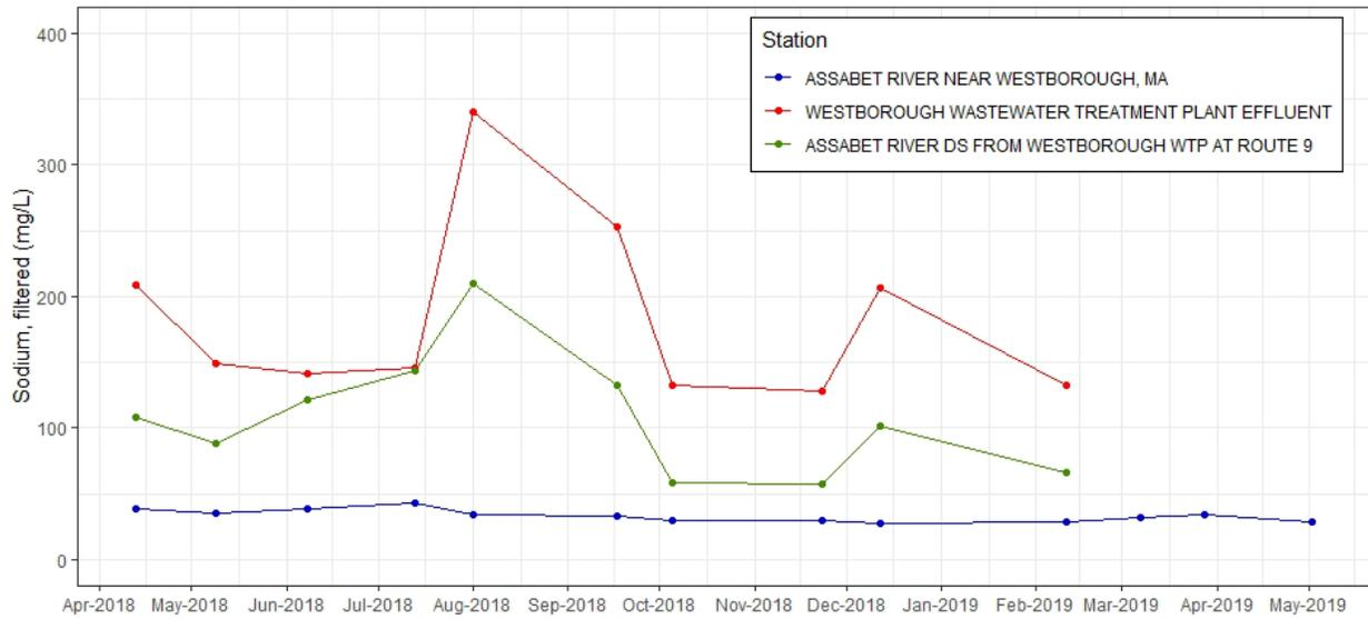
**Figure C-9.** Time series plot of sodium, filtered (mg/L) from discrete samples taken at effluent and ambient stations near Westborough WWTF, 2018-2019.
