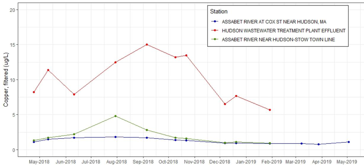
*Figure C-26. Time series plot of copper, filtered (µg/L) from discrete samples taken at effluent and ambient stations near Hudson WWTF, 2018-2019.*
