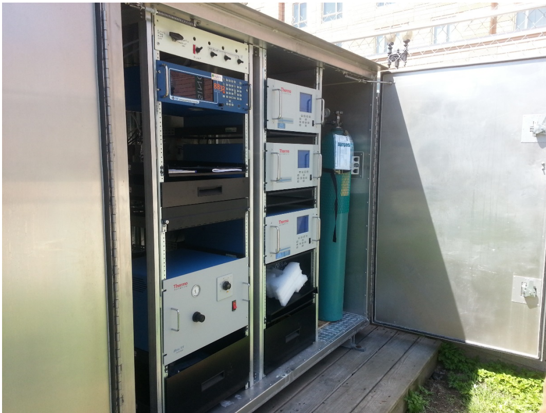
FIGURE 3-4: CO-NO-NO 2 DST MONITORS ENCLOSURE
