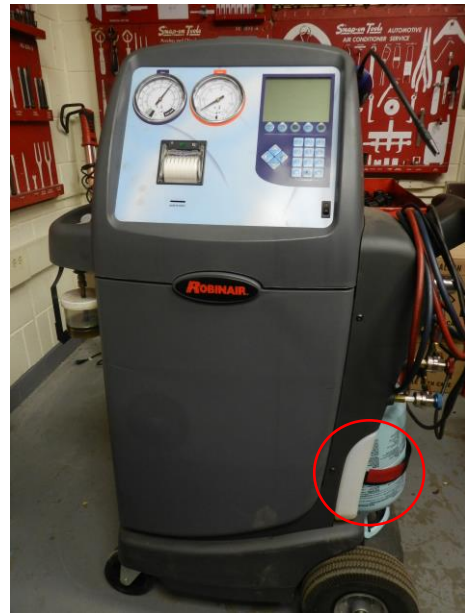
The front of a refrigerant recovery and recharging system (the circled refrigerant tank can be seen more completely below)
