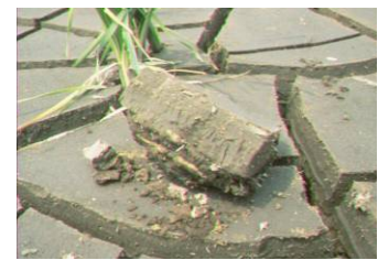
Hydraulically dredged sediment after drying
