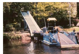
Mechanized harvester with offloading conveyor (provided by J. Dauffenbach, Aquarius Systems)
