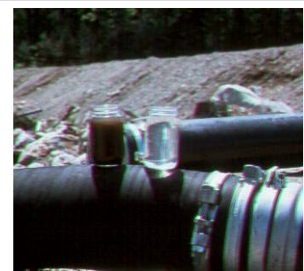
Comparison of influent (left) to effluent (right) from containment area
