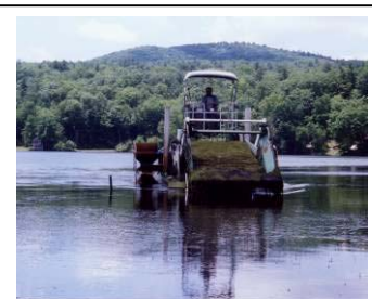
Using a harvester to transplant Chara to a site cleared of milfoil
