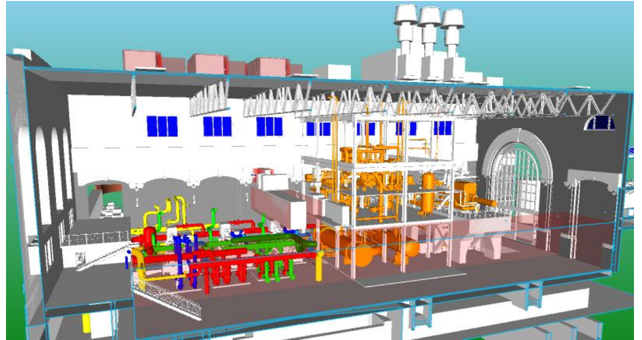
Design of Seawater Heat Pump
