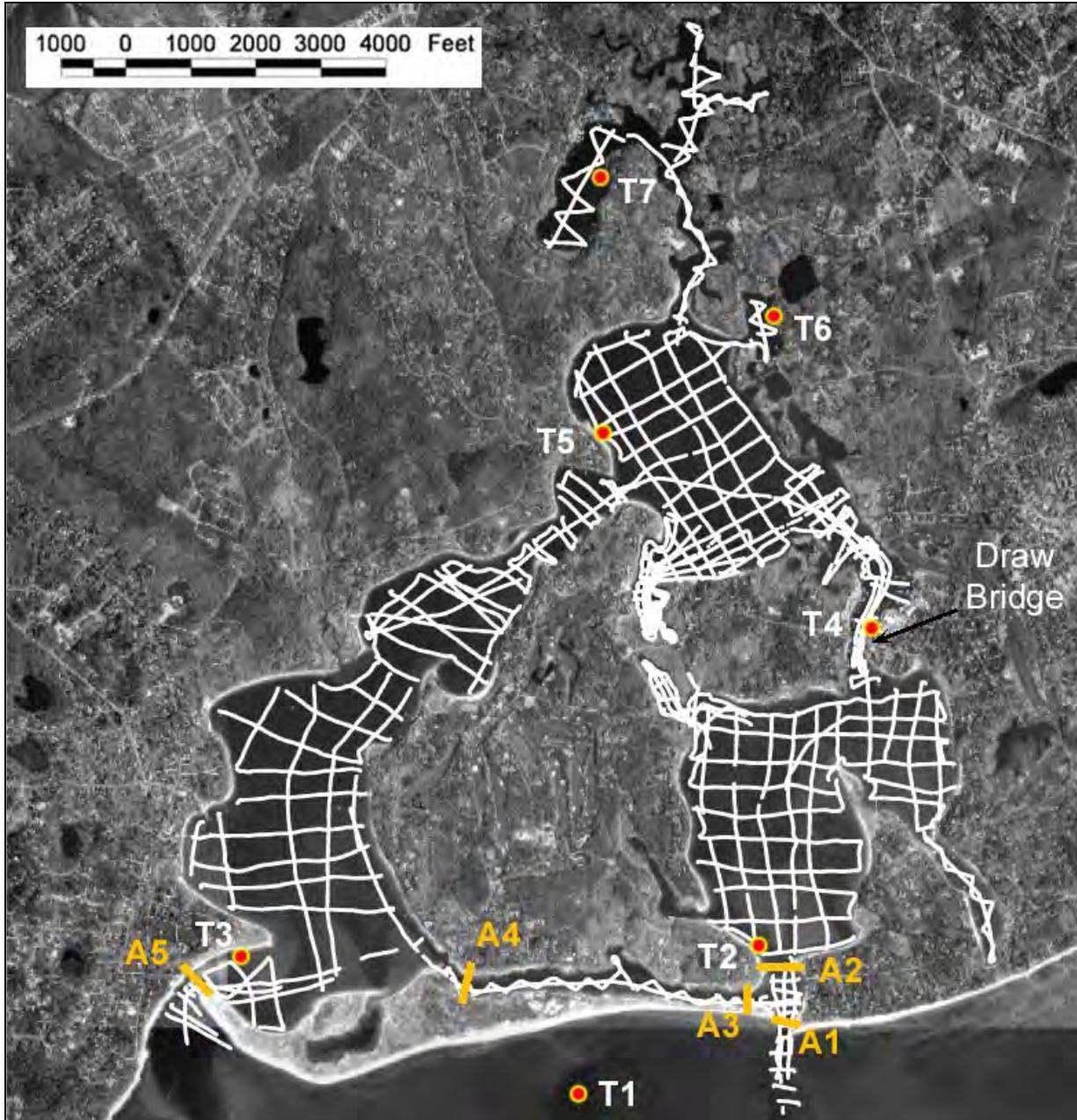
Figure V-8. Transects from the bathymetry survey of the Three Bays system. Yellow markers show the locations of the three tide recorders deployed for this study.
