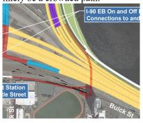
An inbound ramp in the Throat would improve this design and make the paths safer by eliminating the need for cyclists to make a u-turn at the bottom of the outbound ramp. Fitting this into the design for the Throat should be designed and considered.
