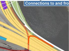
3. **Path widening near the River Street Bridge** Consistent with MassDOT Guidelines, a shared-use path should be at least 14' wide to accommodate substantial use by bicycles, joggers, skaters, and pedestrians, with a 2' shoulder on both sides. Creating separated paths for walking and biking is preferred.
