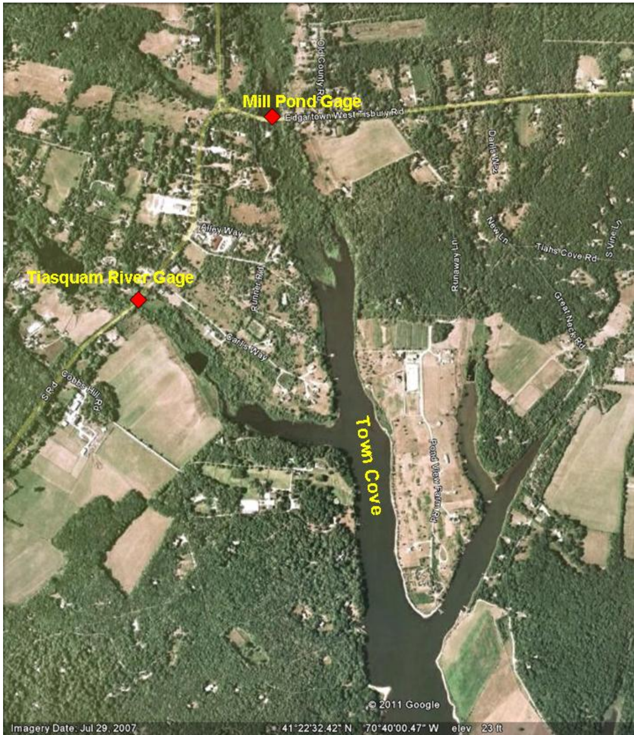
Figure IV-5. Location of Stream gauges (red diamonds) in the Tisbury Great Pond Embayment System watershed. The combined sub-watershed areas contributing to the gauge sites covers ~40% of the entire watershed to the estuary.
