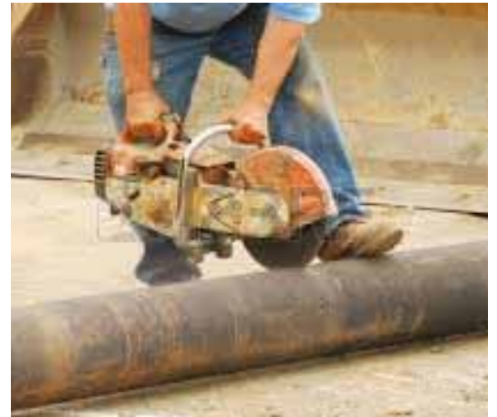
Circular blades can kick-back. Use the proper cutting area and make sure machine guards are in place.
