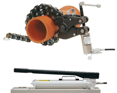
When possible, select tools that don't have potential for kick-back. This hydraulic cutter and diamond wire guillotine pipe cutter avoid kick-back forces.
