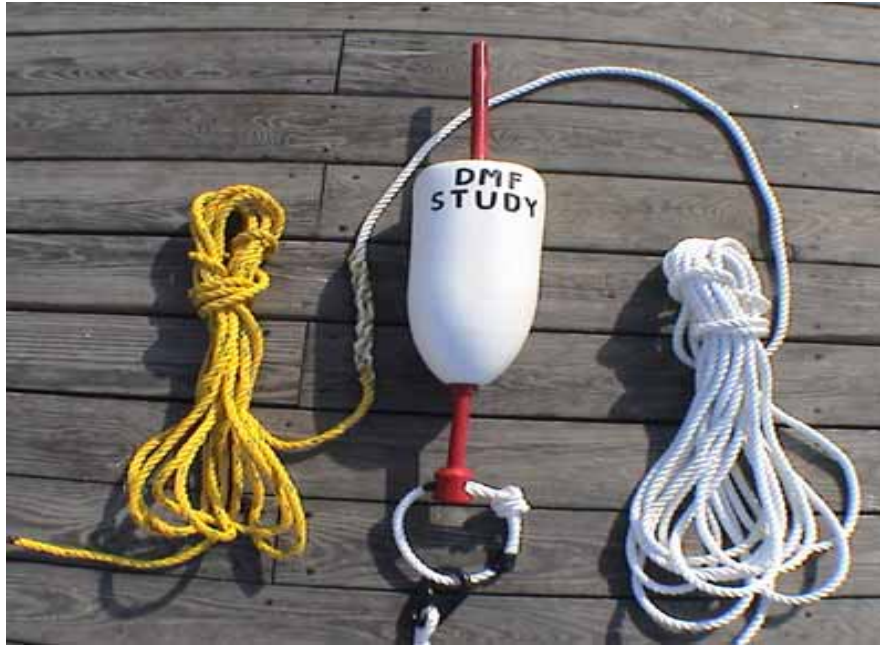
Image 1: 7/16" 3-strand buoyline configured with 33% float line at a 1.75 scope.
