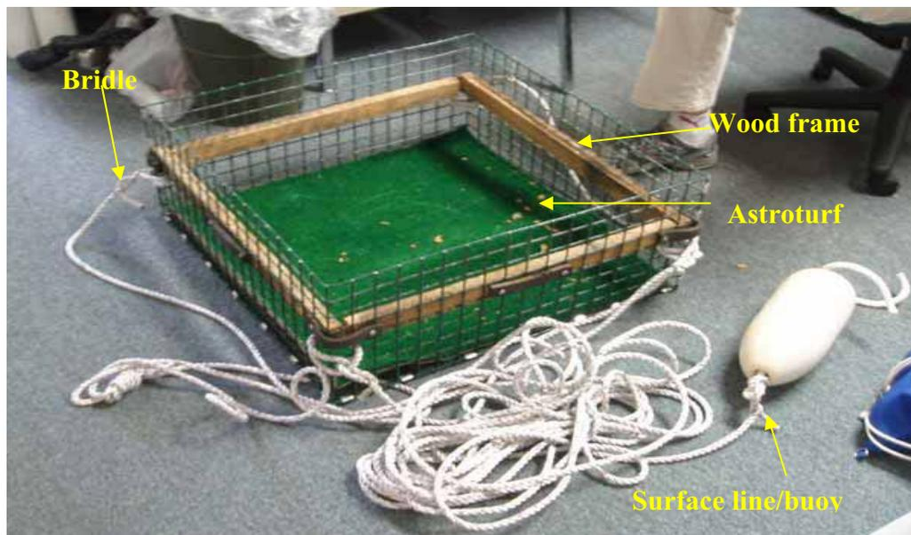
**Figure B5.** Settlement collector ready to be filled with cobble and deployed
