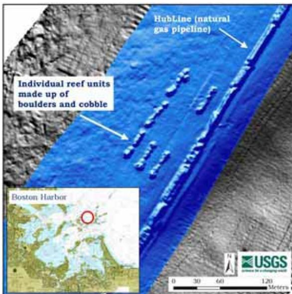
**Figure 2.4.** Results from the multibeam survey, conducted post-construction in July 2006, showing the location of the artificial reef units in relation to the HubLine cobble fill area.
