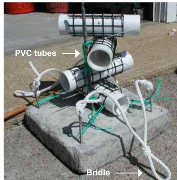
**Figure 1.4.** Current direction meter. Image shows position of stacked PVC tubes on a concrete base and bridles used for deployment and retrieval.
