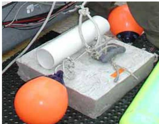
**Figure B8.** Permanent temperature monitoring station ready for deployment. Note: buoys and dive weight were only used for deployment.
