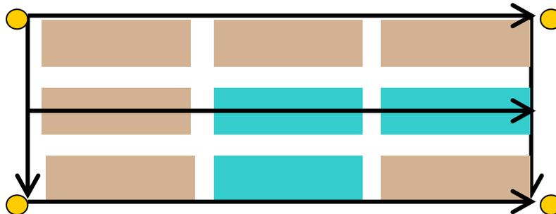
**Figure B2.** Example of the boat's movement over a potential site footprint while depth data were collected.
