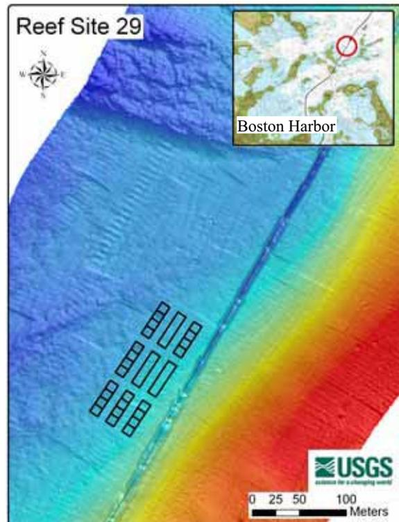
**Figure 2.2.** Multibeam and side-scan sonar survey results from a pre-construction survey in January 2006. Location of the planned reef area (Site 29) is shown over the sonar image; hashed areas depict areas where reef units were to be constructed, open bars depict sand sites.
