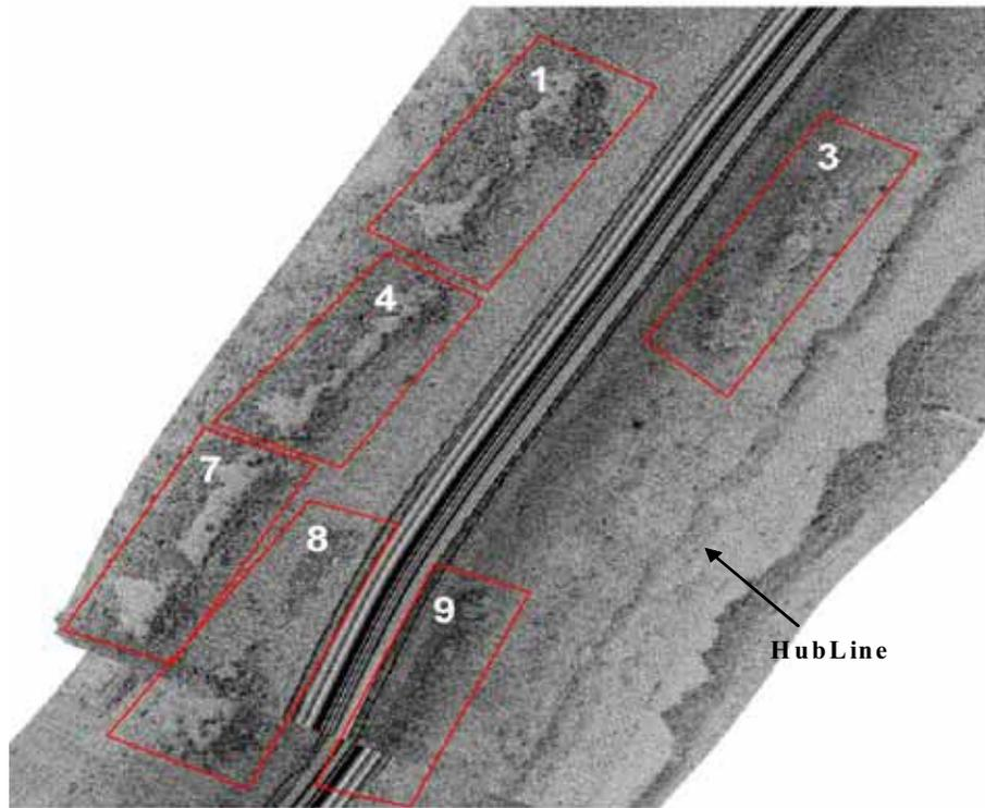
**Figure 2.3.** Side-scan sonar survey, conducted in May 2006, of the artificial reef units (outlined with their unique ID numbers) and the HubLine cobble fill point.
