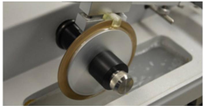
Figure 34. An embedded otolith being sectioned on the IsoMet low-speed saw.
