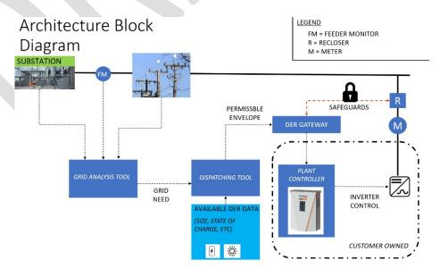
Flexible Connections requires integrating advanced enterprise software and interoperable hardware—including RTAC or DER gateways, local power controllers, and power plant communication protocols—to enable real-time monitoring, dynamic dispatch, and flexible DER connections, all underpinned by cybersecurity and standardized implementation frameworks.
