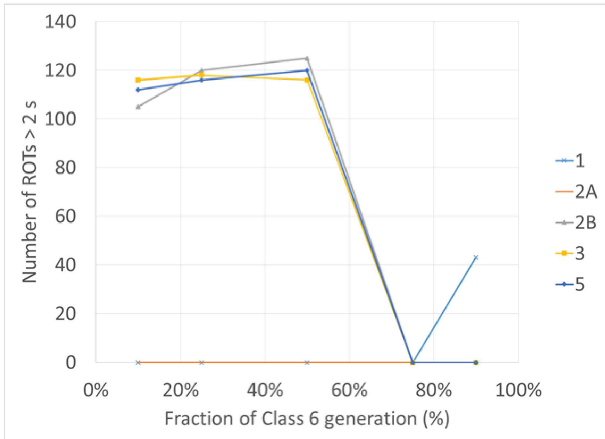
Figure 12. Plot of the number of ROTs greater than 2 s as the number of AI Group 6 inverters is varied, with RTs. The chart legend shows which type of inverter Group 6 is mixed with.
