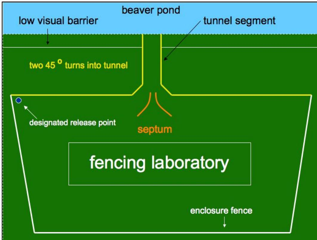
*Note: In this figure, the designated release point for test subjects is clearly labeled. Additionally, the laboratory is depicted with the 45° angled entrance and the septum in place.*
