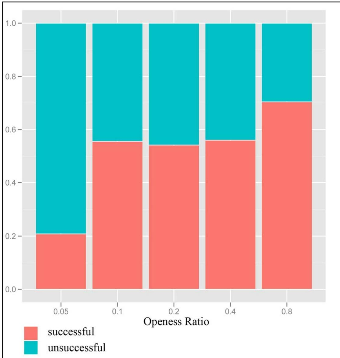
The bar graph in Figure 11 gives rates of passage success amongst painted turtles grouped by five levels of openness ratio (OR) in feet (0.05' n=24, 0.1' n=27, 0.2' n=25, 0.4' n=50, 0.8' n=27) encompassing all tested tunnel lengths and apertures. N is the number of turtles tested for each openness level. The y-axis ranges from 0 – 1 and depicts the fraction out of the total N for each OR tested that were either successful or unsuccessful trials.
