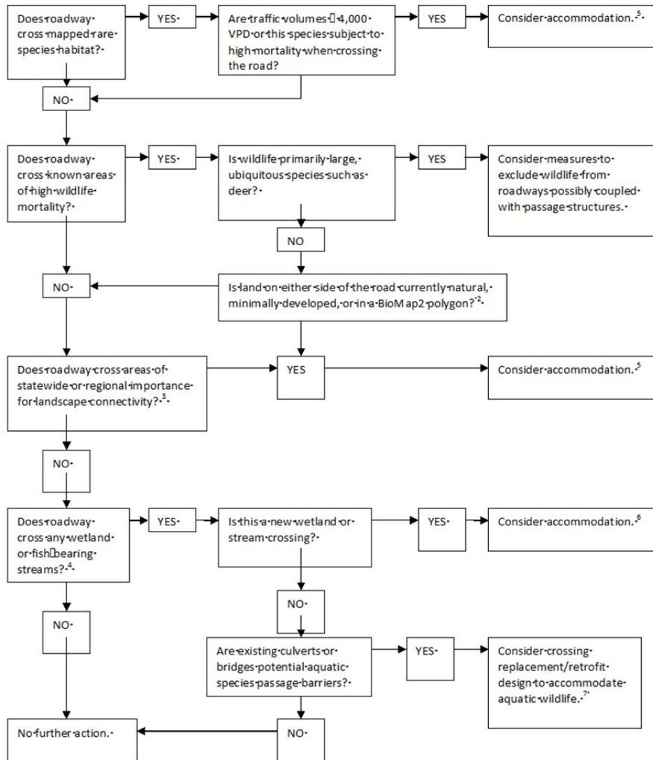
Figure 3.1: MassDOT Project Wildlife Accommodation Scenario for New and Replacement Stream Crossings
