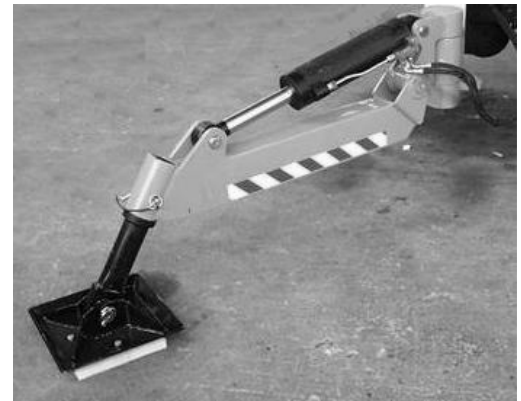
Fully deploy outriggers onto pads or solid surfaces
